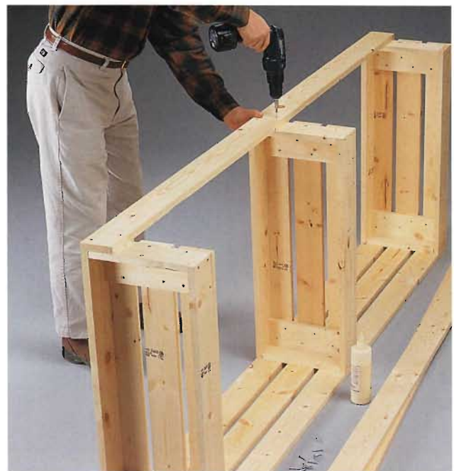
D. When attaching the side slats, position the outer side slats so the edge is flush with the edges of the fixed shelves.
