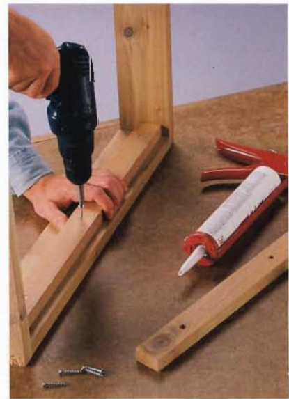
F. Add top supports in the lid frame to strengthen the top panel.
