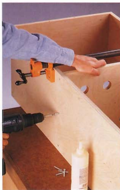
B. Glue and clamp the lower rack between the sides, then reinforce the joint with wood screws.
