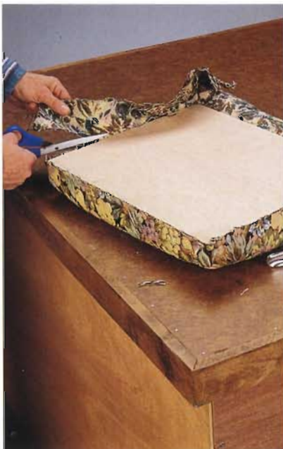
D. After stapling or tacking the upholstery material over the foam-rubber padding, trim off the excess material with scissors.
