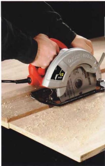
A. Cut the plywood pieces using a straightedge cutting guide.
