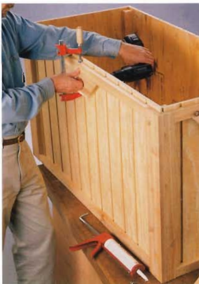
D. Attach a handle block to each face of the box, flush against the bottom of the top trim piece.
