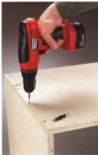
B. Screw the top and bottom to the sides, spacing the screws approximately every 5".
