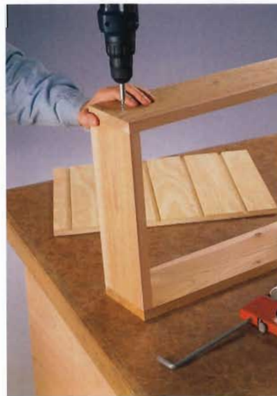
E. Counterbore the screw heads so they don't obstruct the movement of the tray on the tray slides.
