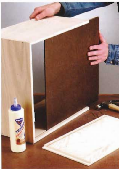
D. Assemble the drawers using glue and brads on the joints. Make sure the dados on the bottom line up properly.
