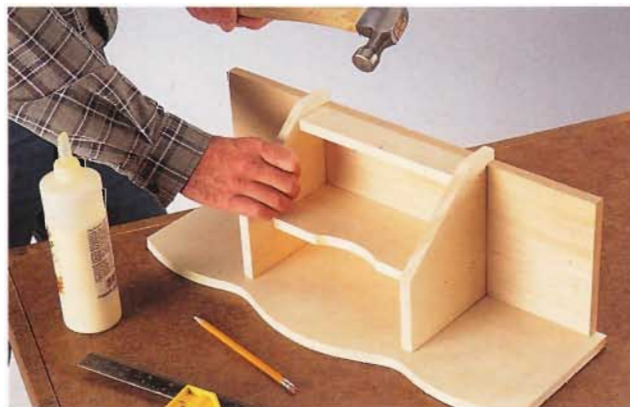
B. Assemble the frame, securing the pieces with glue and 1" brads.
