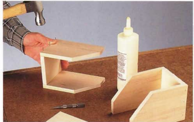
E. Fasten the drawer backs between the drawer sides with glue and wire brads.
