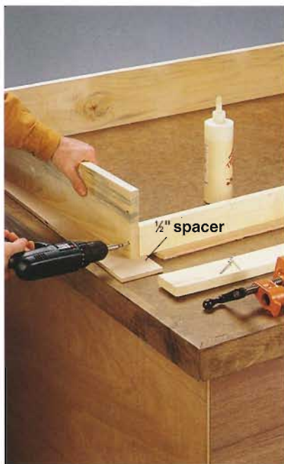
A. Fasten the back between the sides with wood glue and counterbored screws. Keep the bottom flush with spacers.
