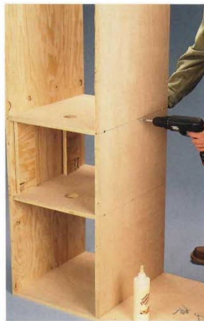
C. Use wood spacers to support each shelf while you fasten it with screws.
