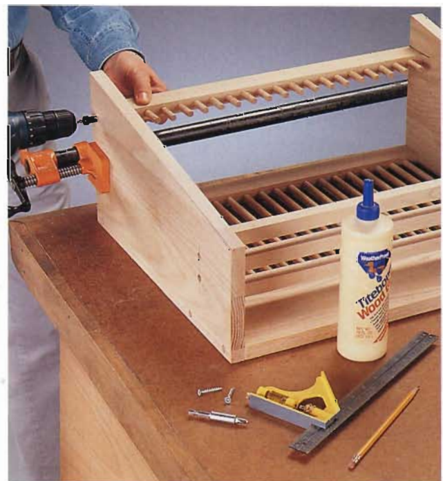
D. Clamp the front rail, drill pilot holes, and then glue and screw the rail into place.
