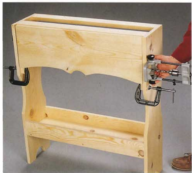
E. Clamp the bin to the framework. Then, drill dowel holes through the sides and into the bin.
