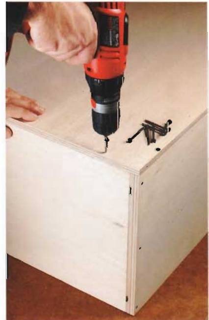
C. Assemble the cabinet sides, top, and bottom, then add the plywood back.
