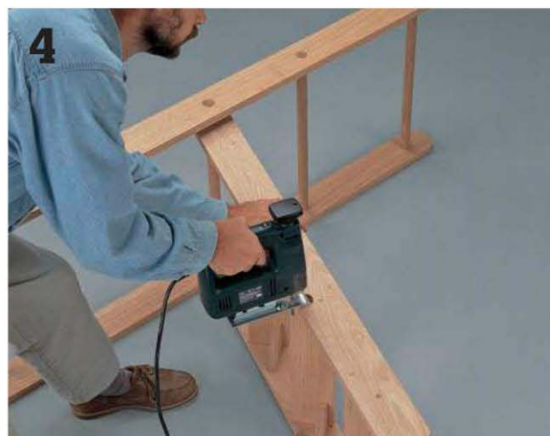
Cut U-shaped notches in the back edges of the step rails so they will lock over the bottom dowel rung.
