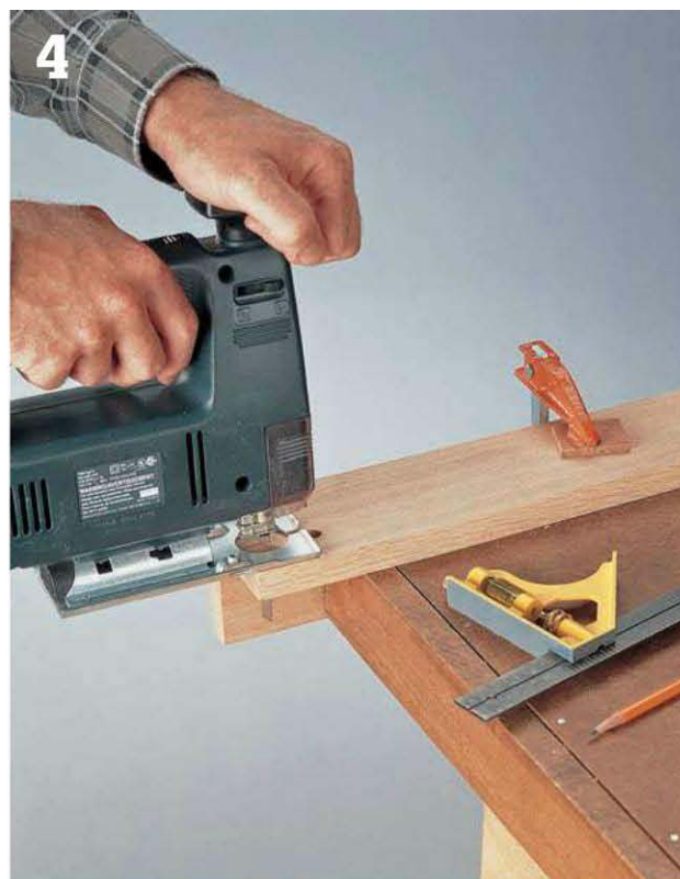
Cut a notch from the top of the leg fronts down to the carriage bolt hole to make it easier to remove and install legs.
