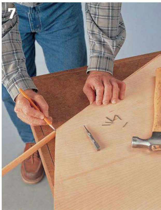
Mark the trim pieces to fit the edges of the poker table, and cut them to length with a 22\frac{1}{2}^\circ bevel.
