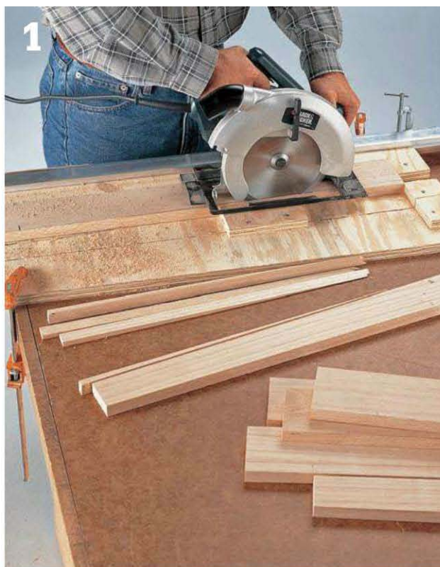
Use a straightedge guide and scrap-plywood stop blocks when cutting leg tapers with a circular saw.
