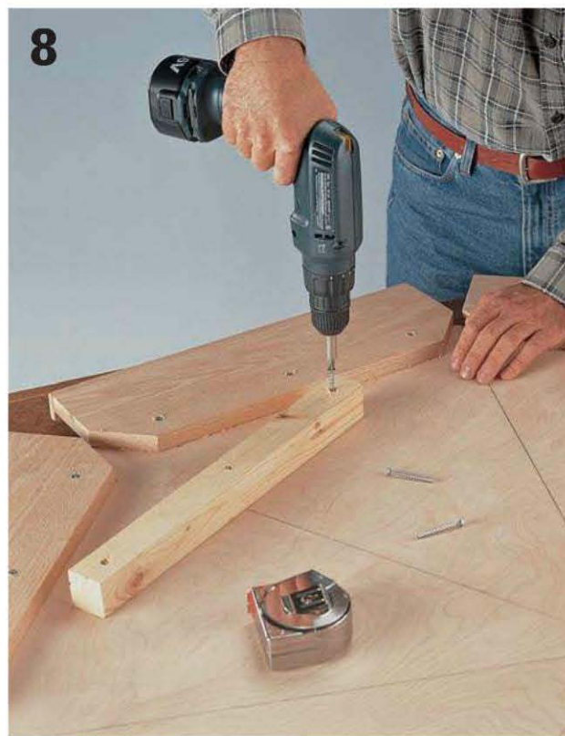
Fasten the poker cleats to the underside of the poker table, 16\frac{1}{8} " from the center of the table.
