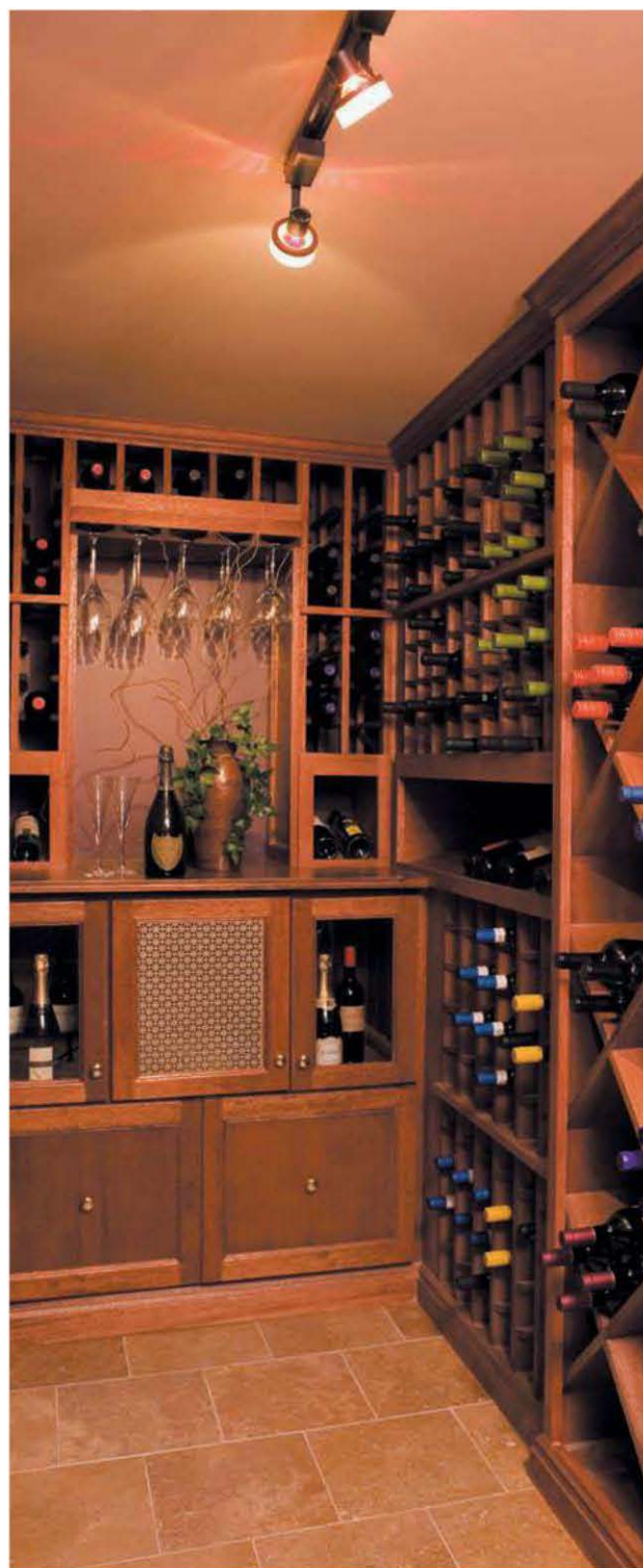
Typical wood wine racks are constructed from moisture-resistant wood, such as redwood, western red cedar, or mahogany.
