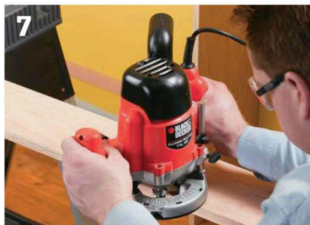
Routing a bead, roundover, or chamfer adds nice detail and shadow lines to the upright backers.
