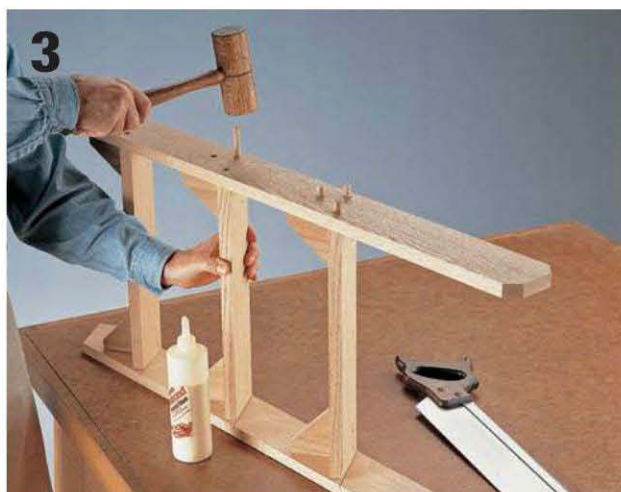
Drive three glued, 2"-long dowels into each step tread joint after the glue in the joints has set.
