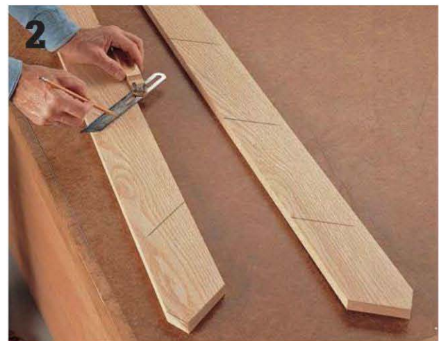
2 Draw reference lines for positioning the treads parallel to the bottoms of the step rails.
