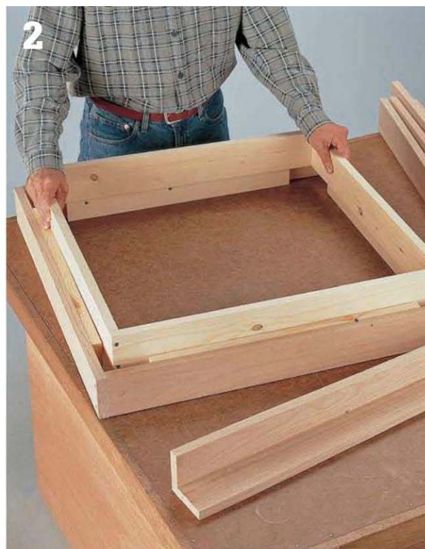
Position the liner assembly inside the apron assembly so it fits against filler blocks.
