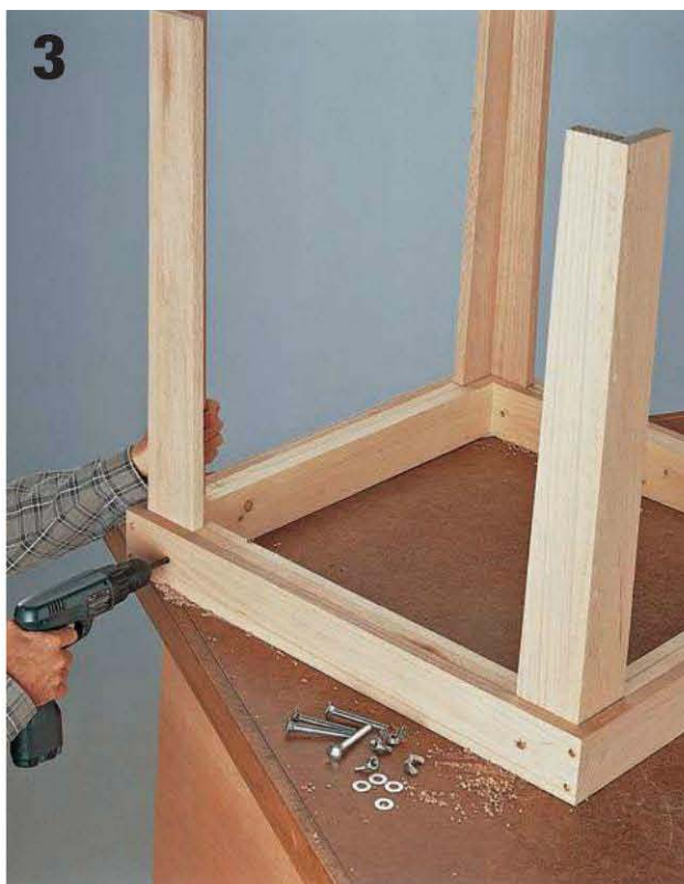
Hold the legs firmly , and drill ⅜"-diameter holes through the apron, legs, and liner for carriage bolts at all corners.
