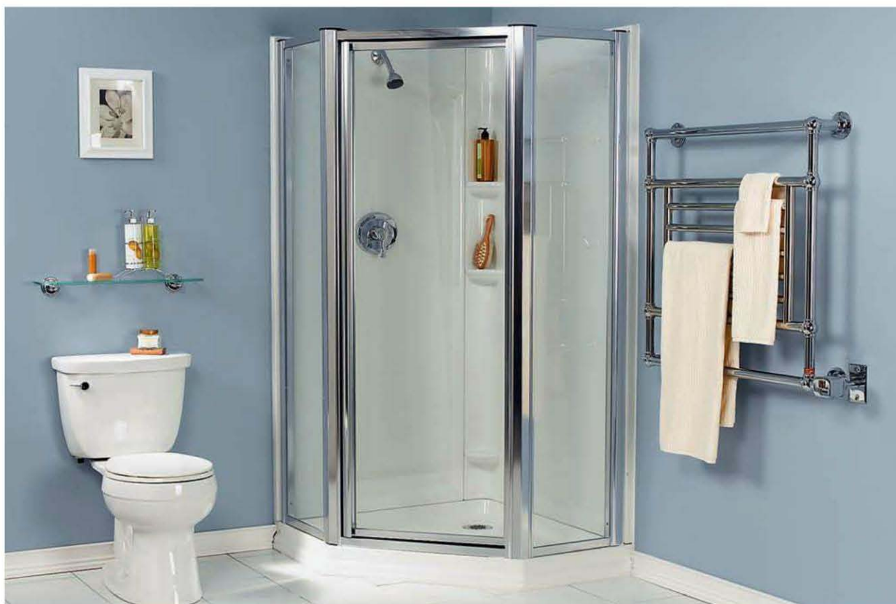
A hard-wired towel warmer offers the luxury of heated towels without the safety concerns of a plug-in device.
