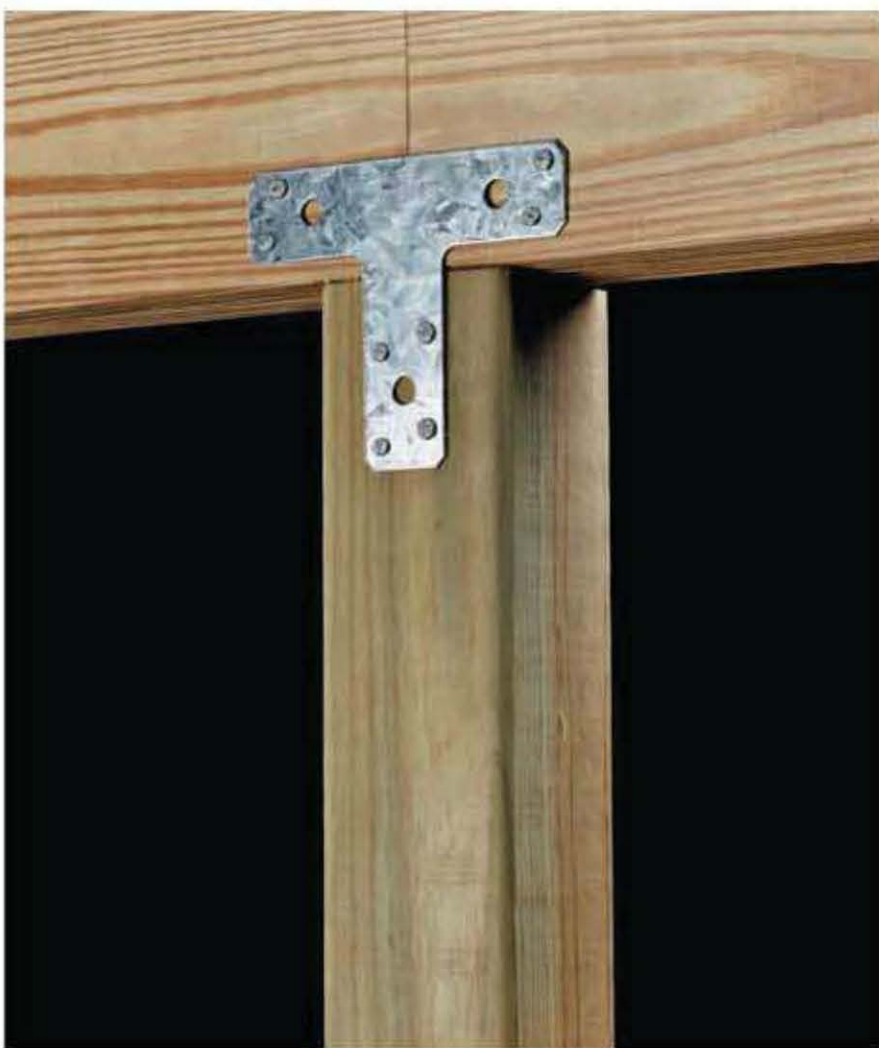
T-straps reinforce the connection between beam and post, particularly on long beams requiring spliced construction. Local building codes may also allow their use in place of post caps.
