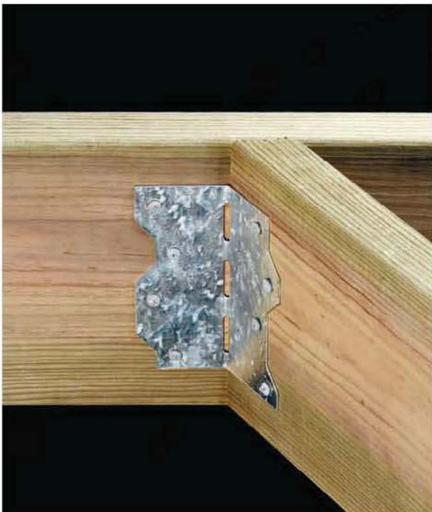
Skewable angle brackets reinforce framing connections at angles other than 90 degrees or at beam ends where 45-degree joist hangers won't fit.
