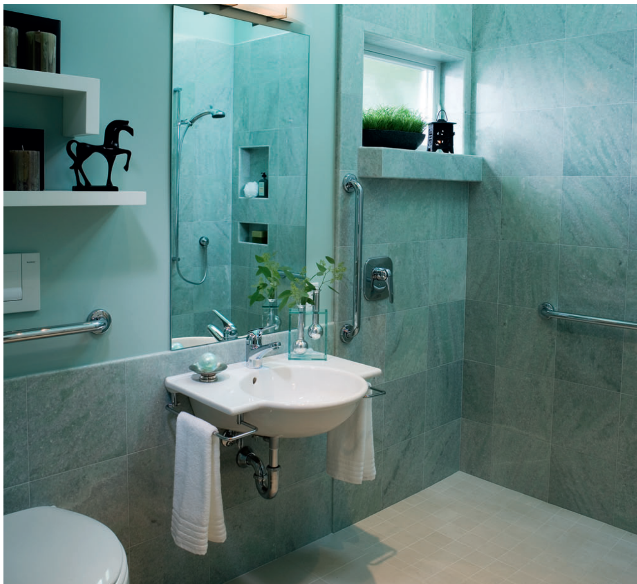
Roll-in shower designs, roll-under sinks, grab bars, adjustable slide-bar showers, and open floor space make bathing easier for people with disabilities.
