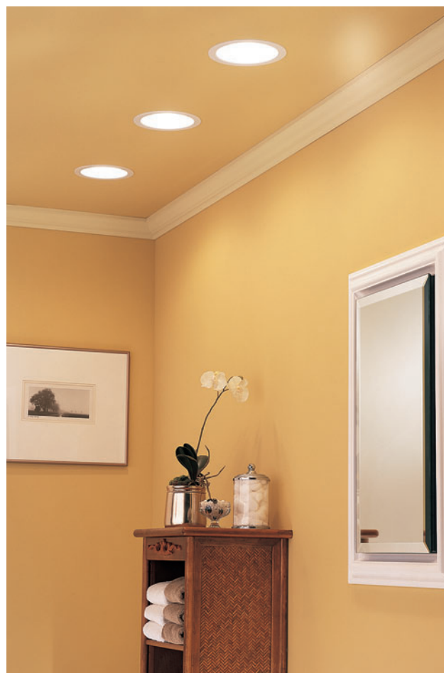
Recessed light fixtures provide nondirectional lighting and have a fairly neutral design impact.
