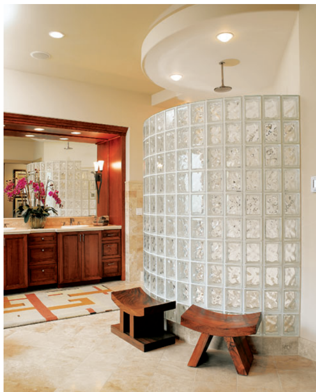
Glass block allows light to penetrate the wall while serving as a partition.
