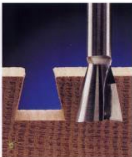
A dovetail bit cuts wedge-shaped grooves used to make interlocking joints for furniture construction and cabinetwork.
