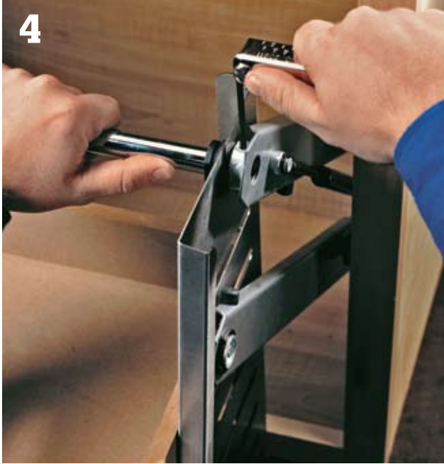
Position the box unit in front of the cabinet, rotate the lower arms downward, and secure them to the side pieces using the bolts, washers, and nuts provided. Insert the top handle. Lower the upper arms one at a time, and insert the handle end into the arm. Secure the handle with the two setscrews in each arm using an Allen wrench.
