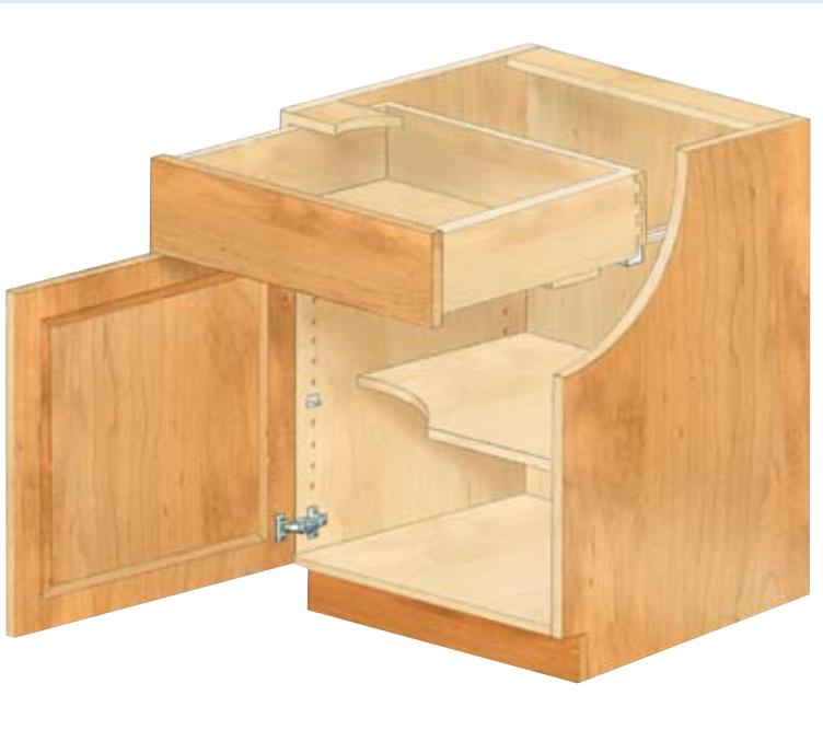
Frameless cabinets , sometimes called “European-style,” are more contemporary. Because they have no face frames, frameless cabinets offer slightly more storage space than framed cabinets. The doors and drawers on frameless cabinets cover the entire unit.
