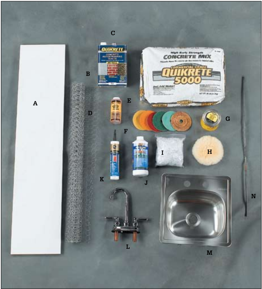
The basic supplies needed to build your countertop form and cast the countertop include: (A) Melamine-coated particleboard for constructing the form; (B) poultry netting or welded wire for reinforcement; (C) concrete sealer (product shown is adequate, but for better protection look for a sealer that has both penetrating and film-forming properties); (D) high/early bagged concrete mix rated for 5,000 p.s.i.; (E) coloring agent (liquid or powder); (F) grinding pads (shown are 5" diamond pads ranging from 50 grit to 1,500 grit for grinding and polishing); (G) paste wax; (H) buffing bonnet for polisher; (I) fiber reinforcement (nylon); (J) acrylic fortifier, latex bonding agent (or water reducing admixture if you can locate it); (K) black or colored silicone caulk; (L) faucet set if installing sink; (M) sink (self rimming shown); (N) No. 3 rebar (¾").
