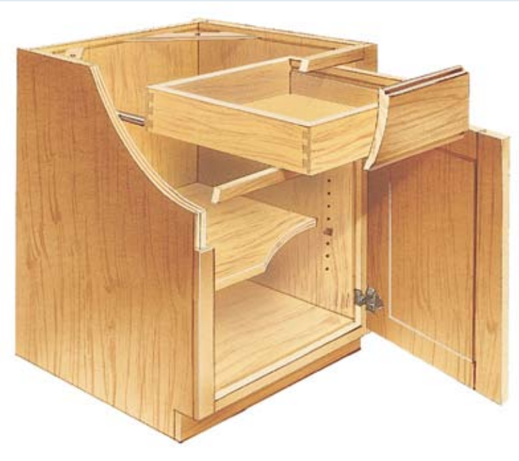
Face-frame cabinets have openings that are completely surrounded by face frames made of vertical stiles and horizontal rails. They give kitchens a traditional look.
