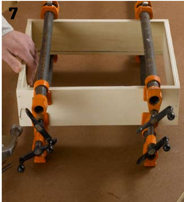
Build or purchase drawers. Simple overlay drawers are easy to make from ½" plywood and a false front made of hardwood. Refer to the information on page 81 for construction details and guidance on sizing drawers.
