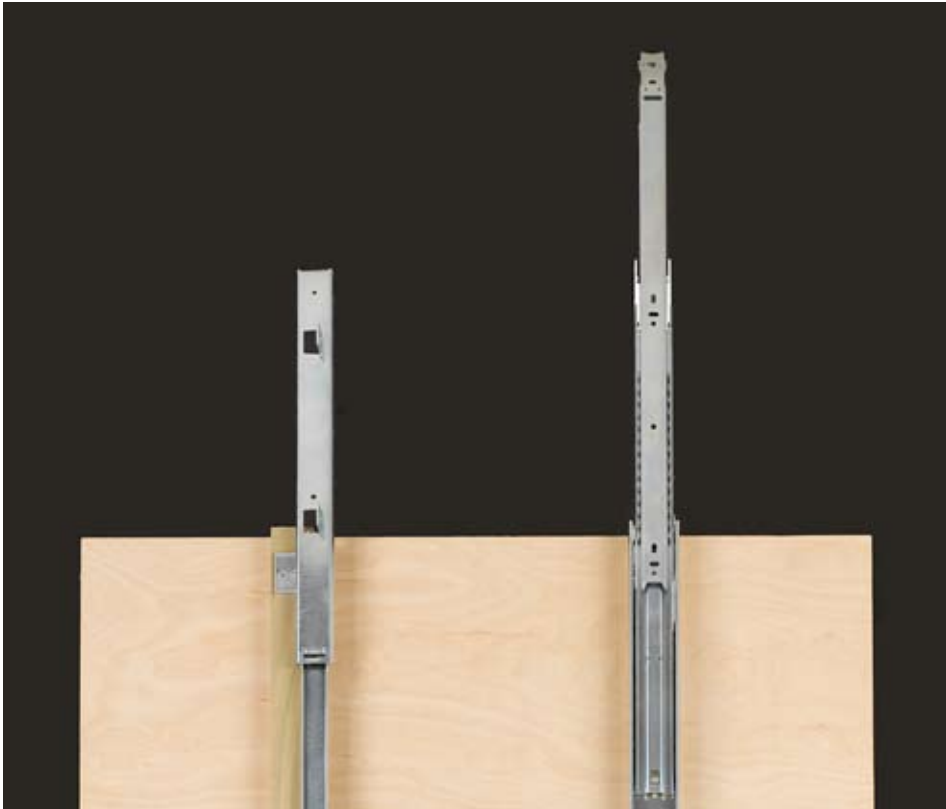
Drawer slides suitable for pullout shelves are commonly available in both standard (left) and full extension (right) styles. Standard slides are less expensive and good enough for most applications. They allow the tray to be pulled out most of the way. Full extension slides are a little pricier than standard slides but they allow the tray to be pulled completely out of the cabinet box for easy access to items in the back.
