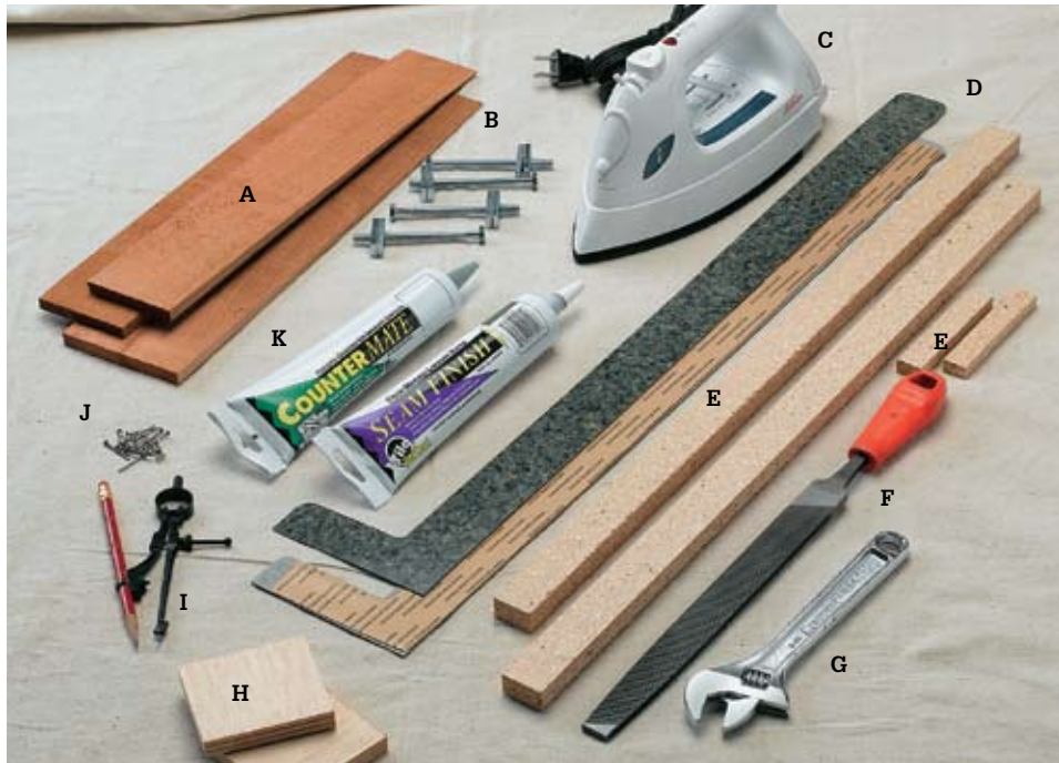
The following tools and materials will be used in this project: wood for shimming (A); take-up bolts for drawing miters together (B); household iron (C); endcap laminate to match countertop (D); endcap batten (E); file (F); adjustable wrench (G); buildup blocks (H); compass (I); fasteners (J); silicone caulk and sealer (K).
