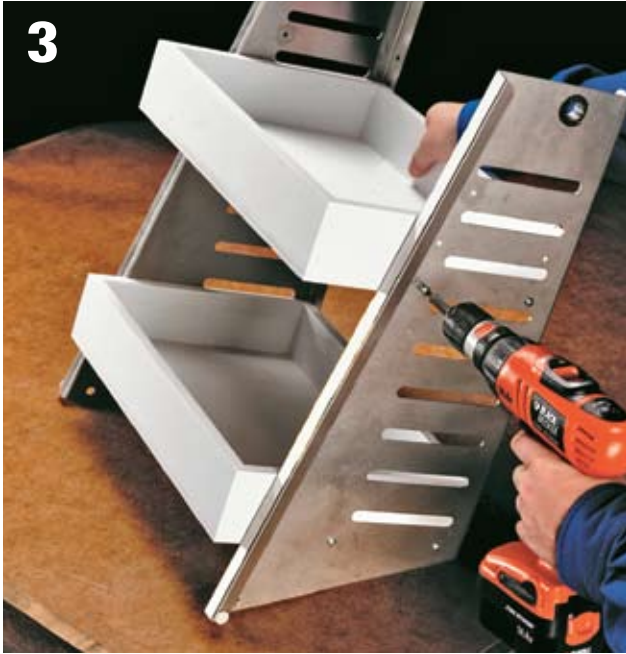
Build two shelf boxes from ½" MDF. Paint and install the boxes between the sides of the shelf unit using the predrilled holes in the side pieces. Secure the boxes with #8 panhead screws. Because the lower box can be installed in only one position, install it first. Then, find the desired position for the upper box, and secure it in place. Slide the lower handle through the holes in the side pieces.
