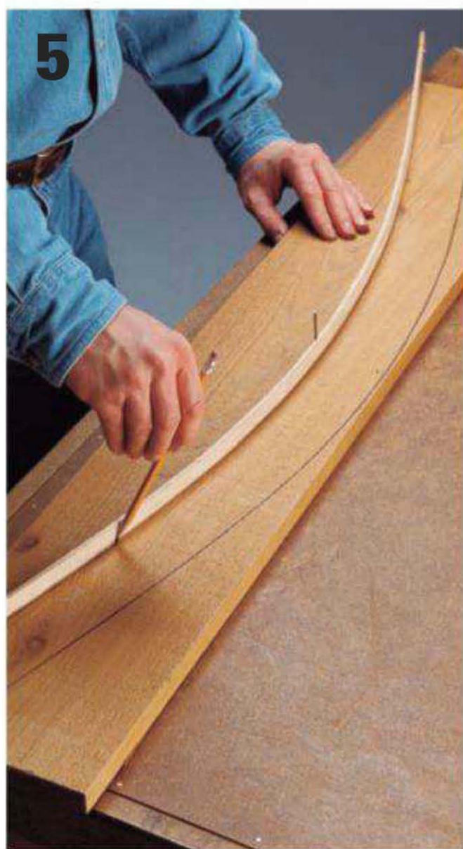
Lay out the handrails. Use a flexible piece of plastic or wood as a marking guide when drawing the cutting lines for the center handrails.
