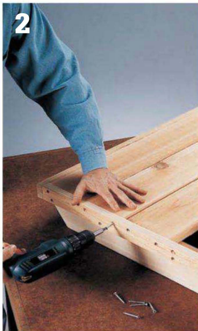
Install the tabletop slats by driving screws through the tabletop frame and into the ends of the slats.
