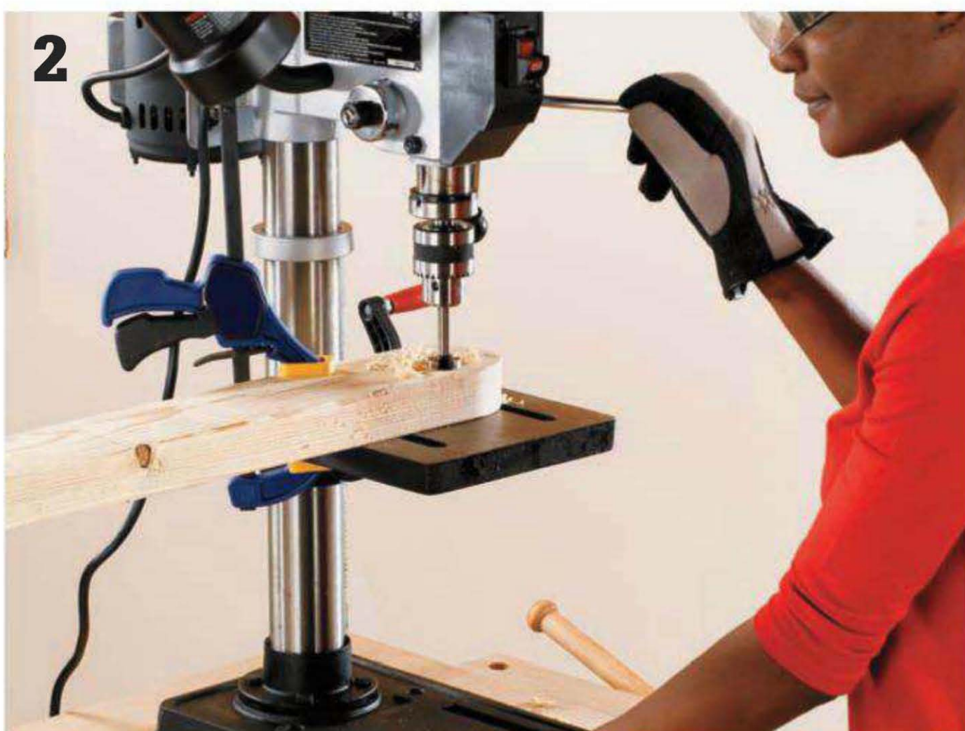
Cut the round handle mortises. Use a Forstner bit to bore the handle mortises. Forstner bits feature flat sharp edges on the bottom that cut a flat bottom hole. They are designed for use with drill presses, not portable drills. If you don't have a drill press use a 1" spade bit and a portable drill.
