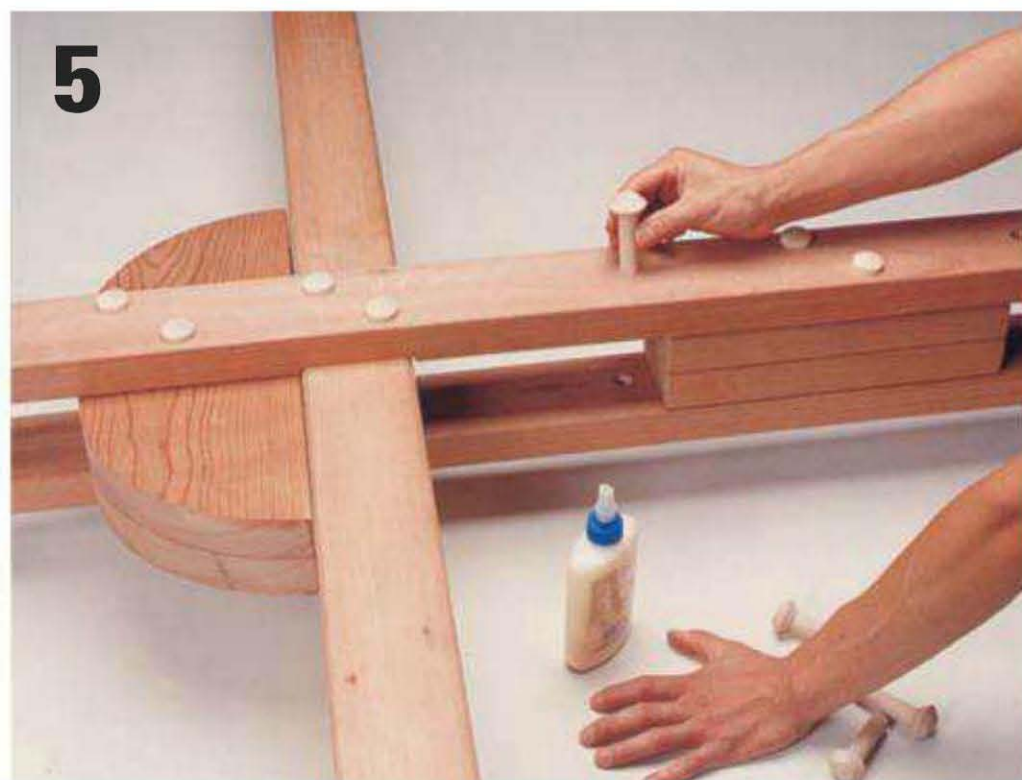
Insert a Shaker peg into each guide hole so the cap extends 1" out from the rail. Glue in place and trim the end flush.
