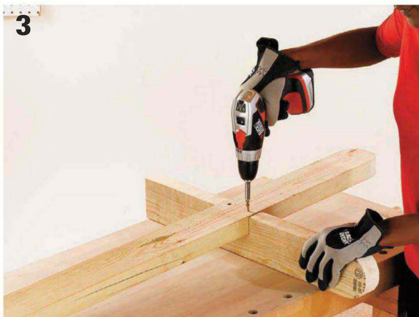
Assemble the base frame parts. Fit the leg notches over the base rails and attach the legs with 2½" screws.
