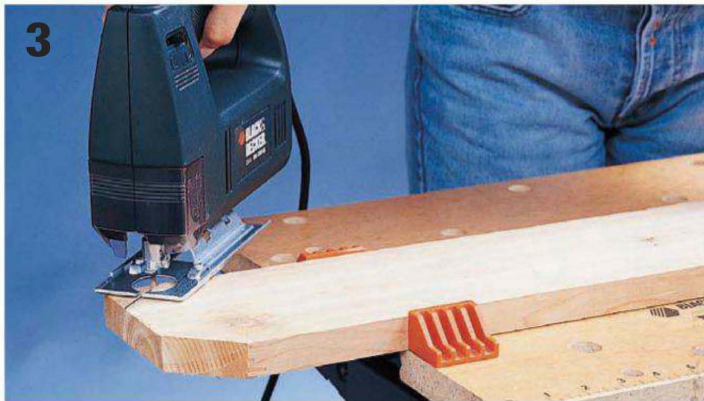
Make corner cuts on the fronts of the arms (shown) and the tops of the back slats using a jigsaw.
