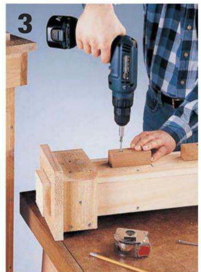
Attach the short post cleats 3\frac{5}{8} " up from the tops of the long post cleats. The top stringers on the panels fit between the cleats when installed.
