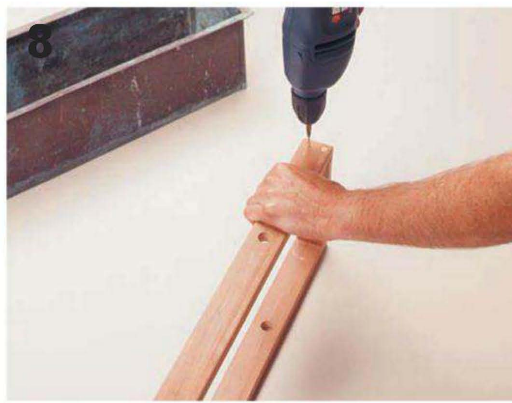
Fasten the planter hanging frame with a pair of #6 wood screws driven in pilot holes at each corner.
