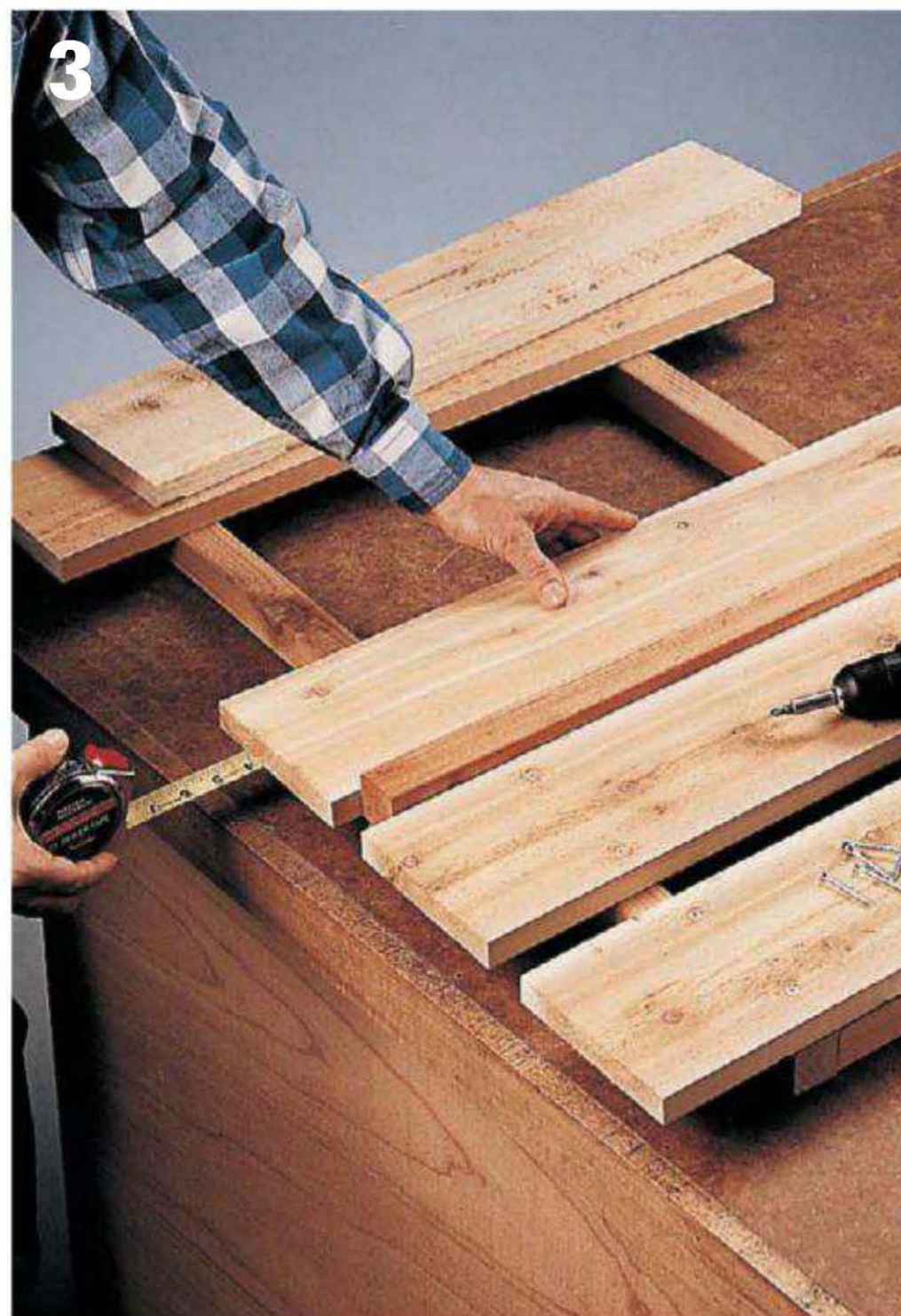
Continue to attach slats. The inner slats should be 1\frac{1}{2} " apart, with the ends 4" below the bottom of the frame.
