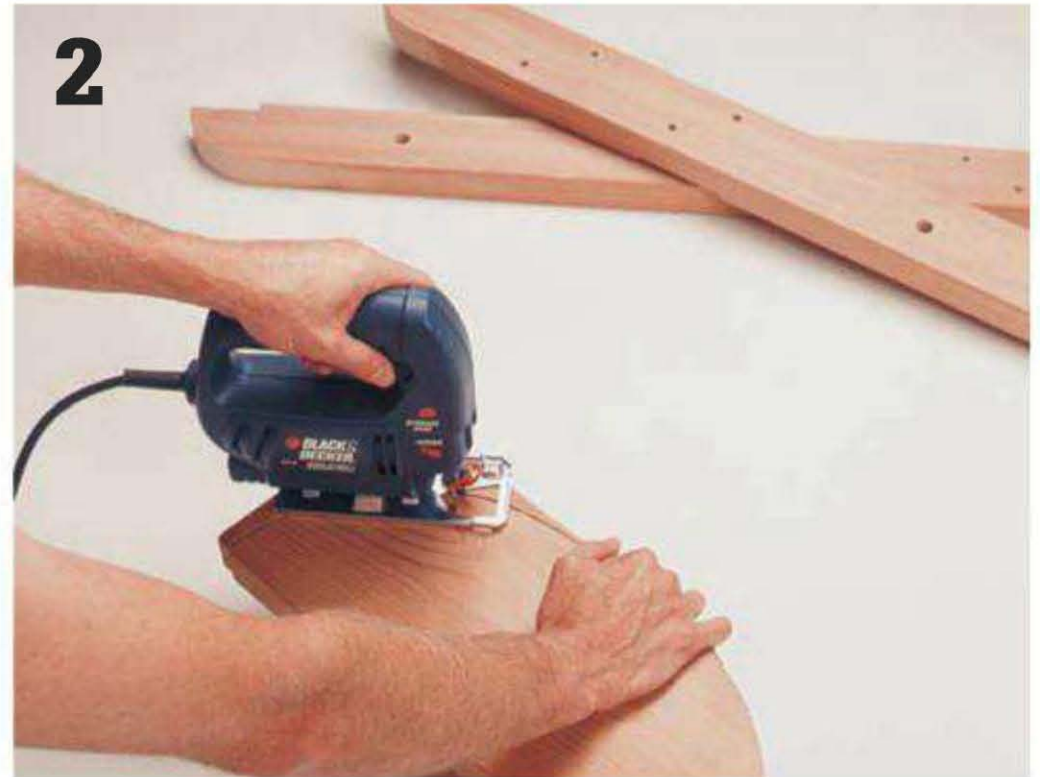
Cut and shape two braces. Draw an arc with a 5½" radius on the braces and cut with a jigsaw.
