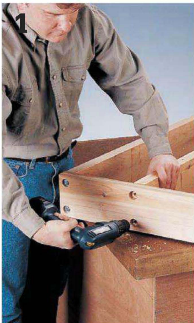
1 Drill pilot holes through \frac{3}{4} "-dia. counterbores when preparing to drive the lag screws into the ends of the bottom rails.
