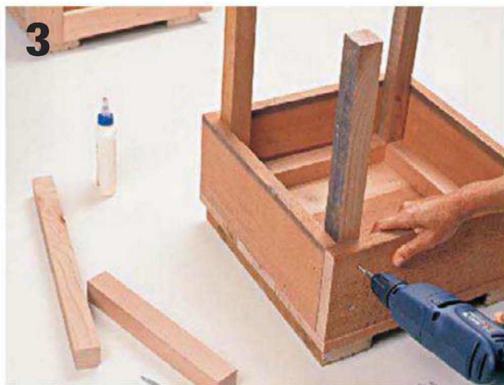
Attach the side strips to the corner braces with 2" deck screws to create the boxes.
