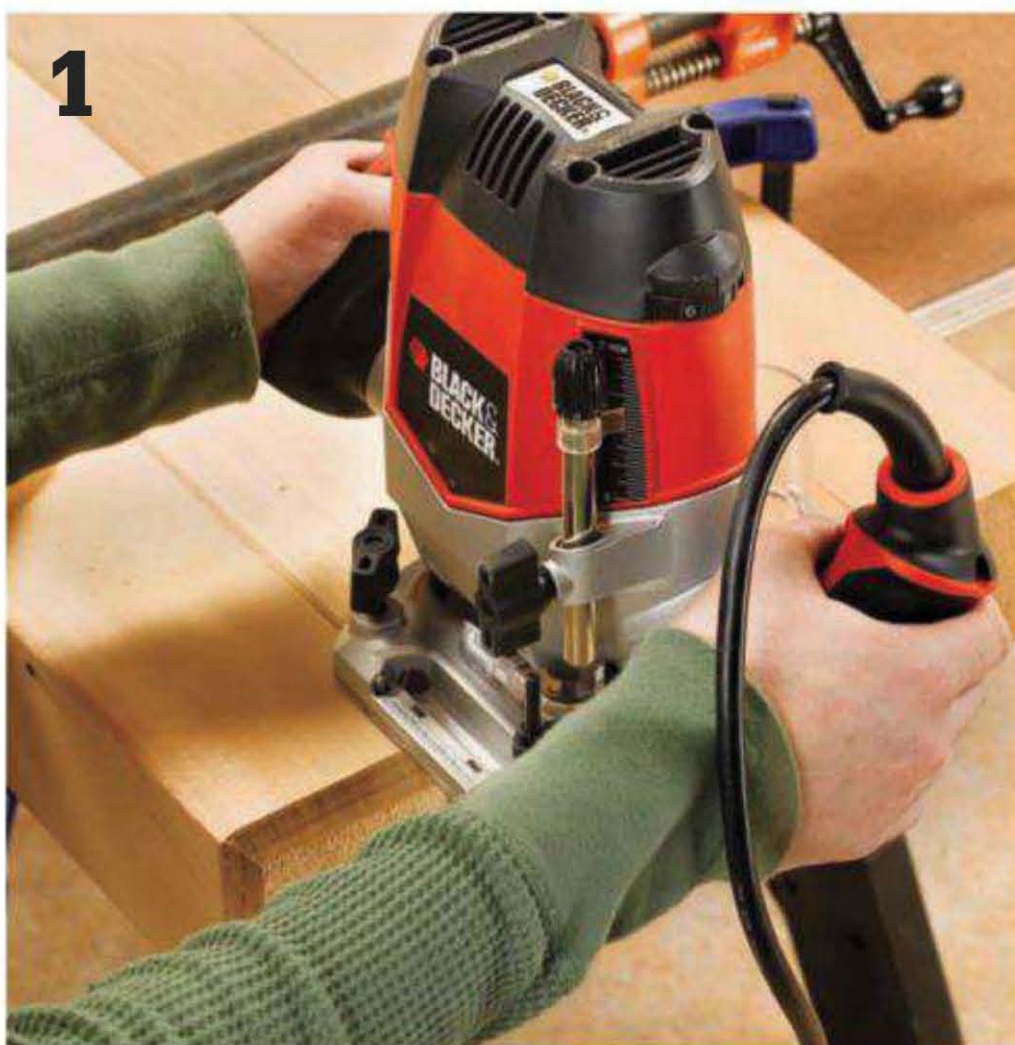
Make the posts. After cutting them to length from 4 × 4 cedar, make a 1/4" chamfer cut around all the tops. Gang the posts together for profiling if you like.
