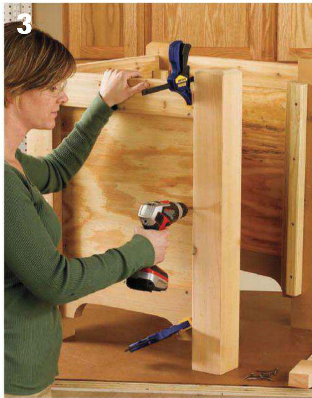
Attach the side assemblies. First, drive 3" deck screws through the corner nailers and into the rails. Then, drive 1¼" deck screws through the side panels and into the nailers. Reinforce the joints with adhesive.
