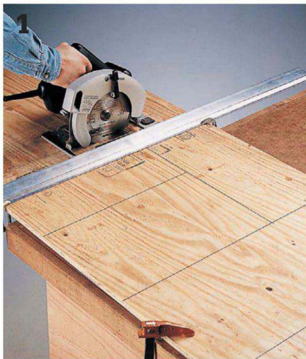
Cut the end panels and side panels to size from cedar siding using a circular saw and a straightedge cutting guide.
