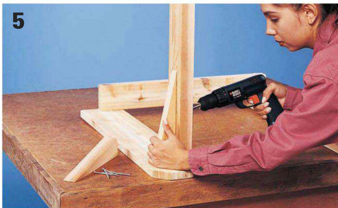
Drive screws through each post and into an arm brace to stabilize the arm/post joint.
