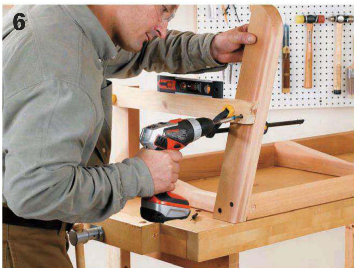
Attach the arm supports. Drive two 2½" deck screws through each end of the arm supports and into the front and back posts. Then attach the arm front with two 2½" deck screws.
