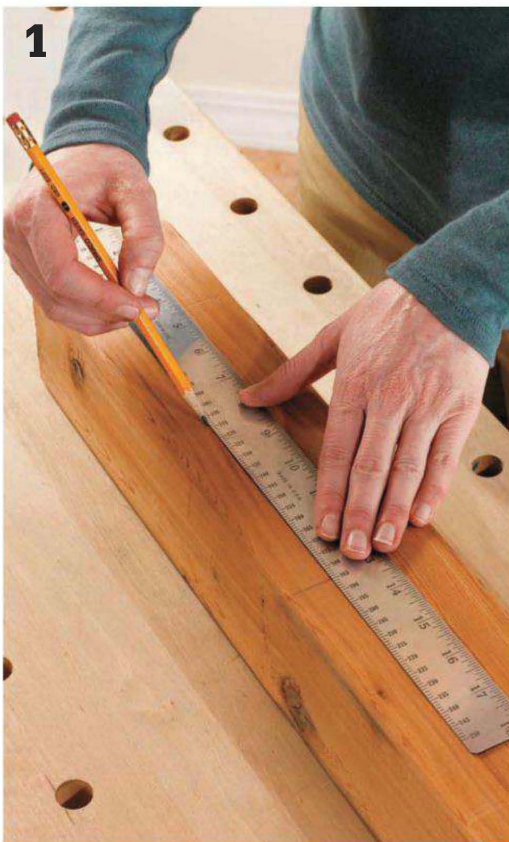
Mark the post bevel cuts. The lines at the top of each back post should be drawn 1" out from the corner and should run down the post for 12" long.
