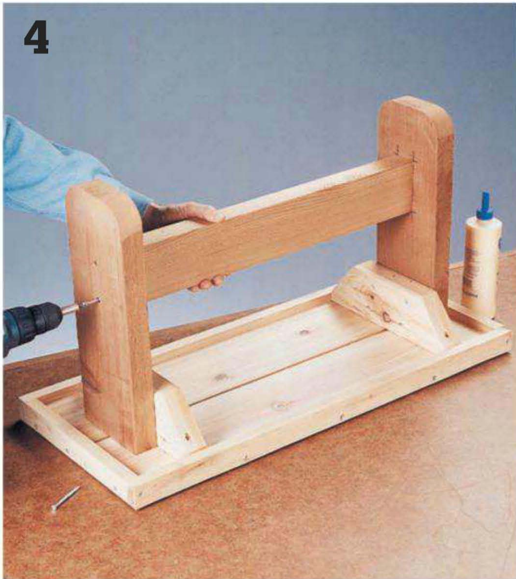
4 Attach the bench legs to the outer faces of the stringers and then attach a stretcher between each leg pair.
