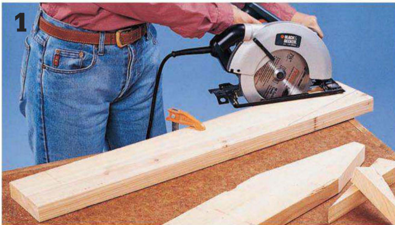
Cut tapers into the back edges of the legs with a circular saw or jigsaw.
