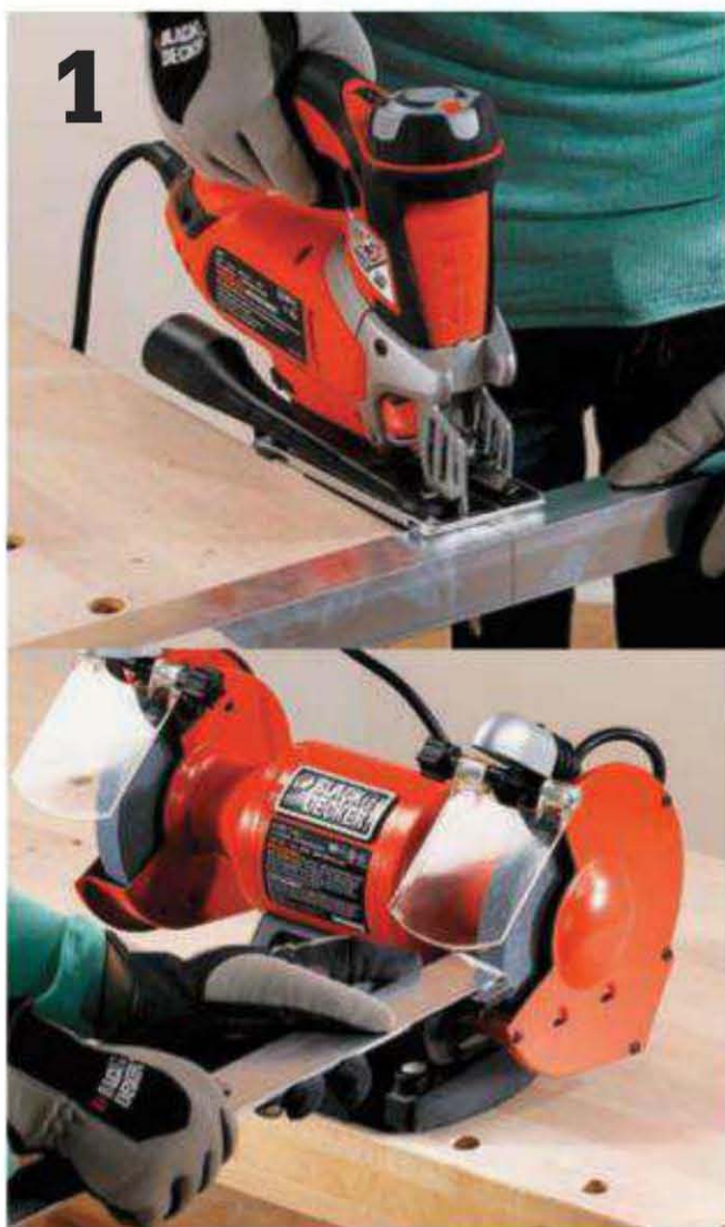
Cut the aluminum angle for the frame parts (top) and then deburr the cut ends on a bench grinder (lower). Don't overdo it on the grinder.
