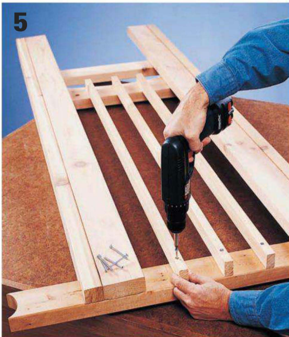
Attach trellis strips to the crossbrace and spreader with deck screws.
