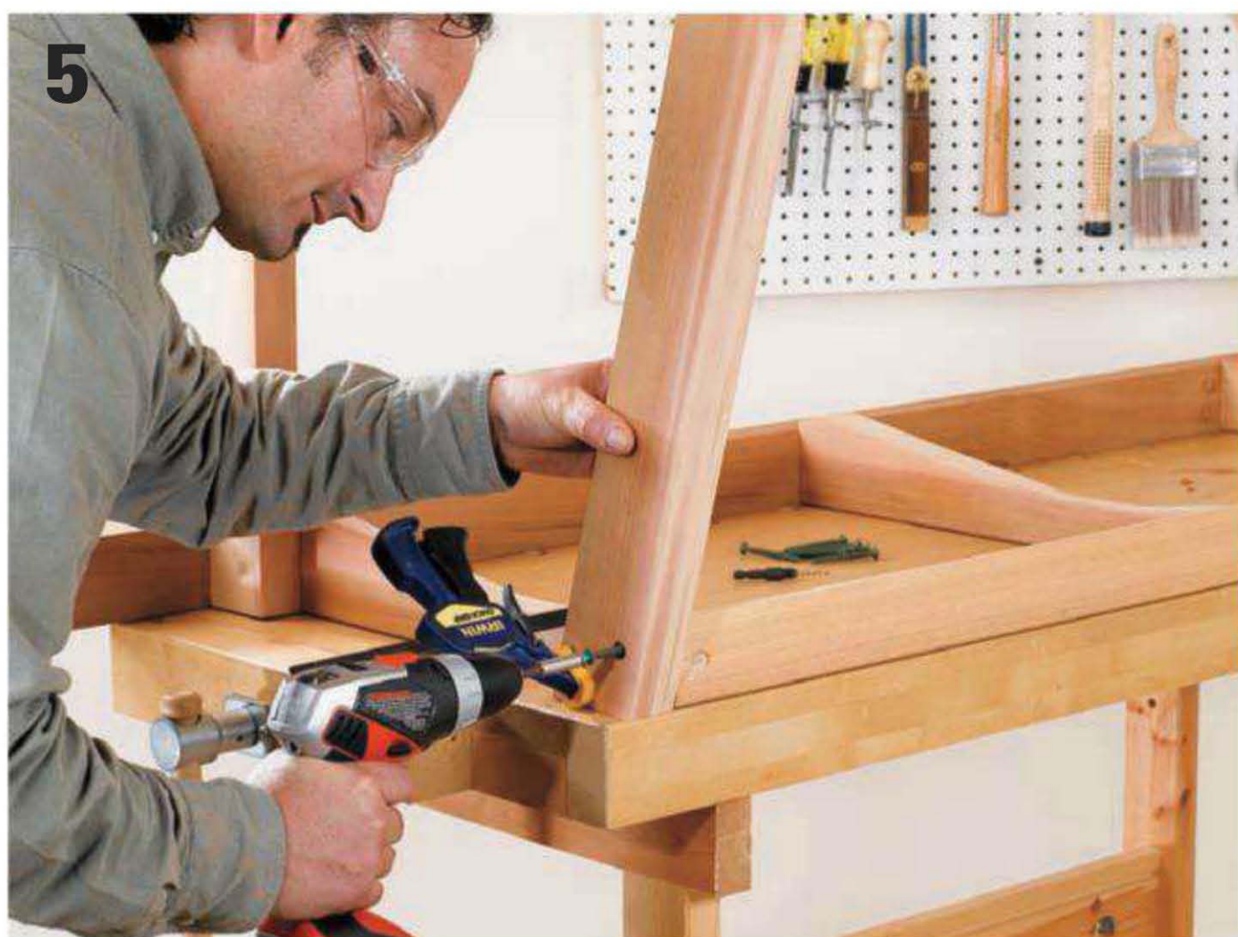
Attach the back posts. Drive two 2½" deck screws through each back post and into the outside seat supports.
