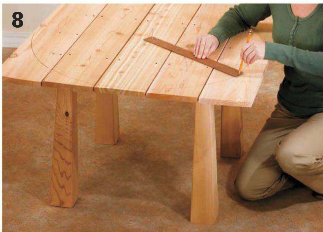
Lay out the circular cutting line. Draw the perimeter of the tabletop using an 18¾" long compass. You can also use a piece of string as a compass.
