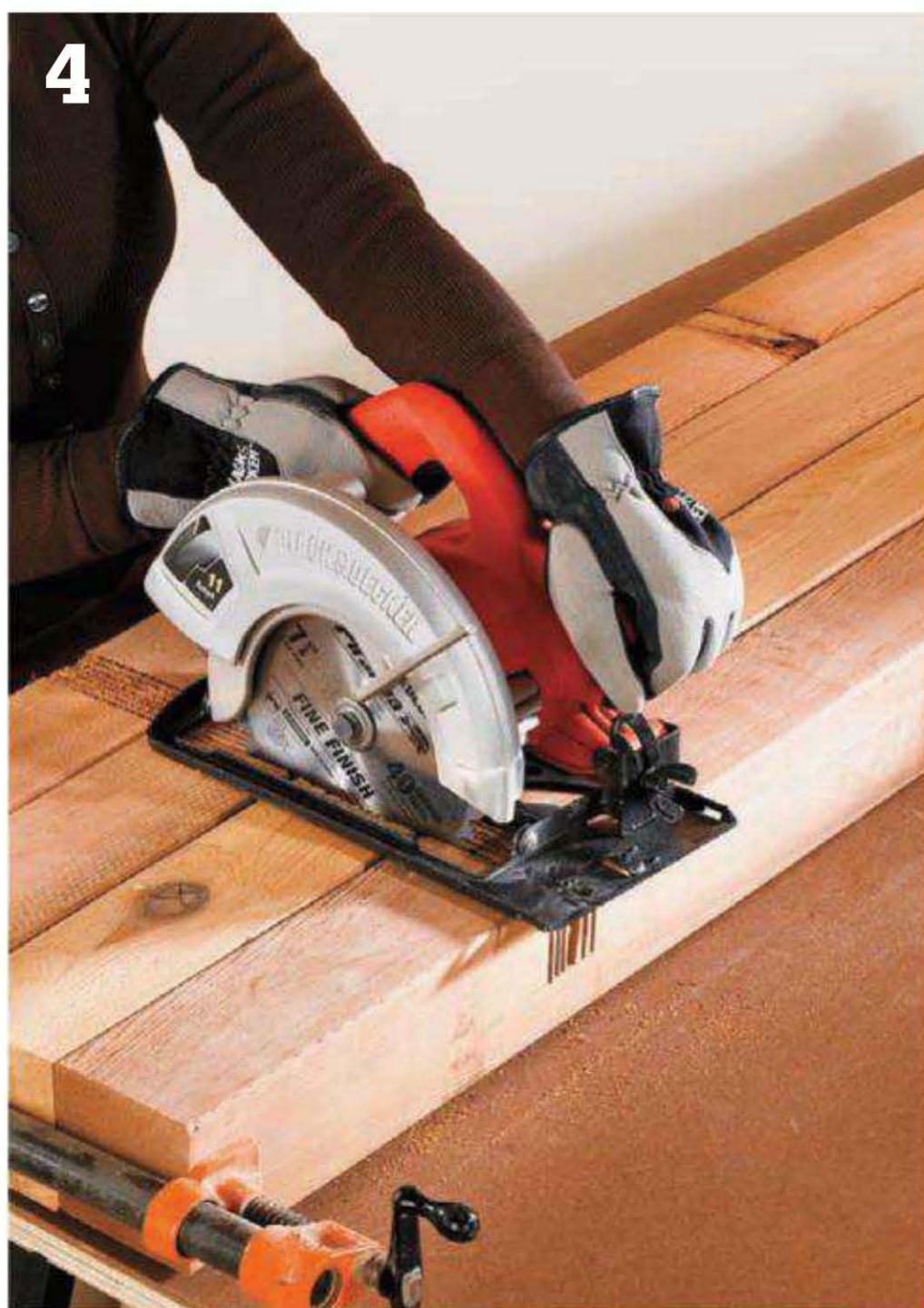
Cut notches into the seat beams. Remove waste material from the notch area by making multiple kerf cuts with a circular saw set to 2¼" cutting depth.
