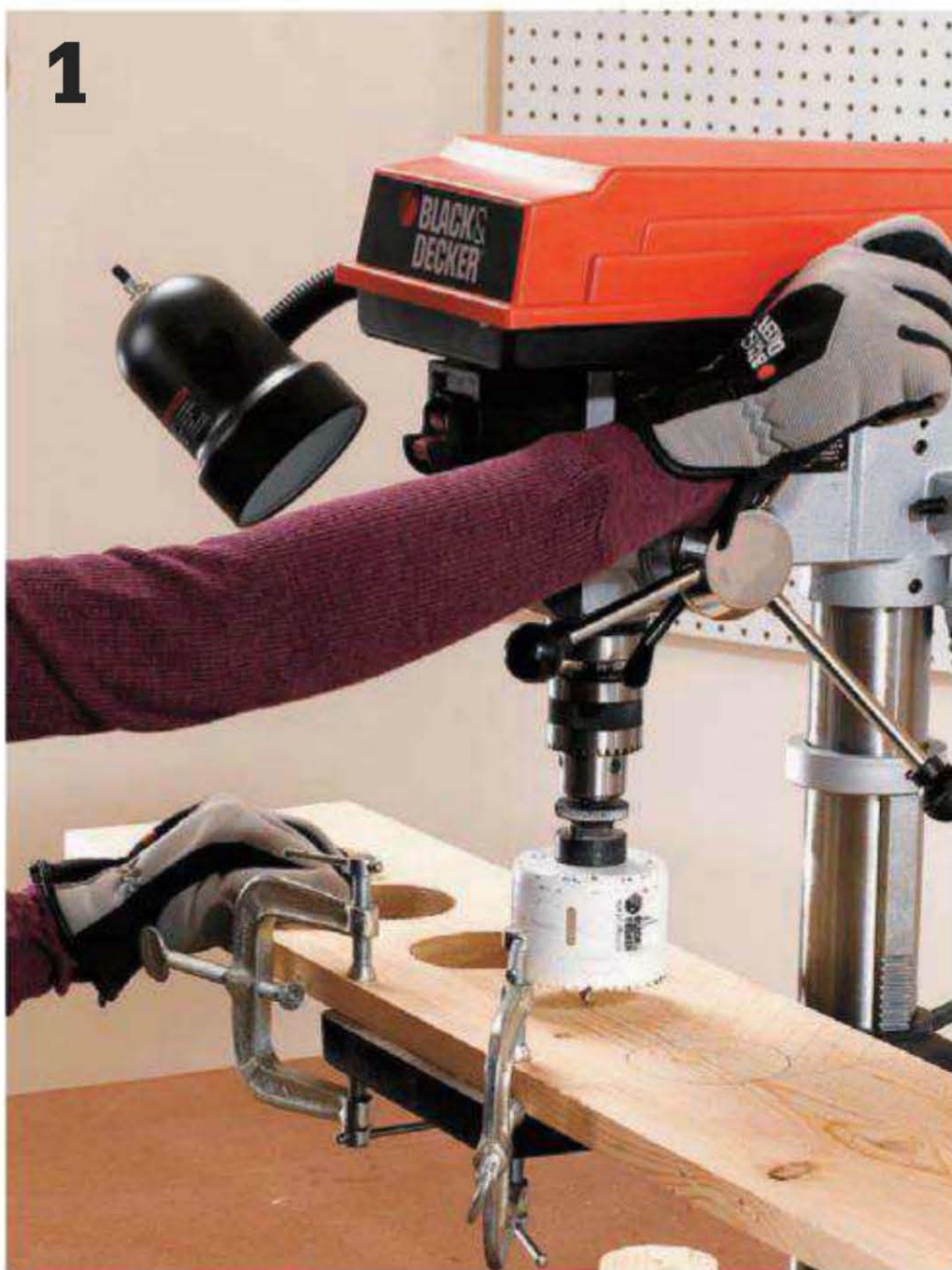
Cut out 3"-dia. circles along a centerline on a 1 × 8 workpiece to make the top rails. Use a 3" hole saw to cut the wood.
