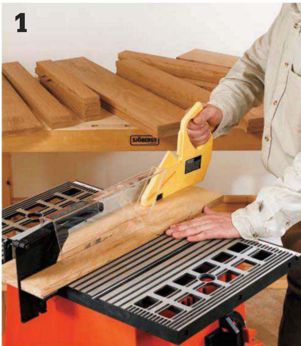
Dimension your lumber. If you purchased sanded-four-side (S4S) stock, you will only need to rip it to the correct widths after you cut the parts to length.
