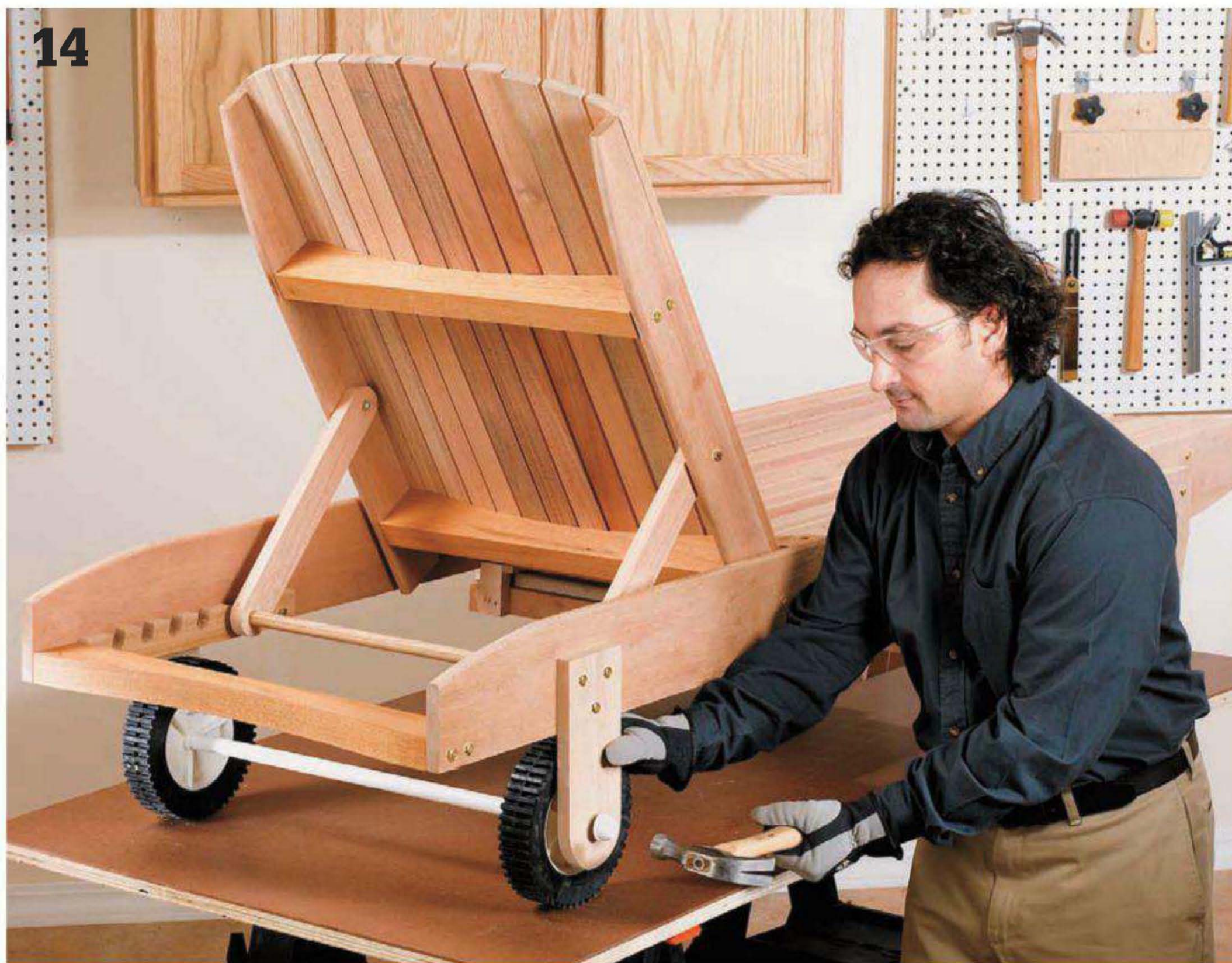
Install the wheels. Make sure the spacers (½" inside-diameter washers) are in place on each side of the wheel and then fasten flanged push caps onto the ends of the rod to secure the wheels to the axle.
