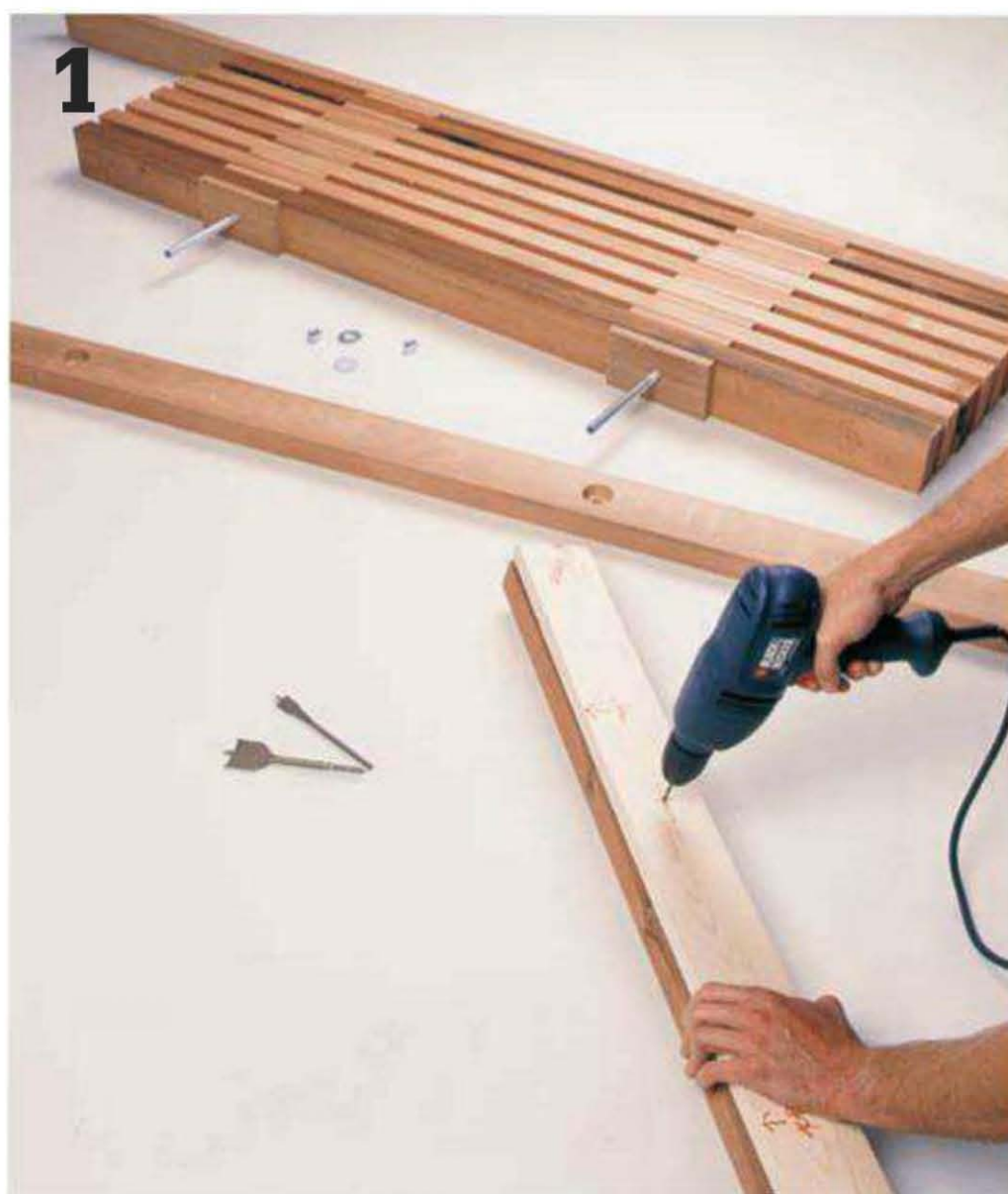
Drill guide holes for the threaded rods in the rails and fillers using templates as guides.
