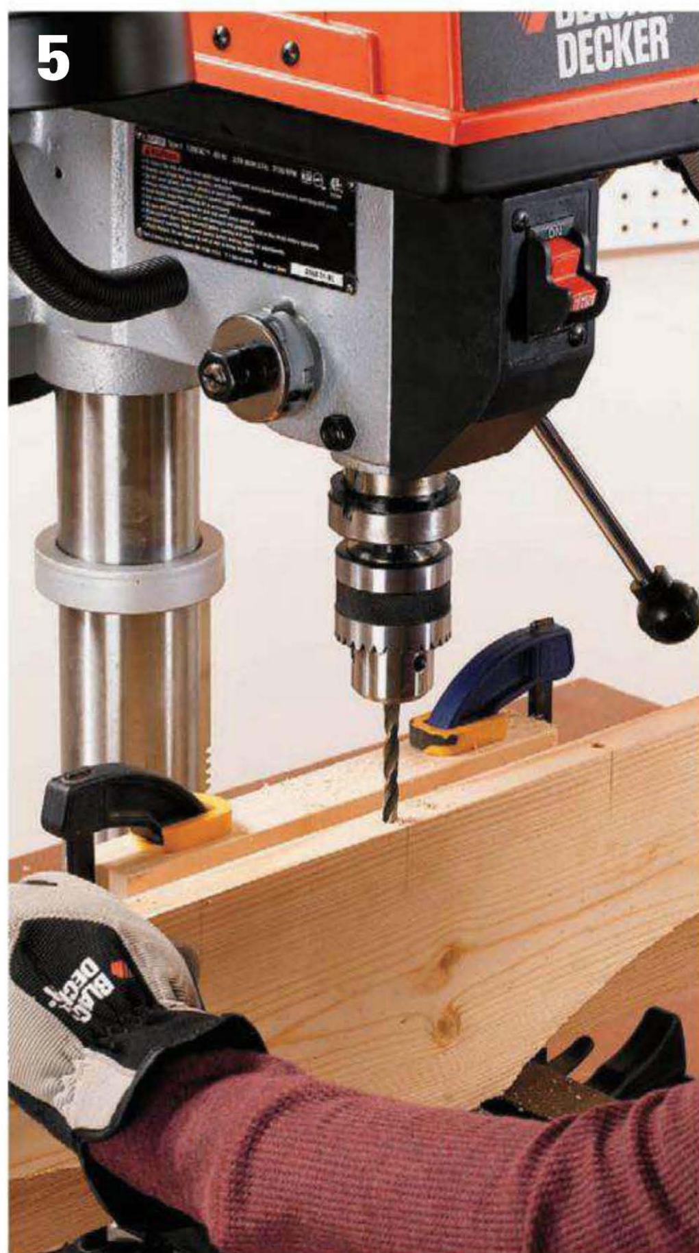
Drill dowel holes in the top and bottom rails to make dowel joints with the filler stiles and the corner boards.
