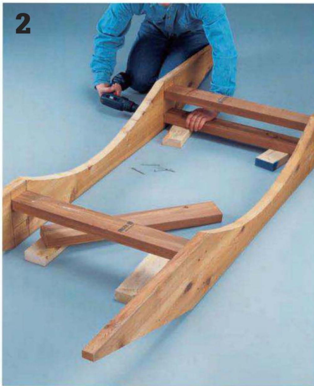
Attach pairs of stretchers between the stringers with 3" deck screws.
