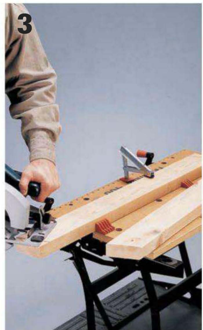
3 Miter-cut the middle supports and roof supports with a circular saw or with a power miter saw.
