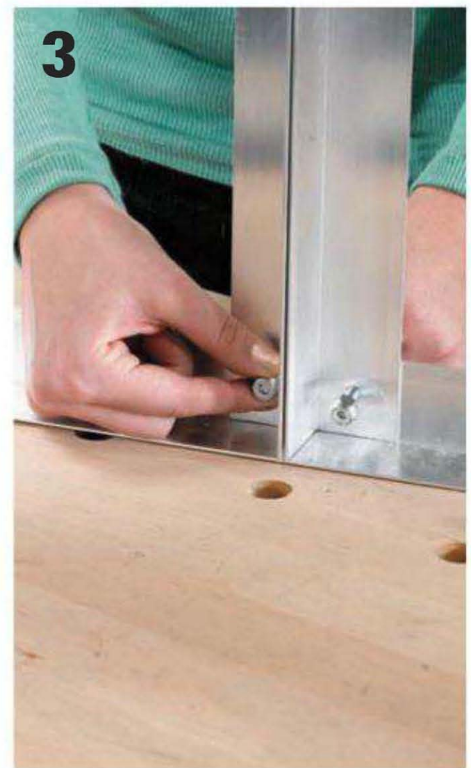
Assemble the frame. Secure each frame joint with a \frac{1}{4} \times \frac{3}{4} " bolt and lock nut. If you're able to locate aluminum fasteners use them, otherwise use stainless steel or hot-dipped fasteners.
