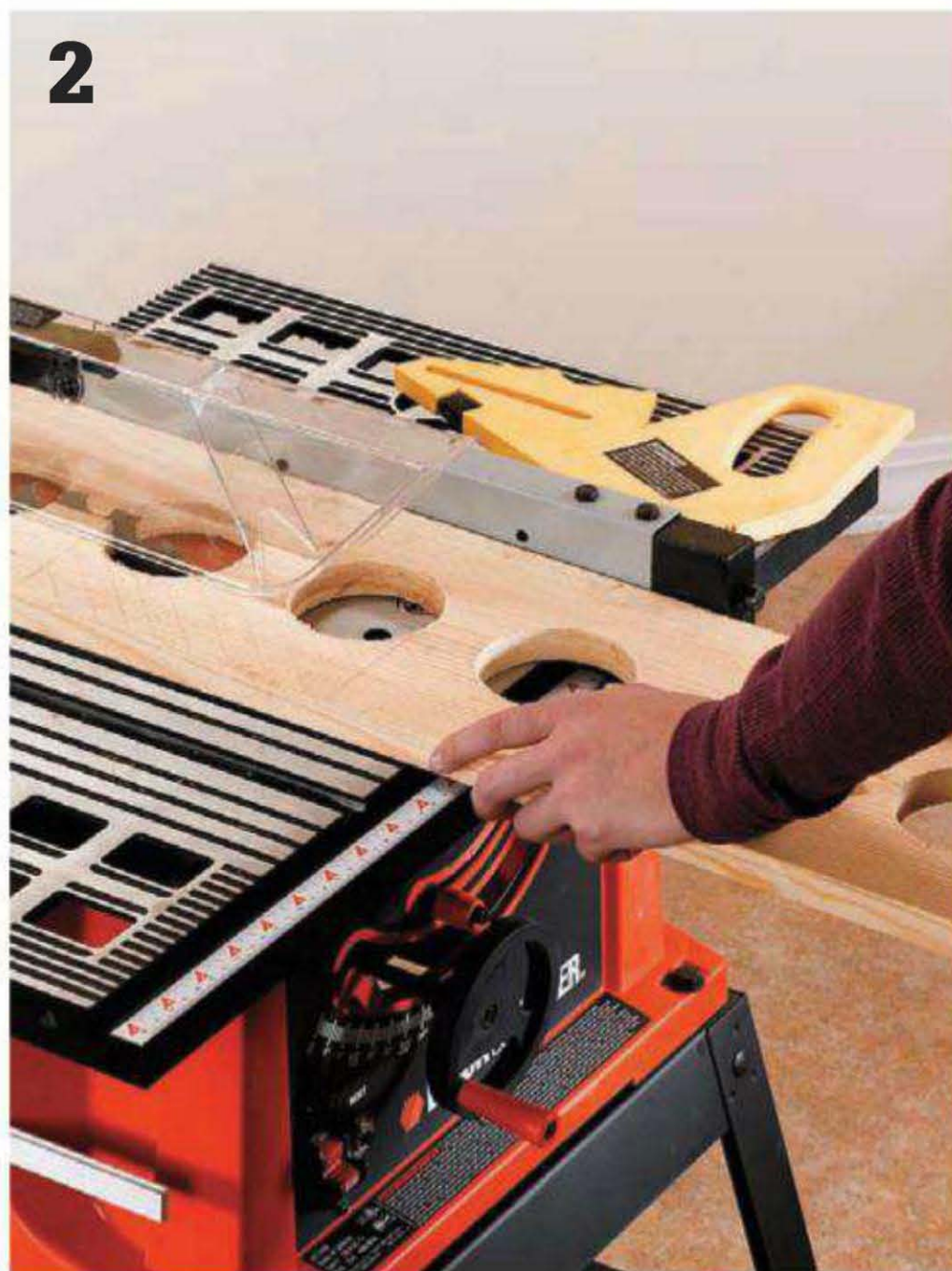
Rip-cut the rail workpiece along the centerline to create two workpieces with half-round cutouts. Use one for the front top rail and the other to make the side top rails.
