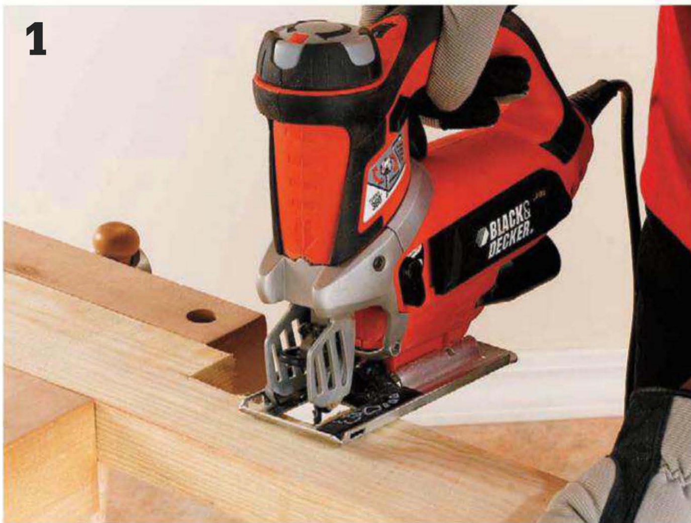
Cut the base rail notch. Draw the notch edge lines on each leg. Use a jigsaw to cut along the notch layout lines.
