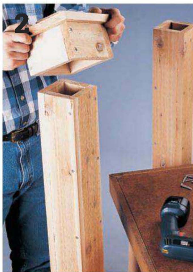
Fit the top collar assemblies onto each post and attach them. Drill pilot holes for all fasteners in the collar assemblies so they don't split apart when you drive screws.
