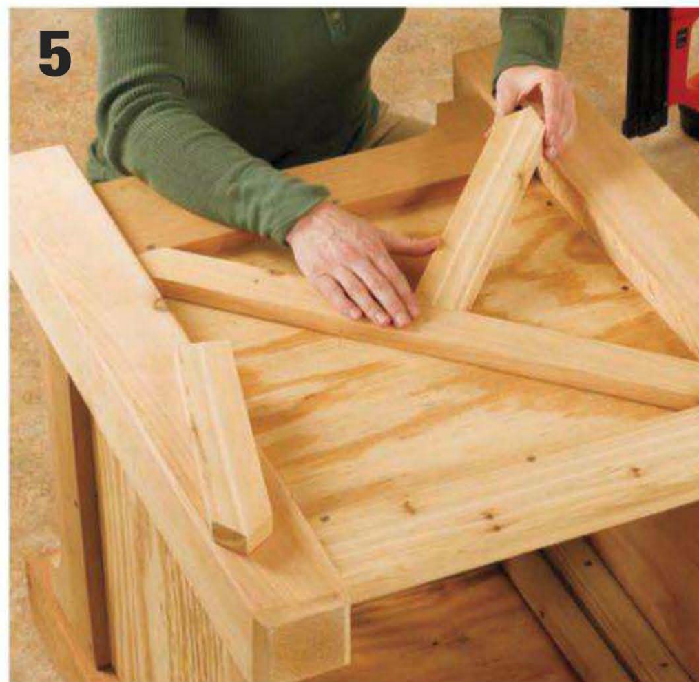
Make the X shape. The distinctive X shape on the outer surfaces of the side panels is made with 2" wide strips of cedar that are fastened with adhesive and 1" brass brads.
