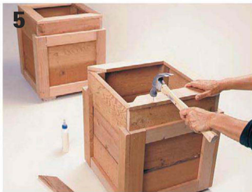
Miter-cut the cap trim boards and nail them in place on the box tops.
