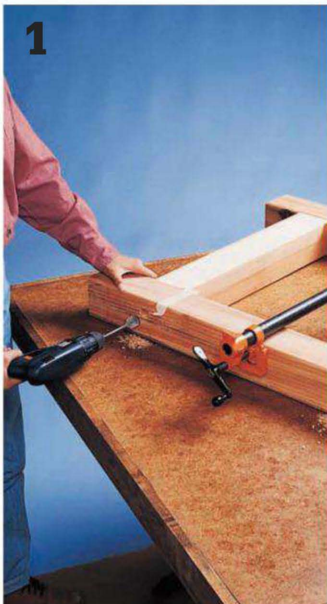
Counterbore two sets of holes on each leg to recess the lag screws when you attach the legs to the stretchers.
