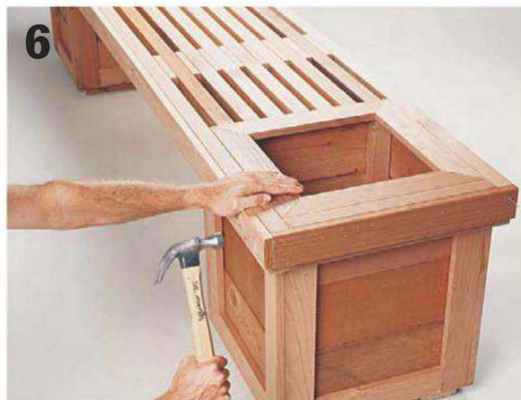
Attach the planters to the outer rails of the seat using deck screws. Fasten the rail strips with finish nails to hide the bench top hardware and fasteners.
