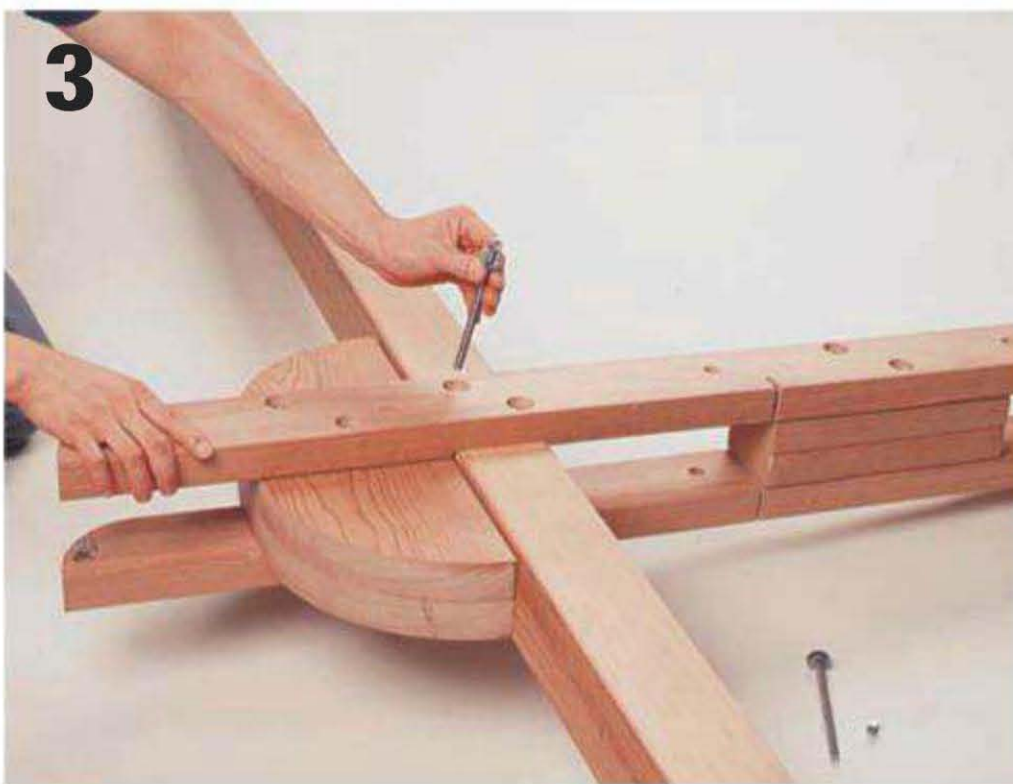
Fasten the post, rails, and braces with lag bolts. Drill counterbores for the bolt heads and the nuts.
