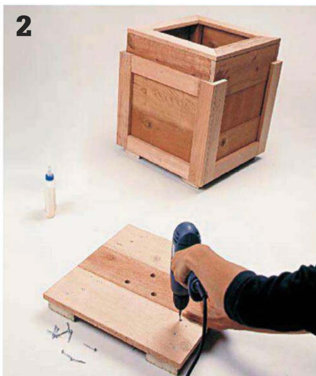
Attach three base strips on top of a pair of feet to create platforms to use as the box bases.
