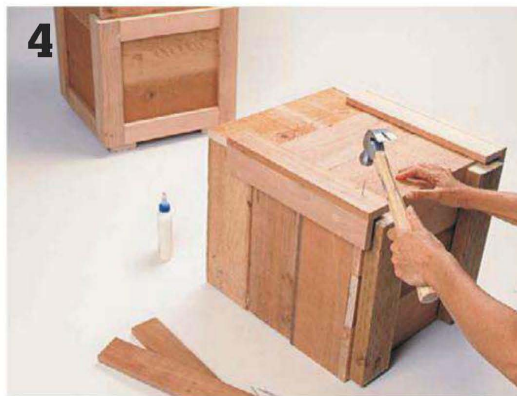
Attach the corner trim boards and the top and bottom trim boards to each planter assembly.
