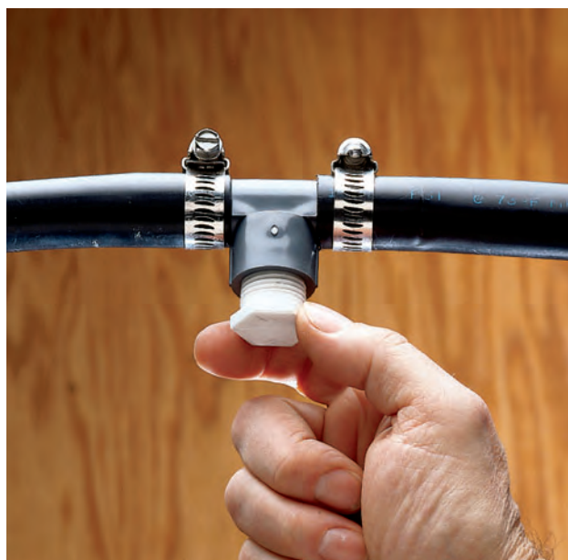
Connect lengths of PE pipe with a barbed PVC fitting. Secure the connection with stainless steel hose clamps.
