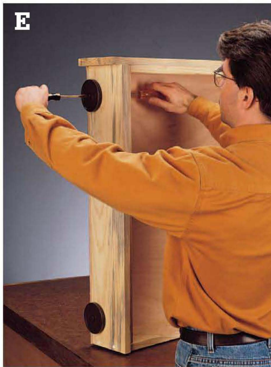
Mount bed-box rollers on the outside faces of the sides so the rollers extend \frac{1}{2} " below the box bottom.
