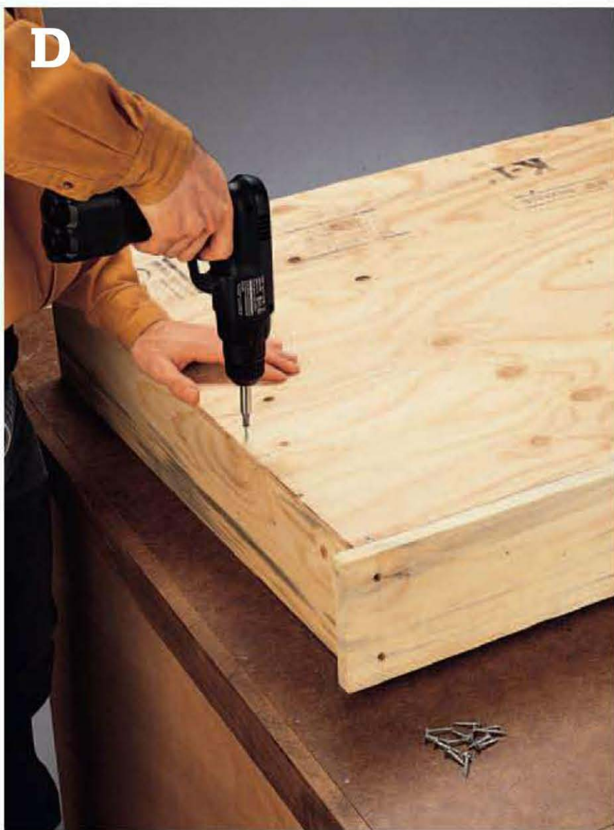
Fasten the bottom panel to the box frame and divider.
