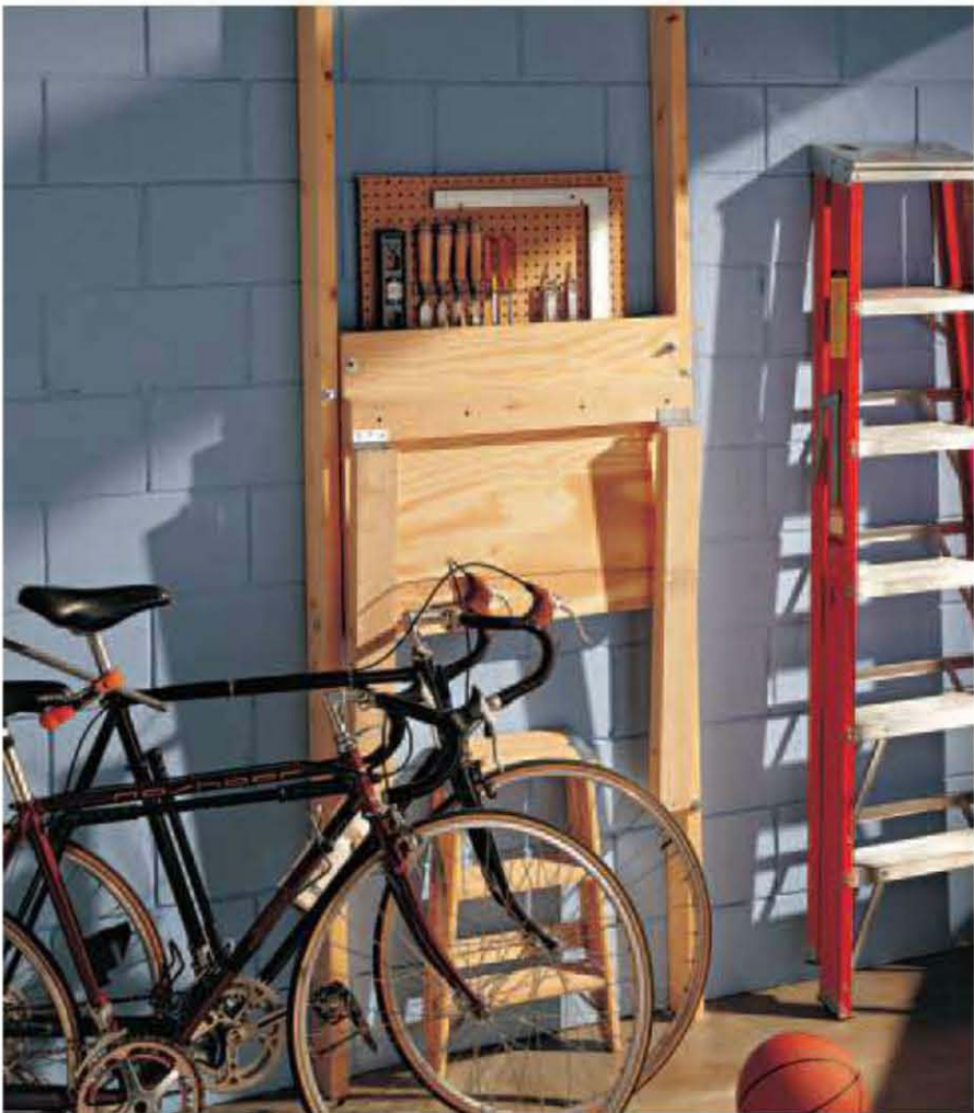
Make the most of limited workshop space by building a fold-down work shelf. The work shelf can be mounted from exposed wall studs, or from a frame attached to masonry walls. When it is not in use, fold the work shelf up and out of the way.
