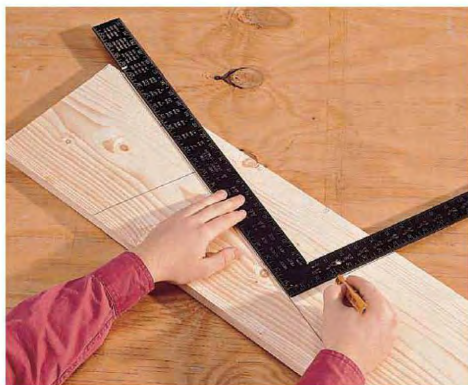
A. Lay out the dimensions of the cornice pieces on 1× finish-grade lumber using a framing square.
