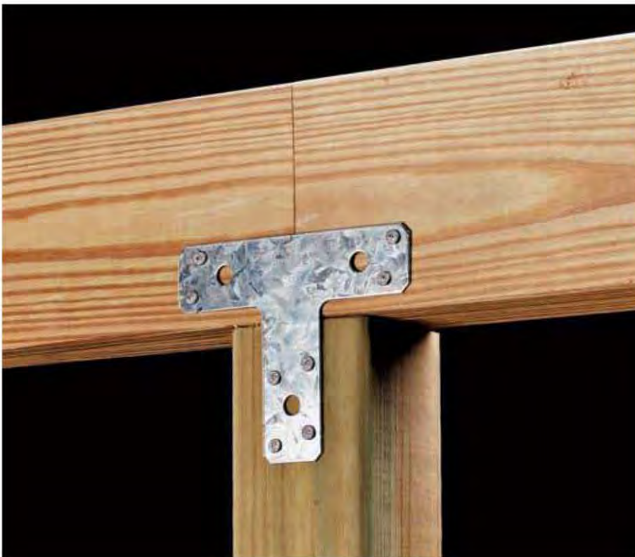
T-straps reinforce the connection between beam and post, particularly on long beams requiring spliced construction. Local building codes may also allow their use in place of post caps.
