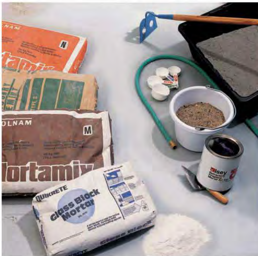
Ingredients for mixing your own mortar include portland cement, sand, and water. For high temperature, add refractory mix.
