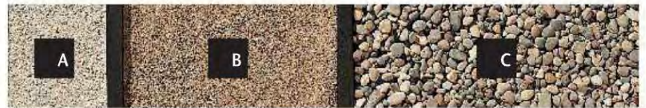
To mix concrete ingredients in a wheelbarrow, use a ratio of 1 part portland cement (A), 2 parts sand (B), and 3 parts coarse gravel (C).
