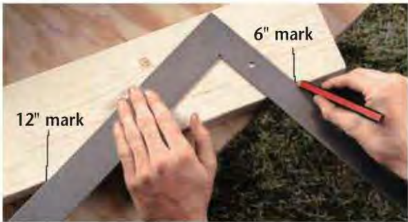
A. Position the framing square at the 6 and 12" marks to draw the top and bottom plumb-cut lines.
