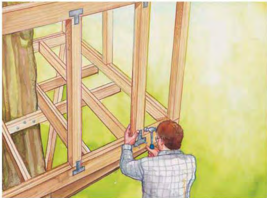
E. Mark the middle posts where they cross the timber beams. Cut the posts at the marks, then fasten them in place using metal connectors.
