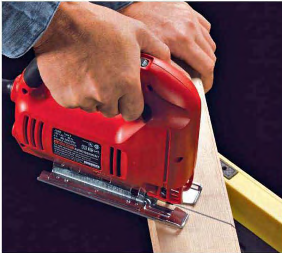
20. Use a jigsaw to cut the stairway rail along the marked outlines.
