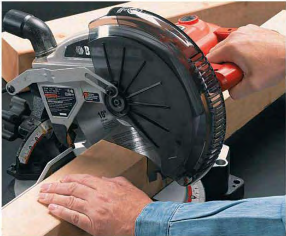
2. Cut posts with power miter saw or circular saw. Make sure factory-treated ends of posts are square. If necessary, square them by trimming with a power miter saw or circular saw.
