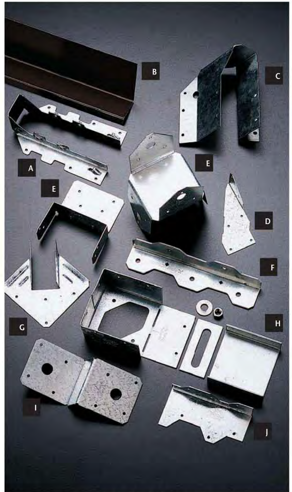
Metal connectors commonly used include: joist hanger (A), flashing (B), angled joist hanger (C), rafter tie (D), post-beam caps (E), stair cleat (F), hurricane tie (G), post anchor with washer and pedestal (H), joist tie (I), angle bracket (J).
