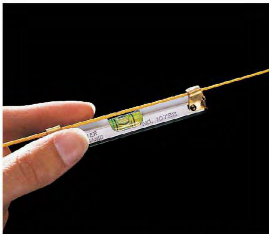
12. Hang a line level on the mason's string. Raise or lower string until it is level. Locate other outside post footing, repeating steps 5 to 12.
