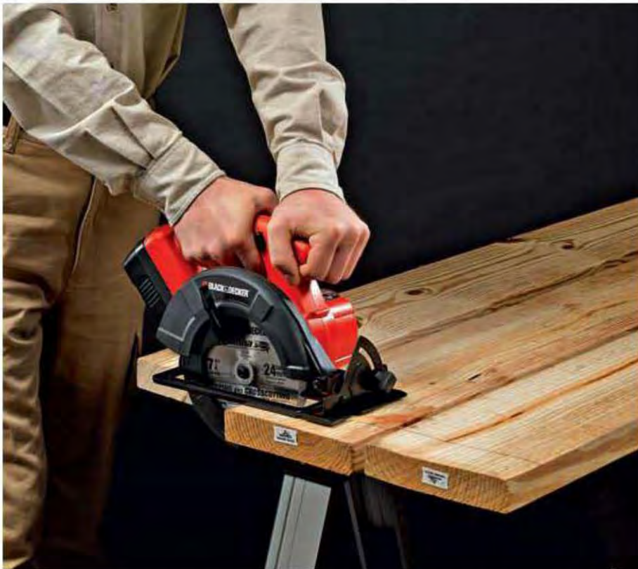
14. Measure and mark lumber for joists using a combination square as a guide. Cut joists with a circular saw or power miter saw.
