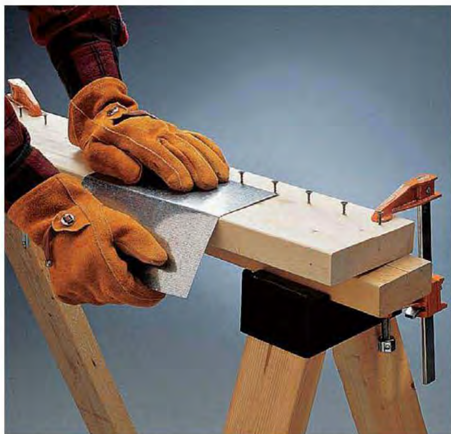
Make a flashing-bending jig with screws lined up along a piece of scrap wood.
