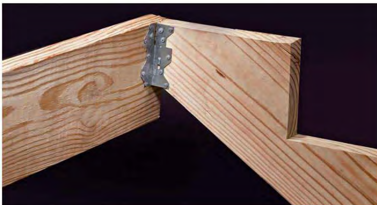
Framing anchors can be used to fasten rim joists together at corners or make other right-angle attachments, such as stair stringers to rim joists.
