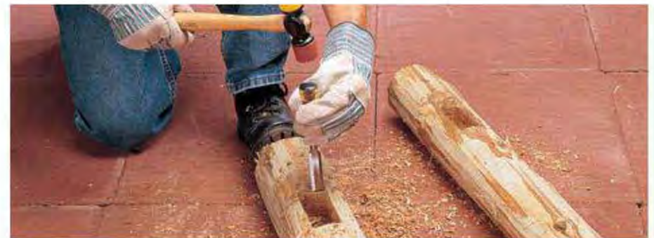
B. Remove as much waste wood as you can in the mortise area by drilling 1"-dia. holes all the way through. Square the mortises with a wood chisel.
