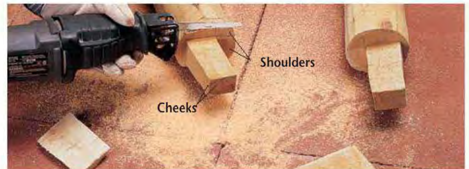
C. Using a reciprocating saw, make cheek cuts then shoulder cuts to create tenons on the ends of the rails.
