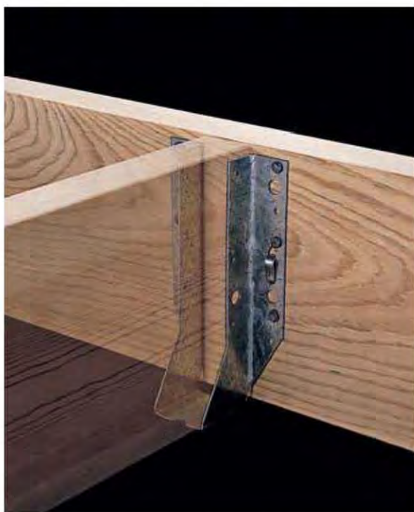
Joist hangers are used to attach joists to the ledger and header joist. Double hangers are used when decking patterns require a double-width joist.
