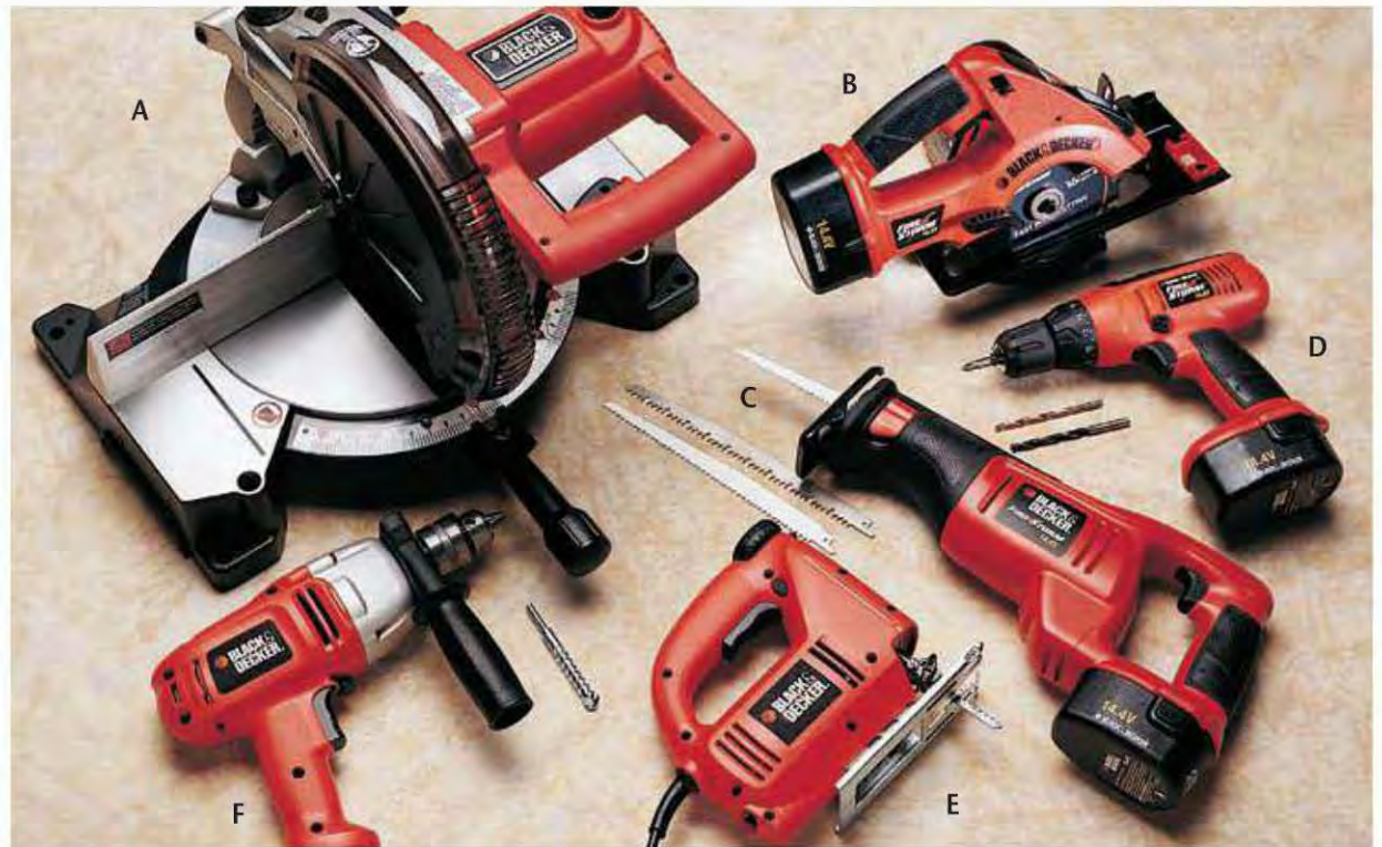
Power tools include: power miter saw (A), 14.4-volt cordless trim saw with a 5\frac{3}{8} "-blade (B), reciprocating saw with 6" and 8" blades (C), cordless drill/driver (D), jigsaw (E), \frac{1}{2} " hammer drill and bits (F).
