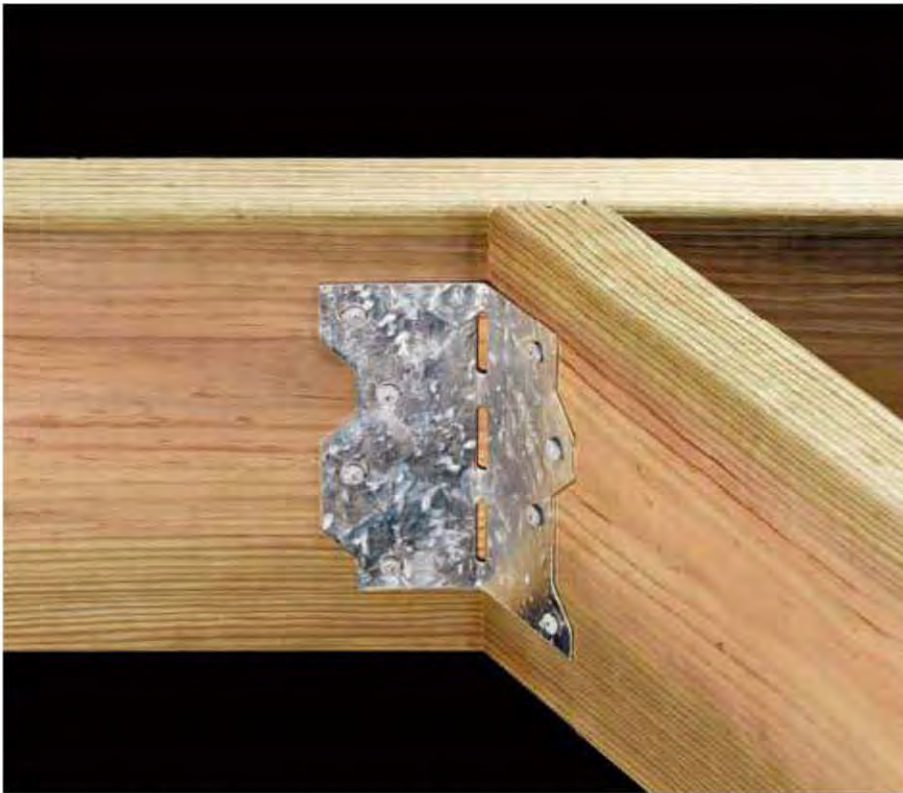
Skewable angle brackets reinforce framing connections at angles other than 90° or at beam ends where 45° joist hangers won't fit.
