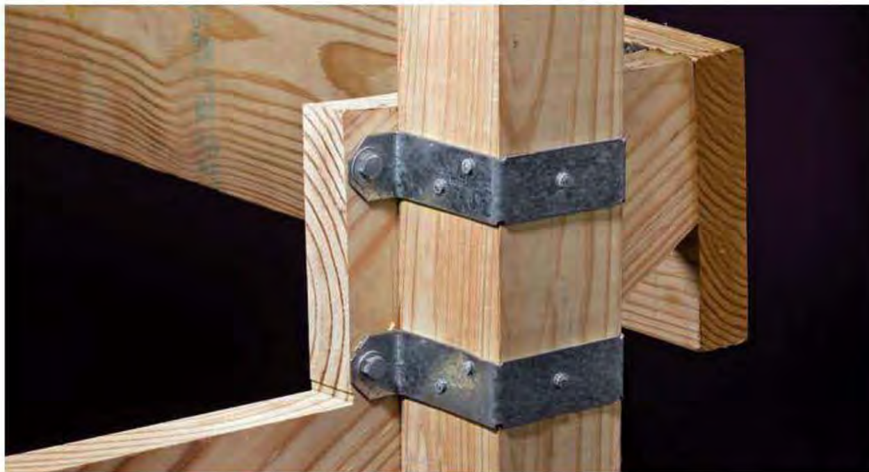
Deck post ties fasten stair or railing posts to stringers or joists without through bolts. Hardware is manufactured in 2 × 4 and 4 × 4 size options.
