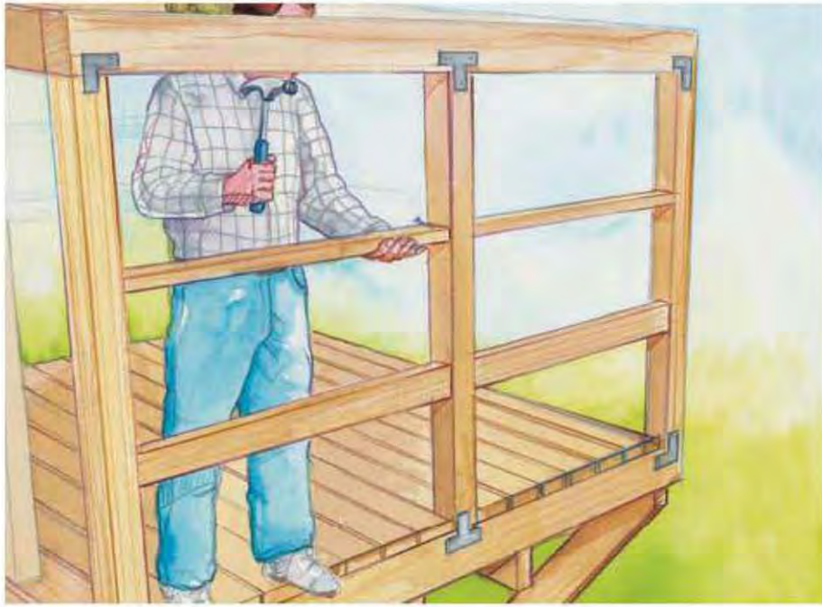
H. Install the girts and top plates between the rails on all four sides of the tree house.
