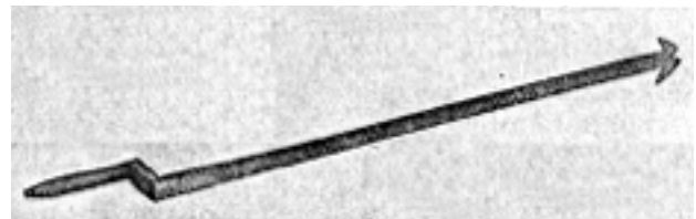
Fig. 7. How to remove old or broken slates with the tool shown above.
