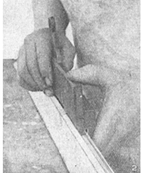
Tongued Joint, Fig. 1. Plane used in preparing tongue. Fig. 2. Use of grooving plane.
