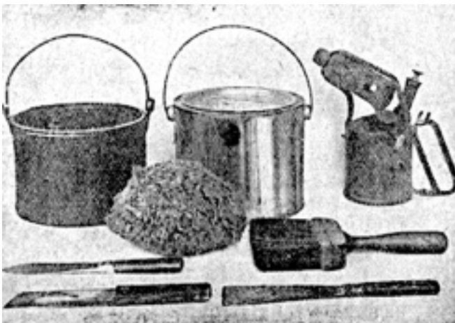
Paint. Fig. 1. Implements which are essential for the amateur painter. Reading in rows from left to right: paint kettle, tin of paint, blow lamp, putty knife, sponge, dusting brush, hacking knife, stripping knife.
