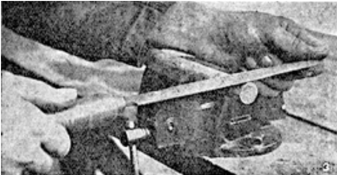
Fig. 3. The end of the pipe must be filed up before screwing is begun.
