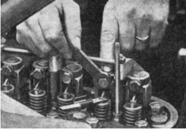
Motor Car. Fig. 14. Method of adjusting valve clearances with a feeler gauge. Tappets of an overhead valve system are being adjusted.
