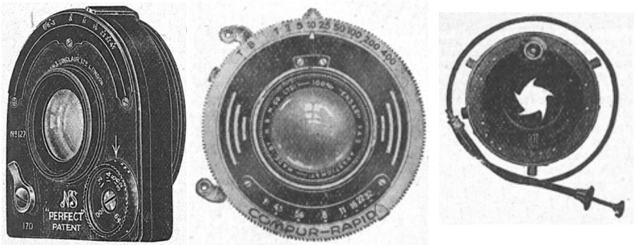
Shutter. Left, the "N.S." shutter with lens in Sinclair "Una" camera gives speeds from 1/2 t o 1/100 sec. Middle, Ensign between-lens, Compur type, with escapement mechanism. Right: "Luc" silent 5-blade shutter; clamped over lens.
