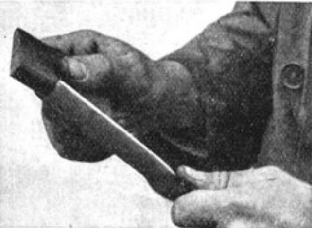
Fig. 4. Showing use of oilstone slip for sharpening edge of hollow-ground gouge.
