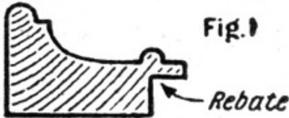
Picture Framing. Fig. 1. Section through moulding, showing rebate.
