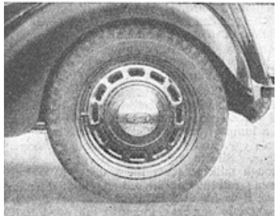
Wheel. Fig. 1. Spoked disk type, now used on most motor vehicles. Made from single steel pressing.
