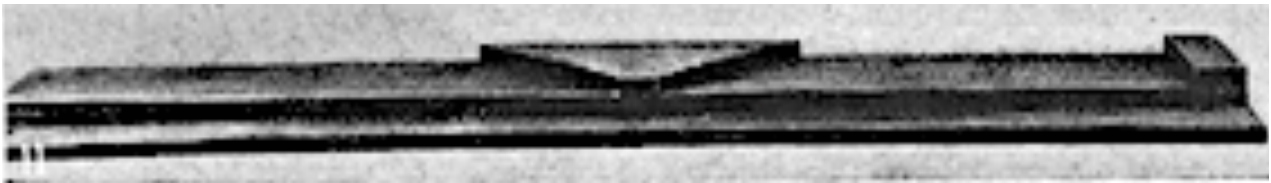
Fig. 11. Mitre shooting board used for planing.
