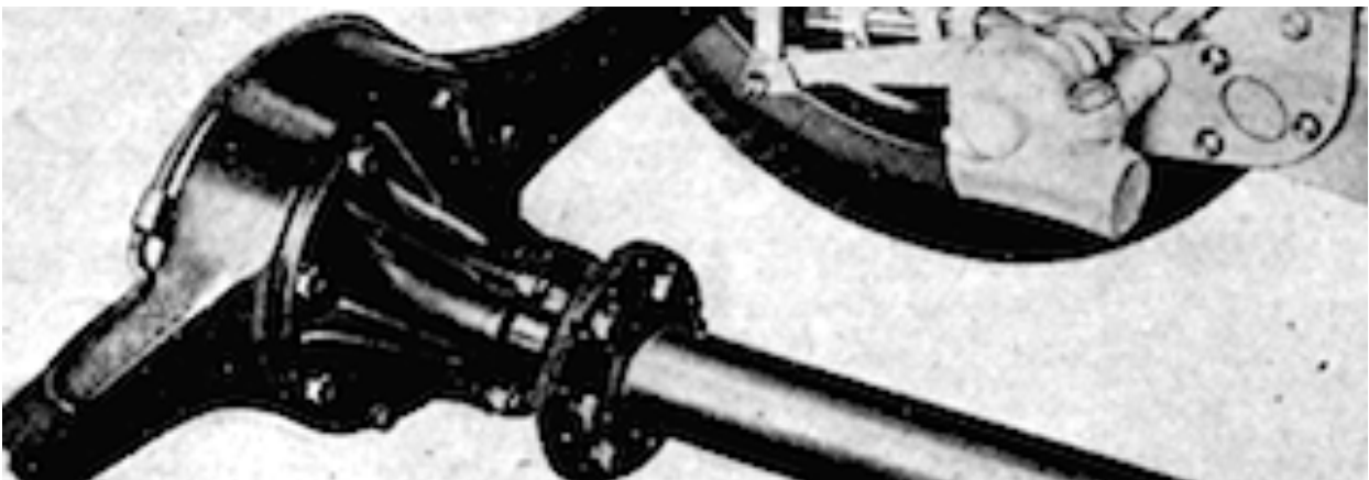
Below. Live Axle. Fig. 2. General view of Fiat live axle casing of the banjo type.
