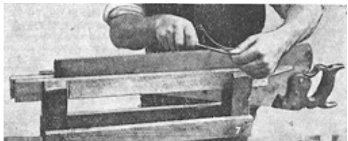
Saw. Fig. 6. Setting the teeth of a saw with a hand saw set. Fig. 7. Showing correct method of using the file in sharpening a saw.
