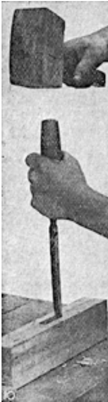
Mortise. Fig. 10. Showing method of using mortise chisel. Fig. 11. How the tenons are cut. Fig. 12. Mortise gauge, which marks two lines simultaneously.
