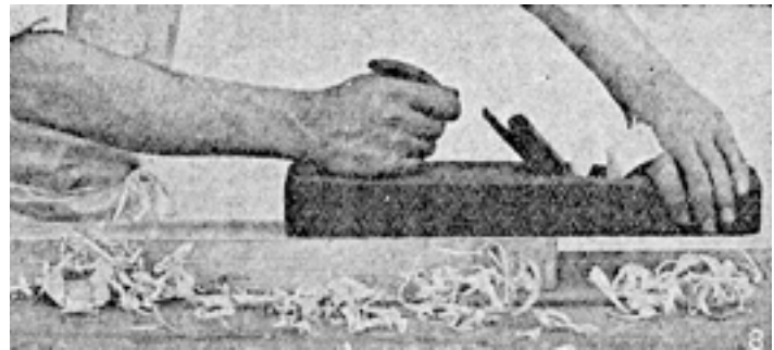
Fig. 8. How the plane is held at the finish of the stroke.
