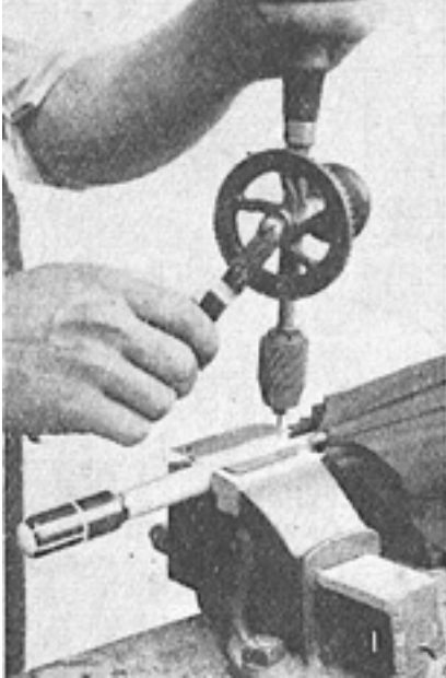
Umbrella. Fig. 1. Drilling a fine hole for a new rivet in the handle. Fig. 2. Filing down the rivet head, the handle being protected by a piece of cardboard. Fig. 3. Removing the tapered cap covering the ring that supports the ribs. Fig. 4. Withdrawing the tying wire. Fig. 5. Fixing the tying wire to the notch.
