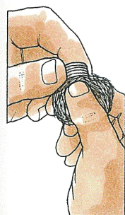
2 Cleaning the threads Use wire wool to clean any corrosion from the threads of the blanking plugs and valve adaptors.
