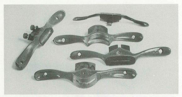
Spokeshaves. Extreme left: an all-purpose shave with a flat sole and two adjusting nuts. Top to bottom: a slightly convex shave, shop-made by modifying the sole and blade of a flat shave; a half-round shave; an adjustable-throat shave; a round-face shave.
