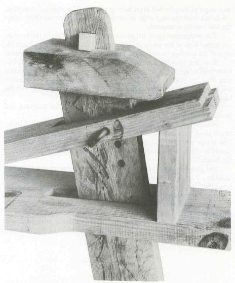
Off-center pivot holes cause the head to open automatically.
