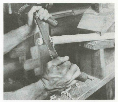
Pushing a drawknife into the shoulder of a tenon. A push stroke can also be used where edge grain rises away from the end of a piece of wood.
