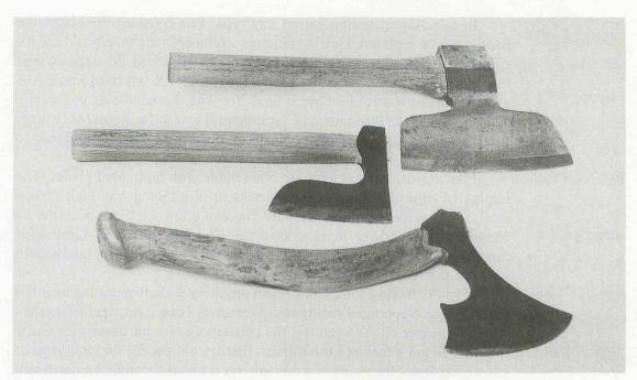
Three of my favorite bench axes. The axe at the top is a broad hatchet, made in Germany before World War II. It has a single bevel and a laminated blade. The middle axe is a Japanese carpenter's hatchet. The lower hatchet is a reproduction of a 12th century Viking axe from Sweden. The blade is double beveled.
