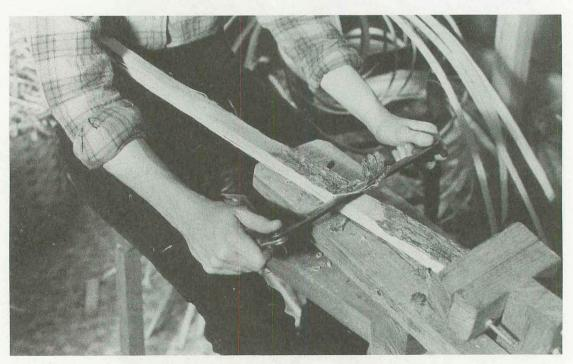
Use a drawknife to remove bark and to shave billets to a square cross section. The squares are then rived tangent to the growth rings.
