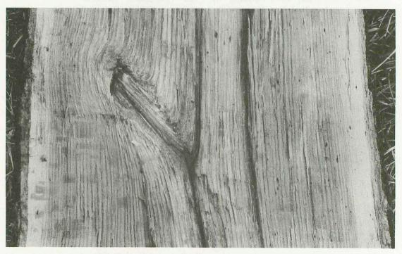
This split log shows how branches (and knots) originate at the pith. Note the distorted grain surrounding the knot.
