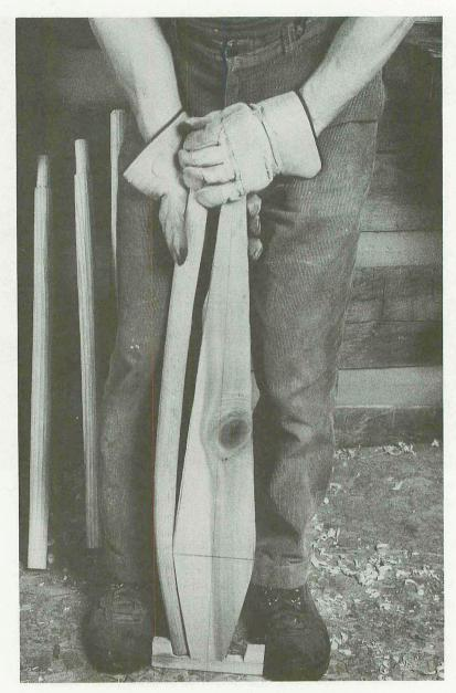
Jigging a ladder-back post. A second post will be bent on the other side. The posts are held in place with pre-knotted loops of twine.
