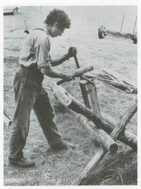
This brake is used to split stock from 2 to 6 feet long. It consists of a forked limb from a black locust and two short poles that are propped inside the fork.
