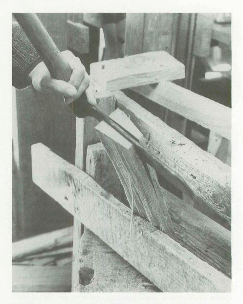
When riving narrow divisions, such as chair slats, place the froe with equal mass on each side of the blade. This brake was made of scrap lumber nailed to a large stump.
