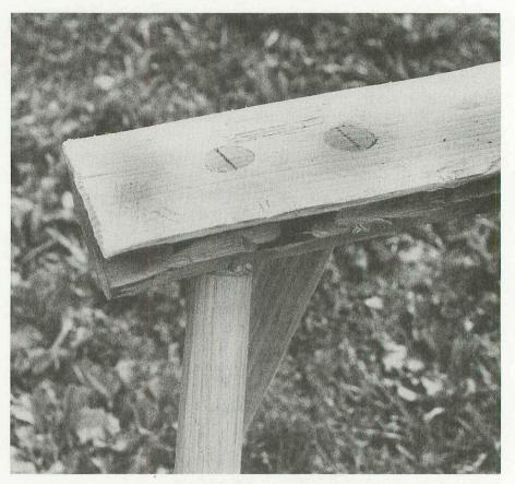
The tenon wedges must be perpendicular to the long fibers of the trestle.
