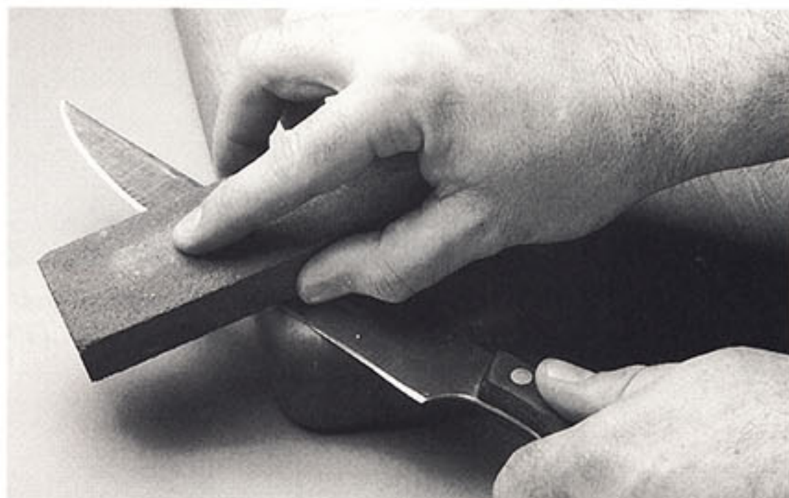
Stroke a coarse stone across the edge of a bread knife to achieve the necessary 'tooth.'
