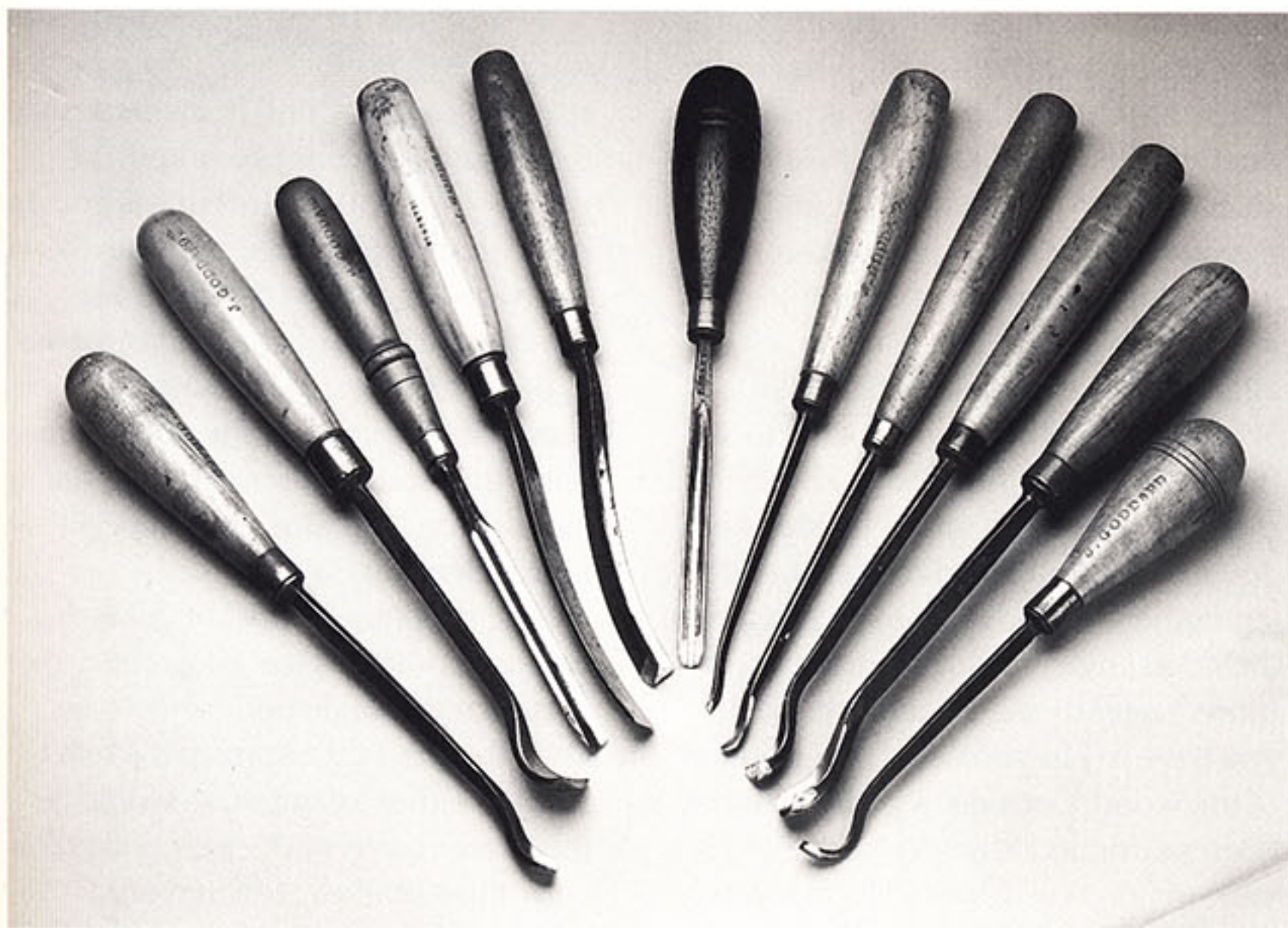
A selection of older carving tools, showing a variety of handle shapes. All but three of the tools were made in the famous Addis factory, the world's foremost maker of carving tools until it closed down a half century ago.
