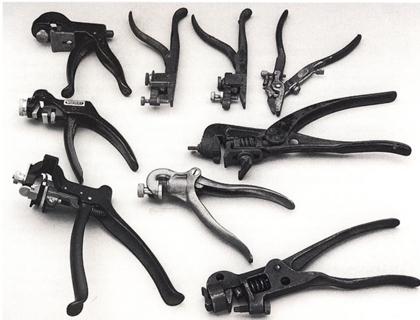
Like jointers, sawsets were (and still are) available in a wide range of styles, from the pistol-grip models at left to the plier styles at right.
