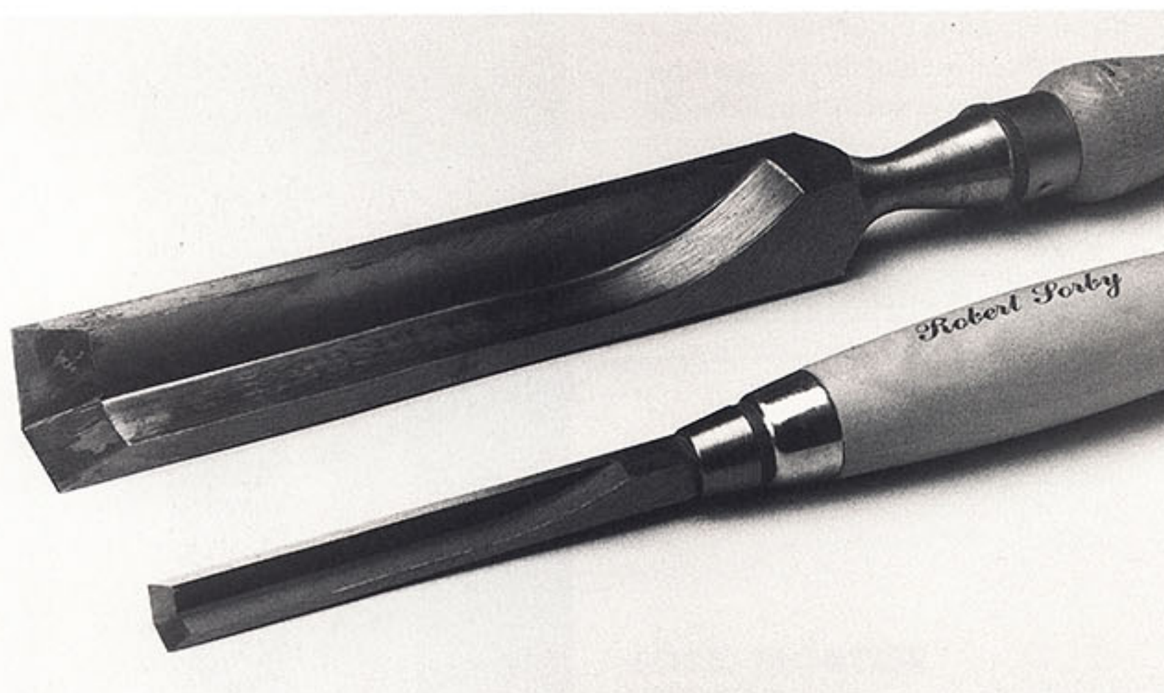
Corner chisels, shown here in 1-in. and \frac{3}{8} -in. sizes, are used to clean the corners in mortises. (Photo by Susan Kahn)
