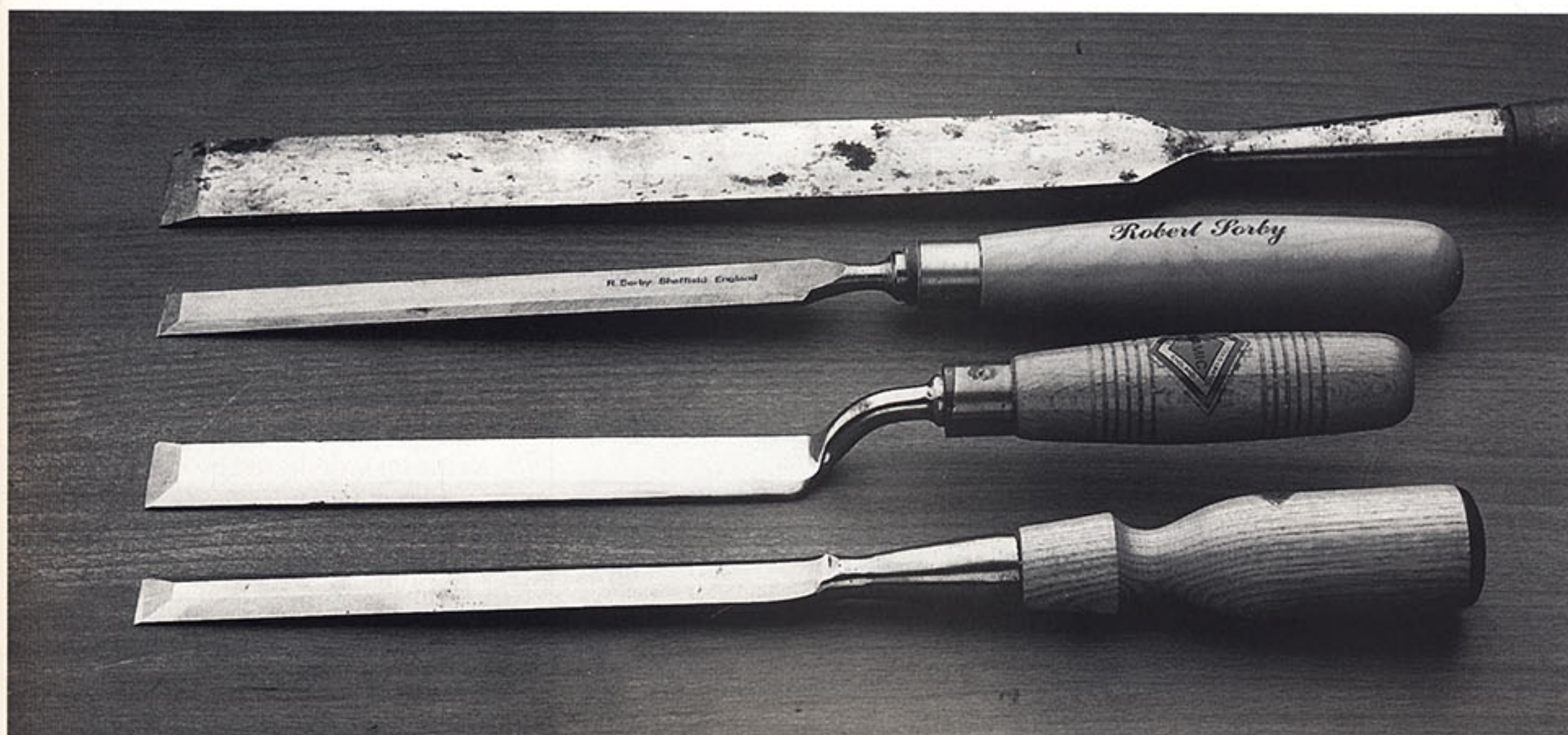
Paring chisels, shown in straight and cranked-neck designs, can be sharpened at relatively low bevel angles. Most people associate the term 'paring' with small, light chisels, yet there used to be much larger and heavier (but still slim) styles used in some trades—chisels like the shipwright's socket paring chisel shown at top.
