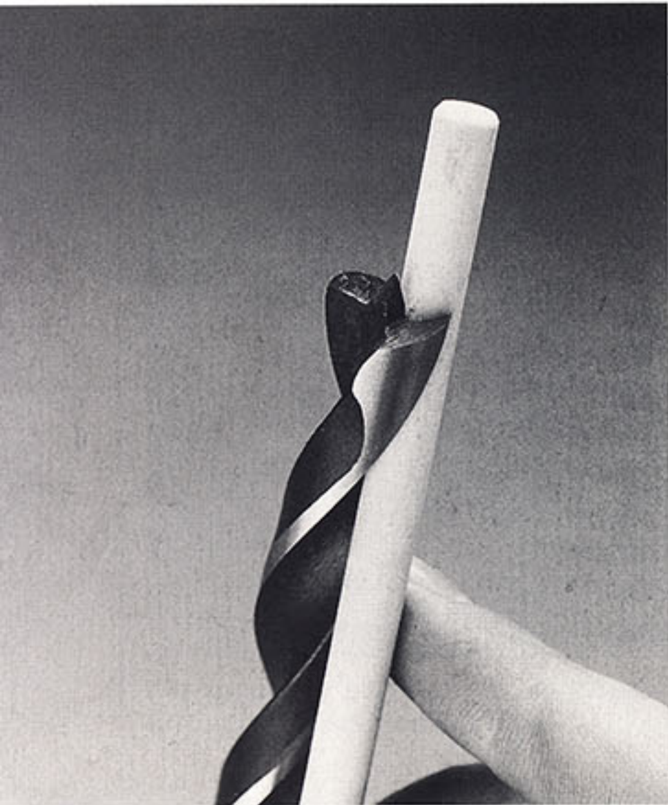
Use a small, round stone in the flute to hone a utility brad-point bit.
