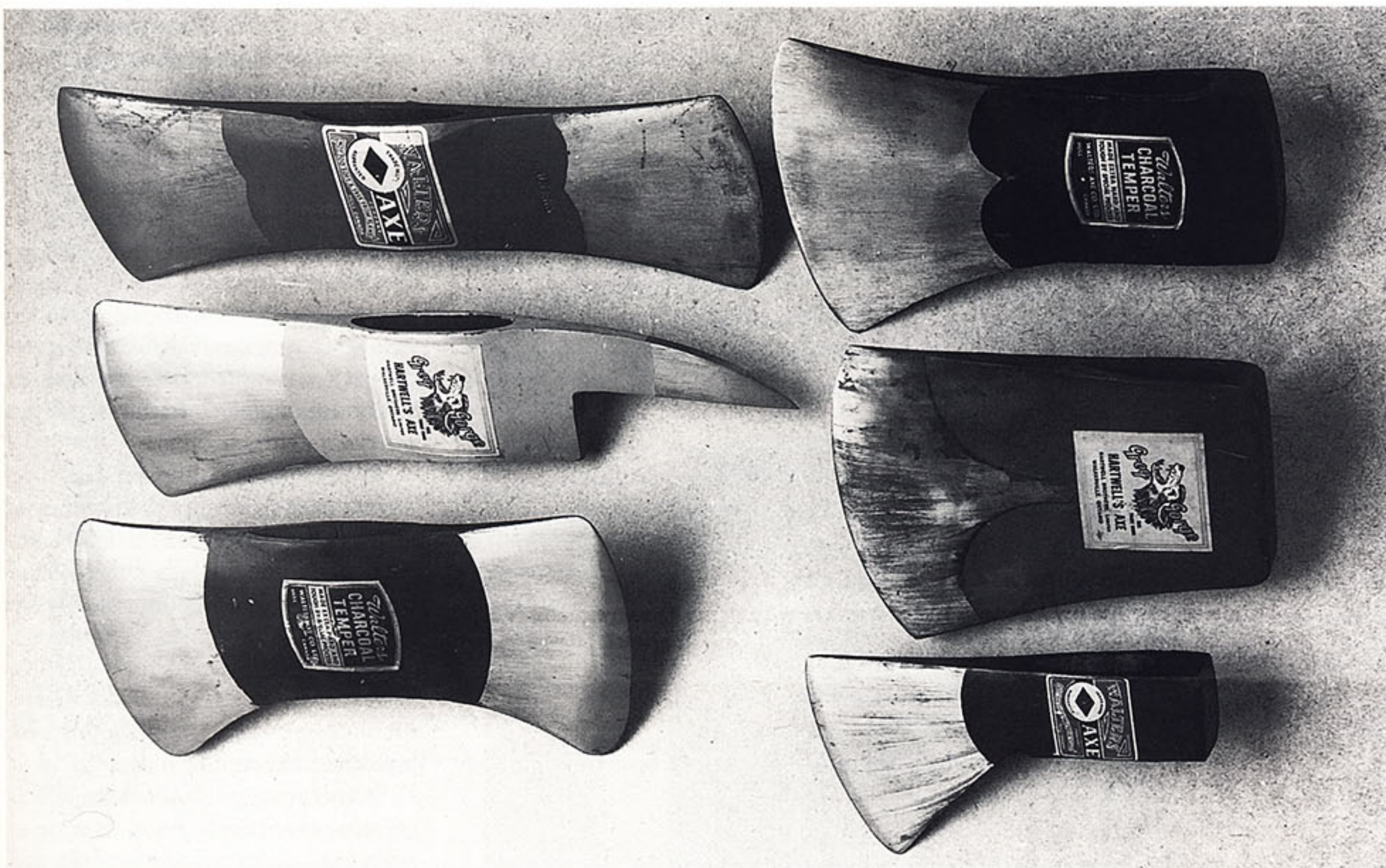
A selection of felling and notching axes. The three double-bit axes at left are (from top to bottom) felling, rafting and swamping styles. The three single-bit axes are (top to bottom) general purpose, full-wedge notching and carpenter's tomahawk pattern.
