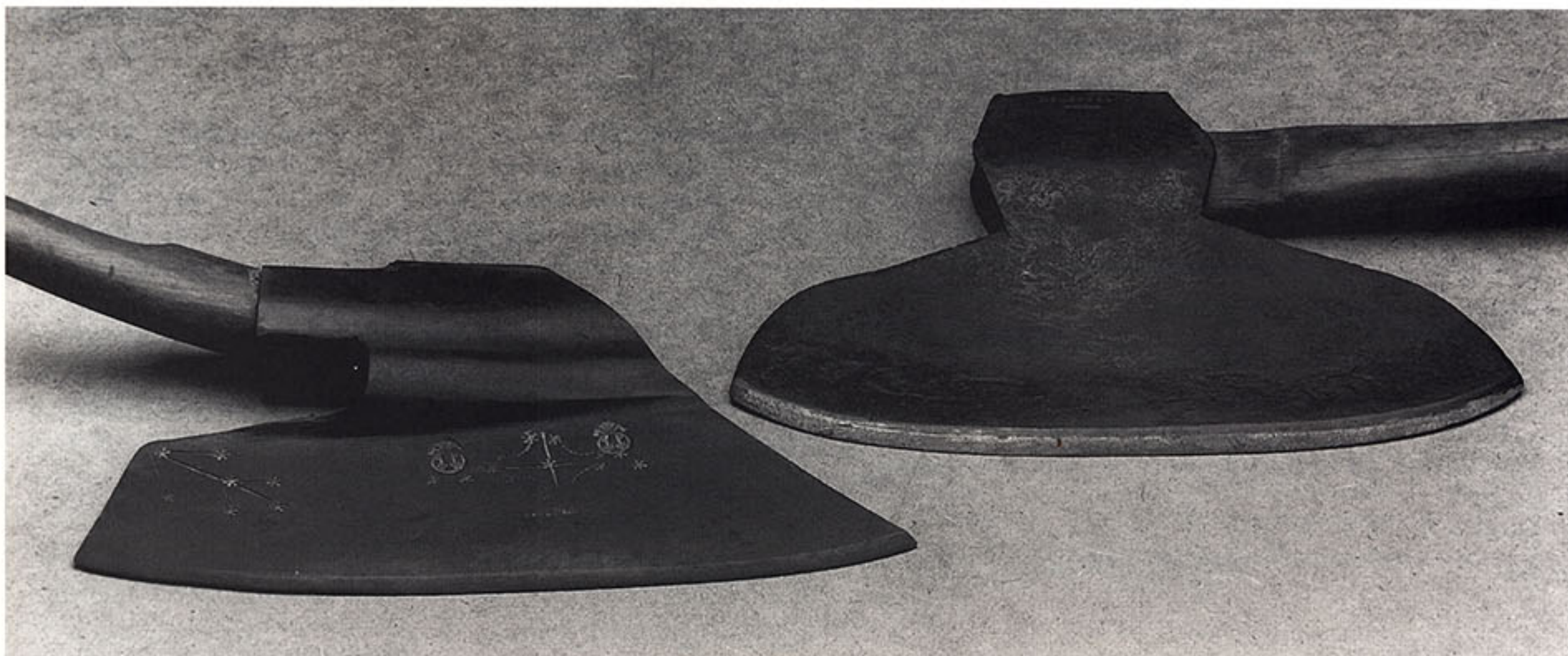
The European bearded ax (left) and the Canada-pattern broad ax (right) are the two most common styles of broad axes.
