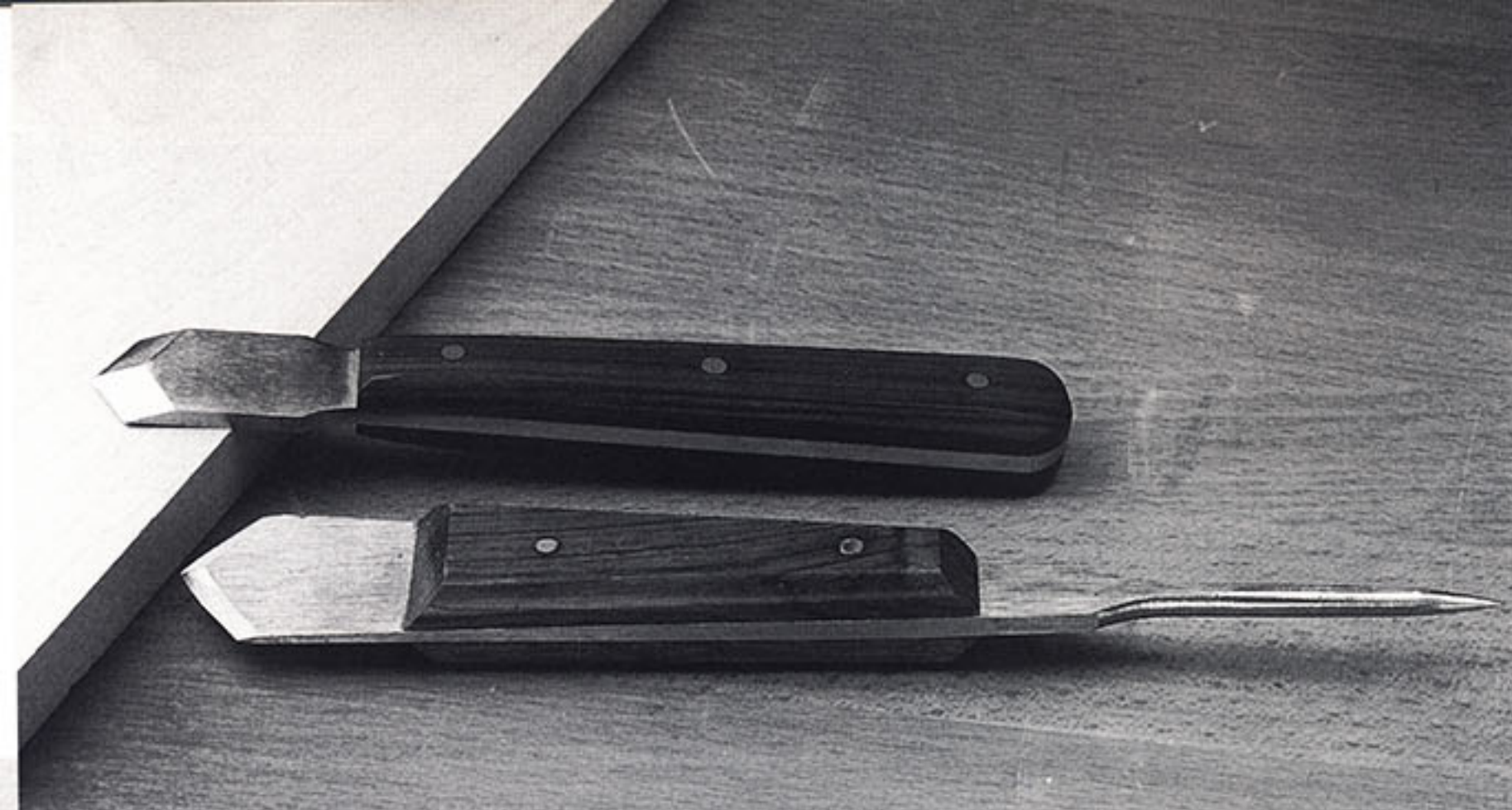
Two styles of marking knife: the top knife is beveled on one side of the blade only, the bottom knife is beveled on both sides and has an integral scratch awl.
