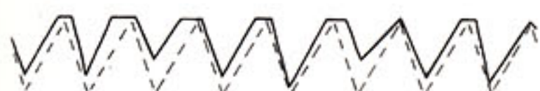
Bad tooth pattern requires reshaping of teeth.
