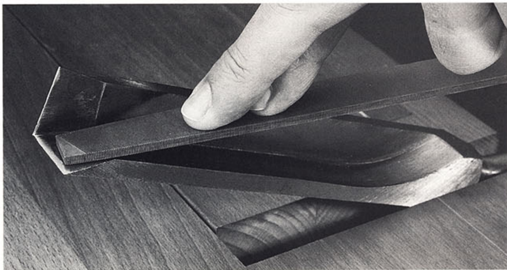
Use a safe-edge mill file to sharpen the inside bevels of a corner chisel.
