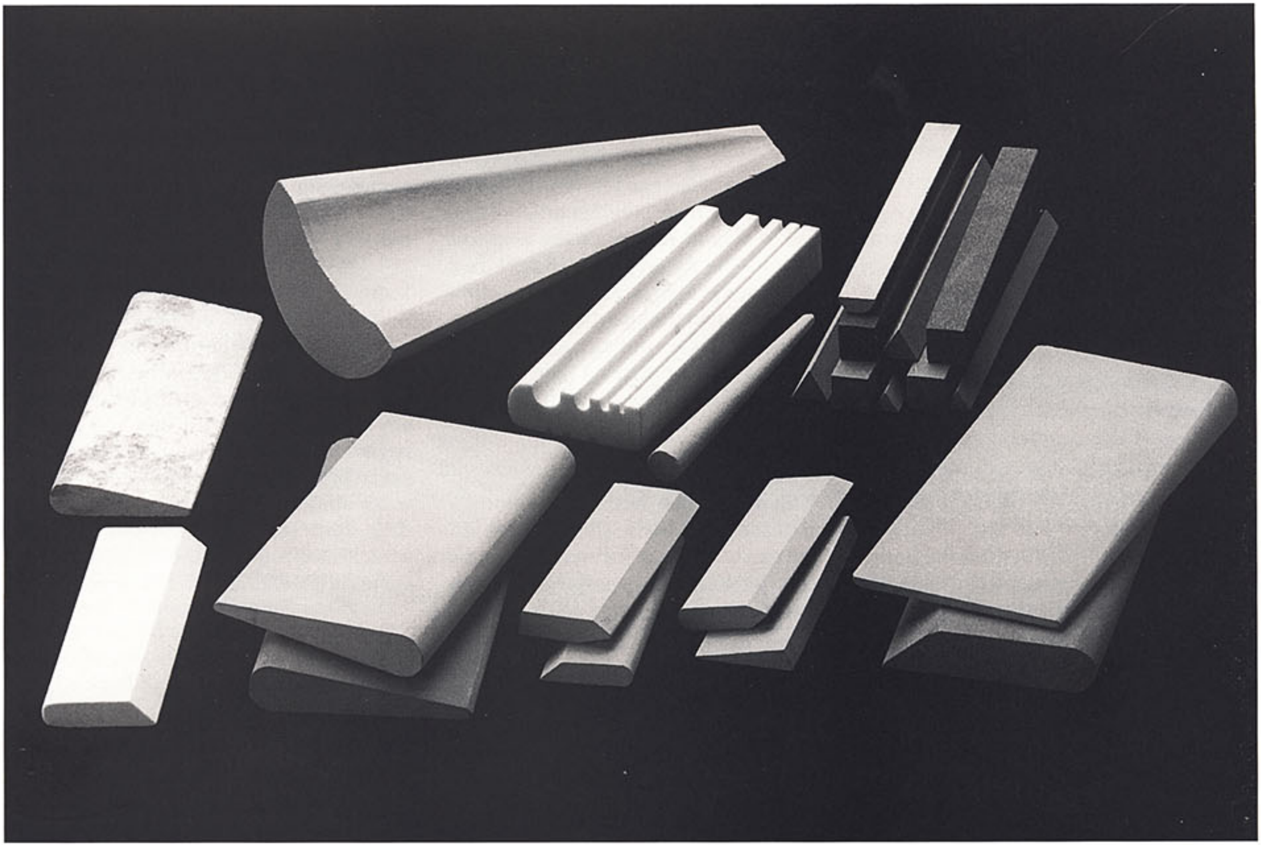
Shaped stones, available in numerous profiles and abrasives, are nowadays used primarily to sharpen turning and carving tools.
