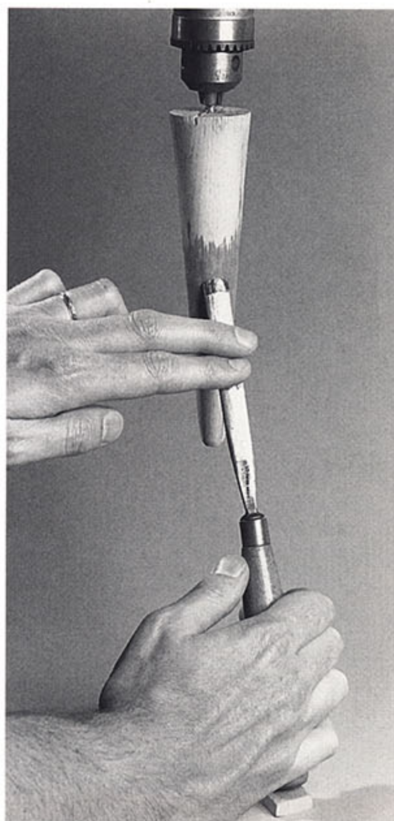
To true the sweep using a drill-press-mounted cone, hold the gouge against the cone at a slight skew so that the cone gives a trailing stroke as it rotates.
