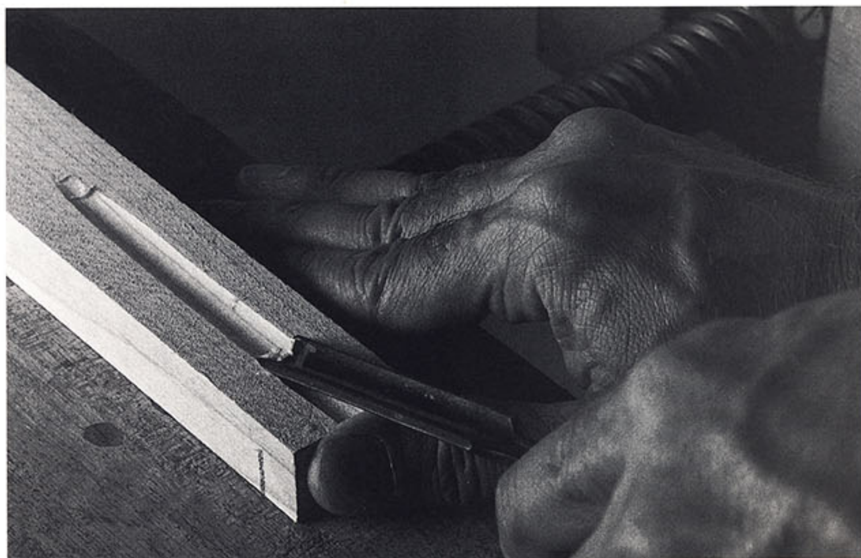
Cutting a groove in the face of a softwood block with a gouge produces a perfectly formed strop for honing the bevel of the same gouge. (Photo by Susan Kahn)
