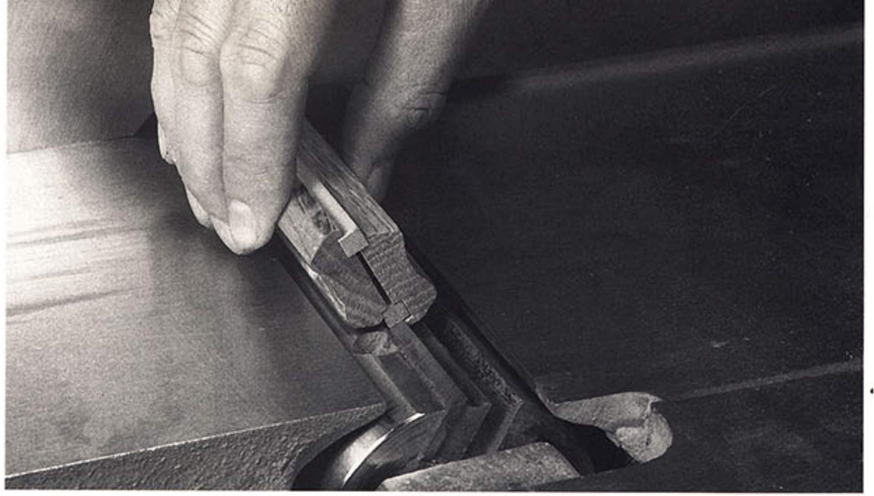
Commercial honing devices can be used to hone the bevel and deburr the knife edge. (Photo by Susan Kahn)
