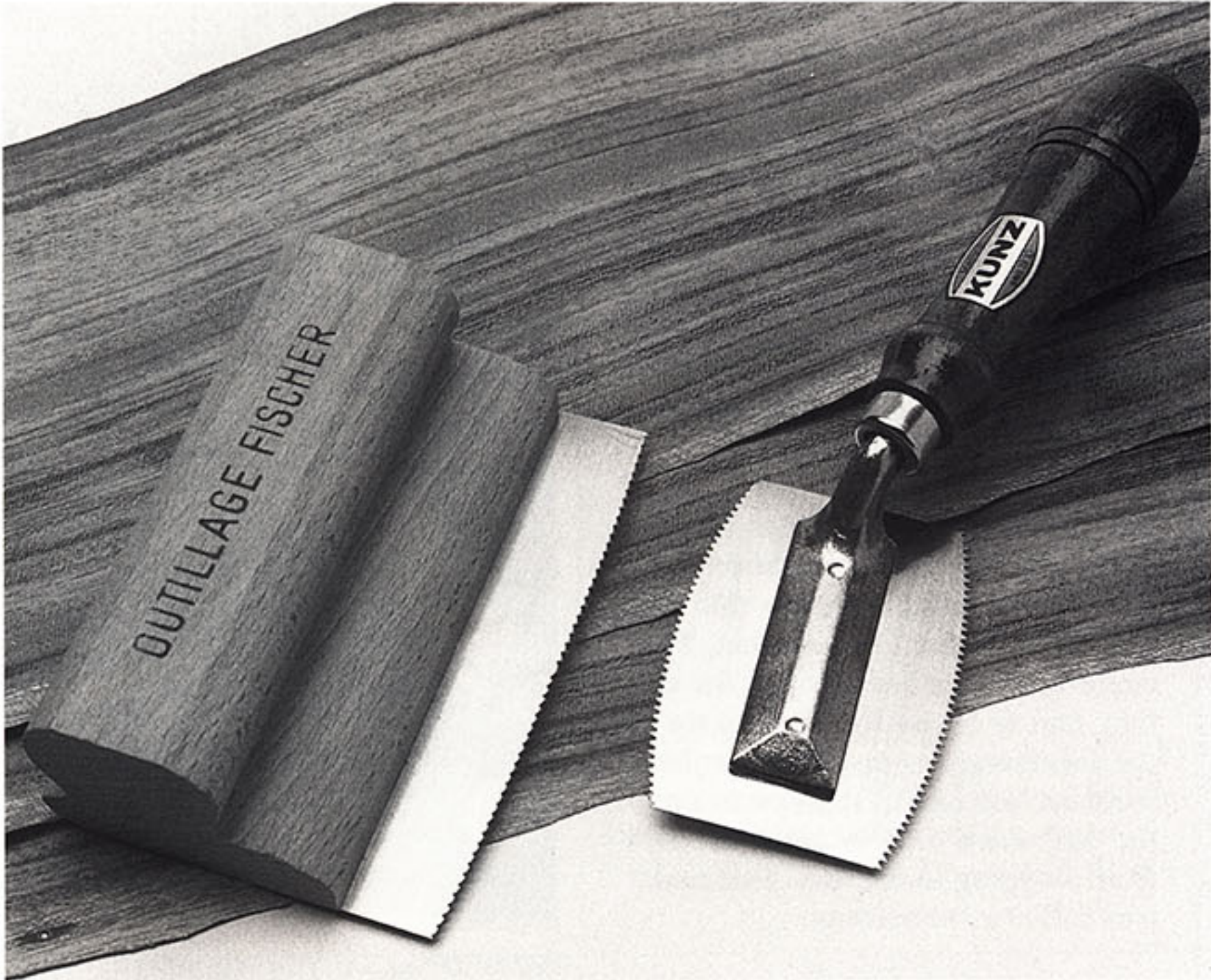
Two styles of veneer saws: at left, a French veneer saw; at right, a standard veneer saw. (Photo by Susan Kahn)
