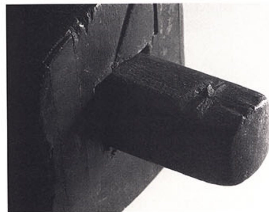
The stem of this old marking gauge has been scored by repeated filing of the marking pin.
