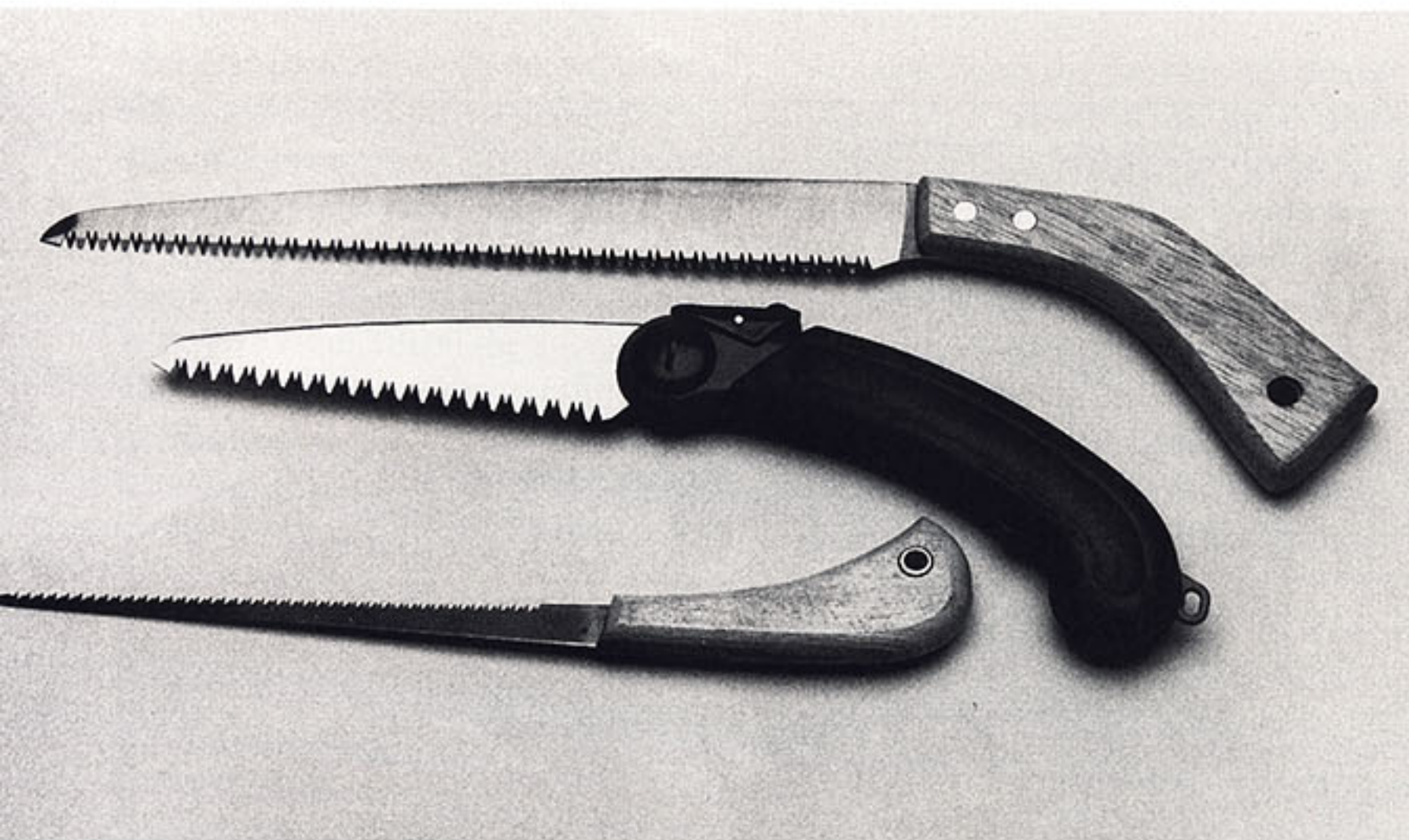
Two pruning saws and a keyhole saw. The saw at top, which has set teeth, is typical of Japanese pruning saws (though made in Taiwan). The middle saw, which has a tapered blade, is a top-of-the-line folding pruning saw made in Japan. The keyhole saw at bottom is just as effective in plasterboard as in wood. (Photo by Susan Kahn)
