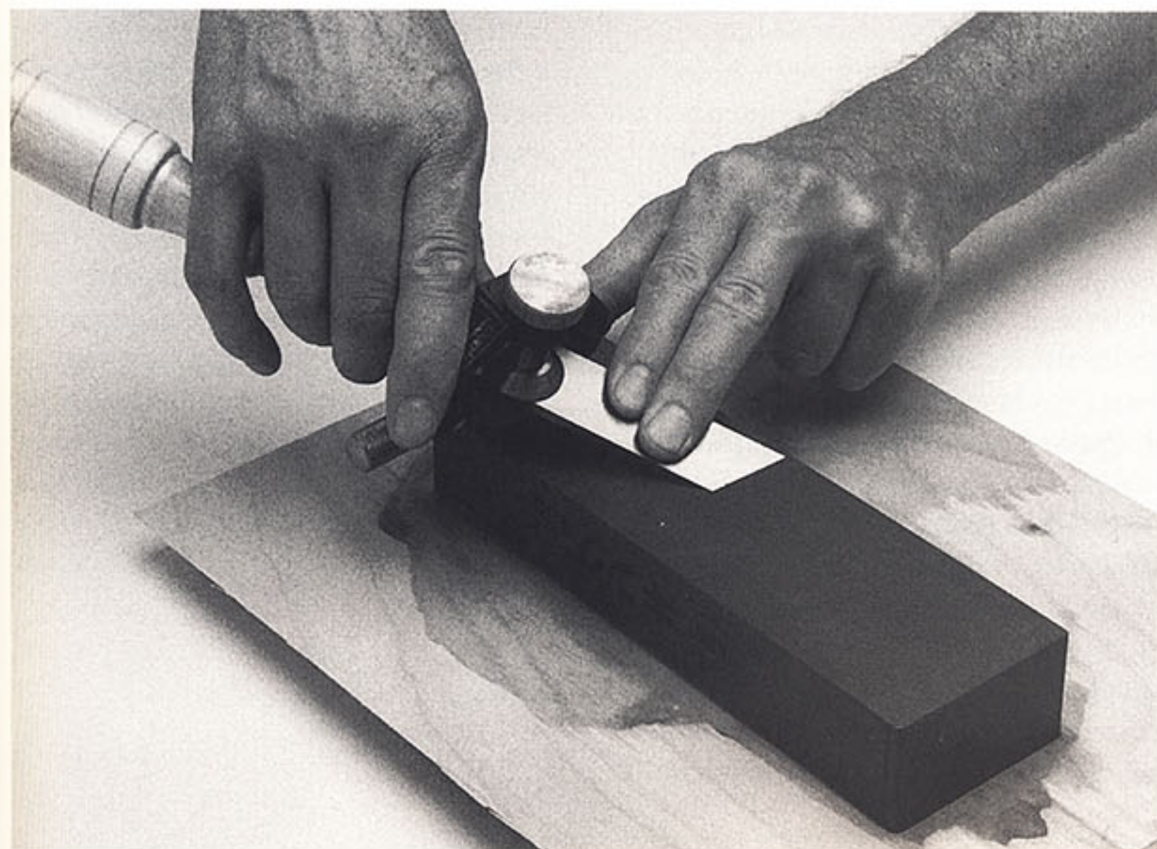
Skew chisels, available in left- and right-hand pairs, are specifically adapted to cutting end grain.
