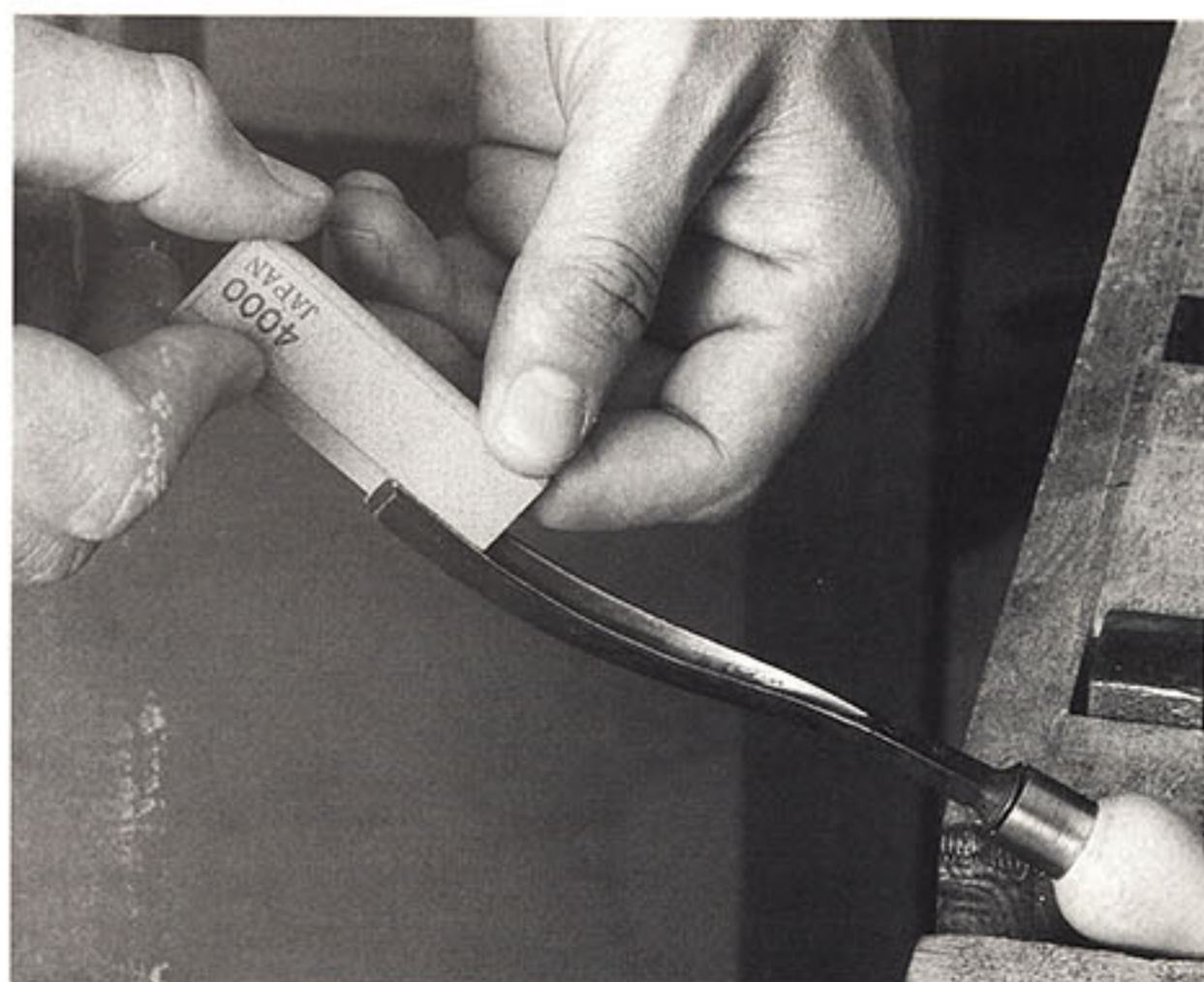
Alternatively, you can clamp the parting tool in a vise and use a slipstone on the inside.
