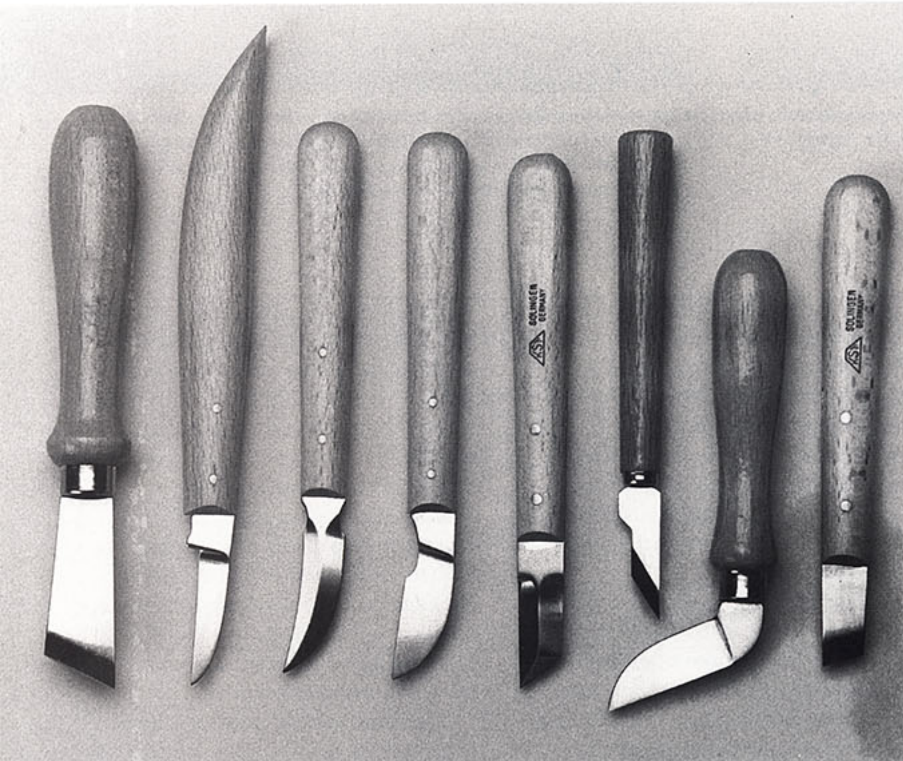
Chip knives are available in a wide range of styles. The knives second and third from left are more popular for carving in the round than for chip carving. (Photo by Susan Kahn)
