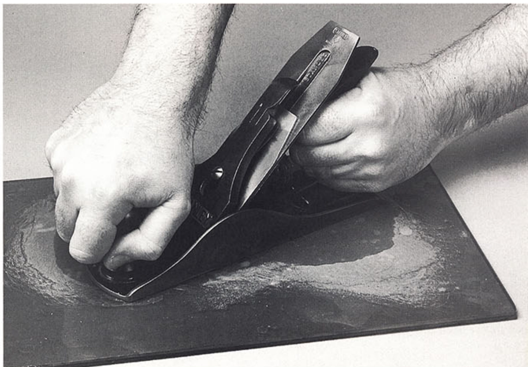
Moving the plane in a figure-eight or circular motion, lap the sole with silicon-carbide grit on a sheet of Mylar-faced plate glass.
