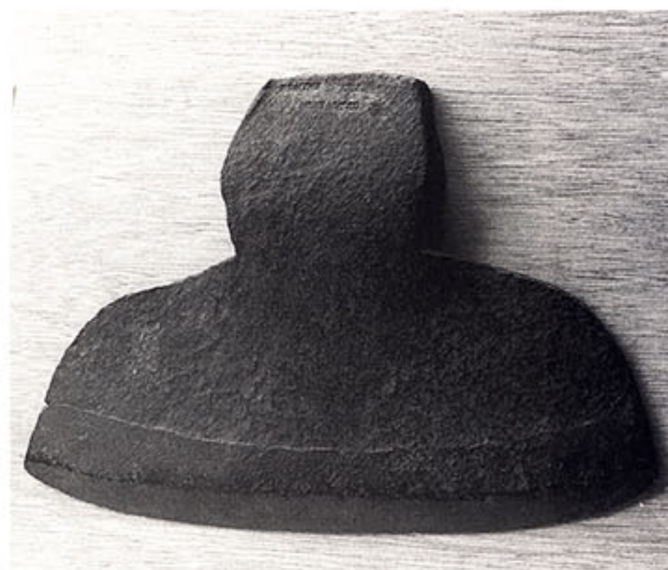
This classic old Canada pattern broad ax (made by Lyman Perkins, Hull, Quebec, sometime prior to 1834) shows rust pitting and a typical scarf weld.
