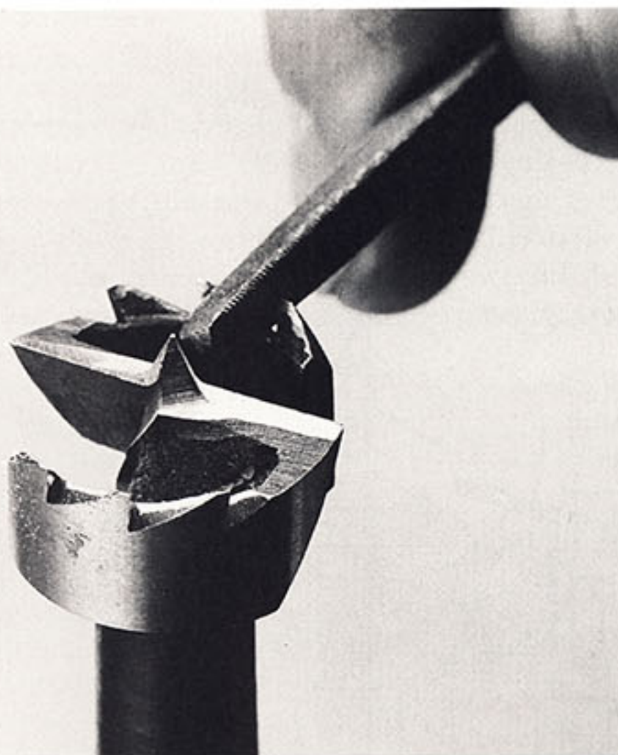
Sharpen the teeth of a sawtooth bit with a triangular file.
