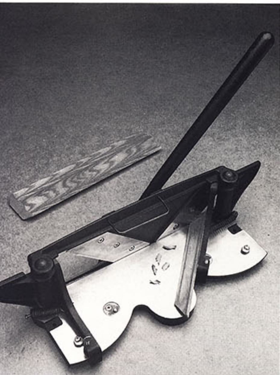
Miter trimmers are used only for trimming stock, usually taking off less than 1/8 in. per pass.
