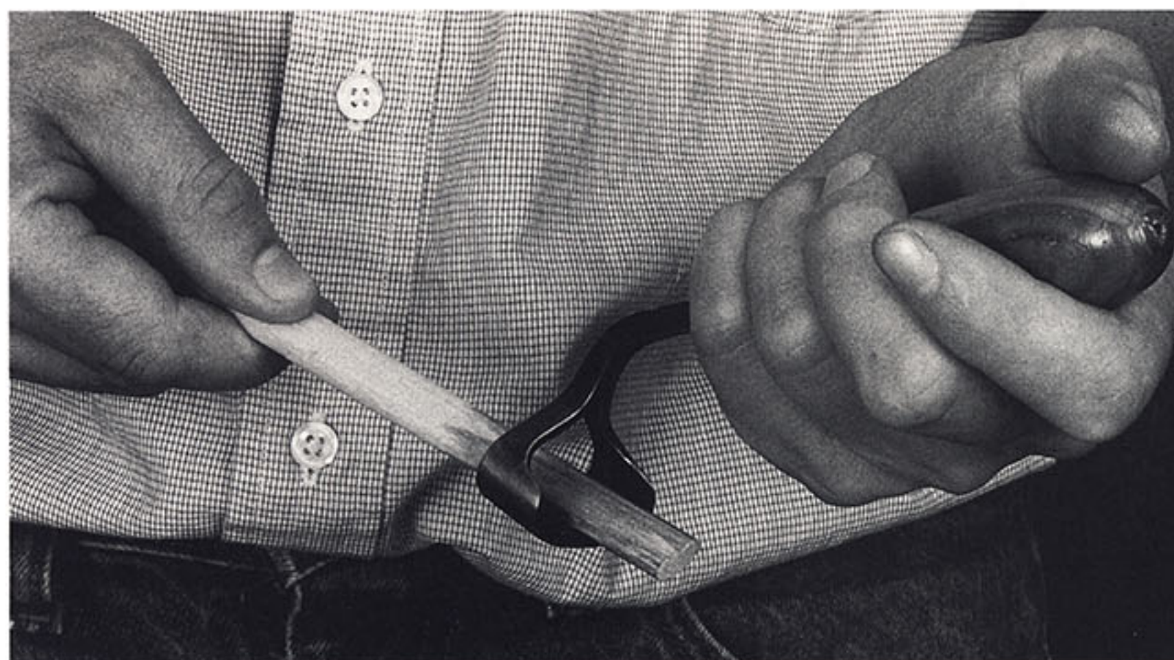
With the cutting edge of the tool facing away, use a chromium-oxide-charged wooden form to hone the inside of a scorp. Move the form much like a file, from the back inside of the scorp toward the edge. (Photo by Susan Kahn)
