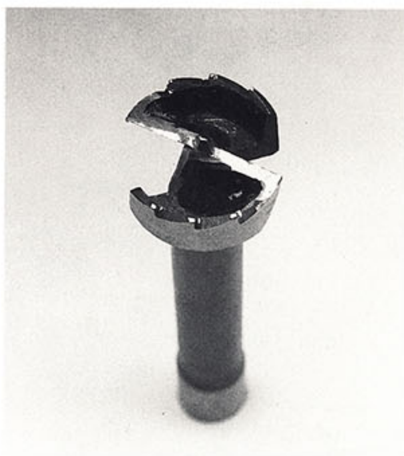
A sawtooth bit that has been jointed to make all teeth the same height.
