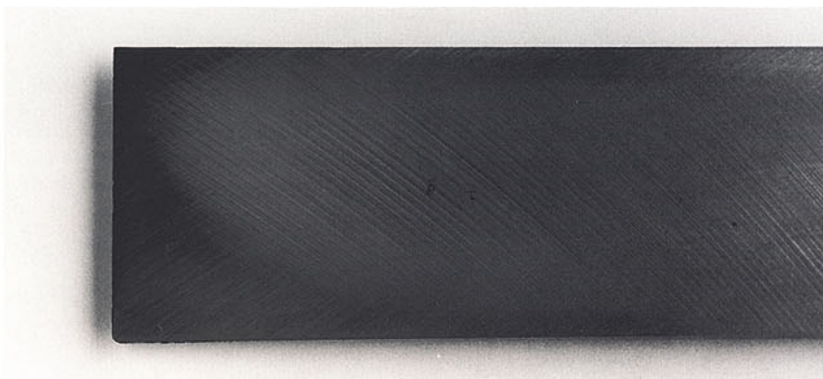
A chisel comes from the factory with grinding marks on its face (top). These marks must be removed to create a sharp edge and to flatten the face (above).
