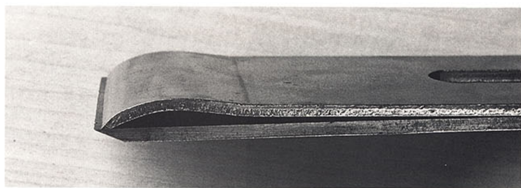
Dress the tip of the cap iron on a stone, with the opposite end of the iron held about \frac{1}{8} in. below the level of the stone.
