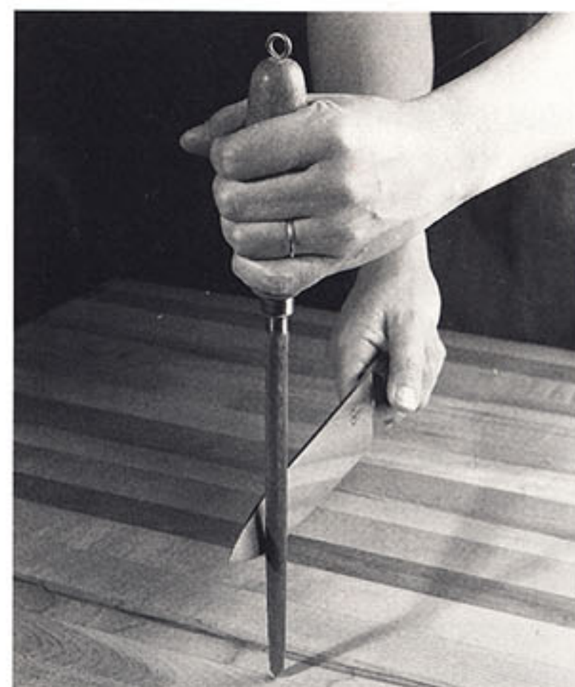
To use a knife steel, hold the steel vertically and take slicing cuts across it with the knife.
