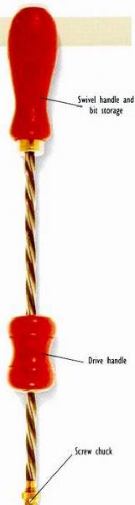
ABOVE: Archimedean drill, also called a fret drill, is used for boring small-diameter holes in thin-section wood.
