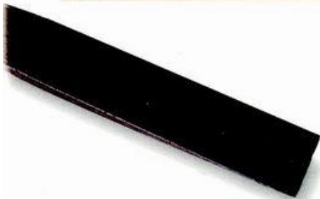
ABOVE: Flat-backed pattern maker's chisel
