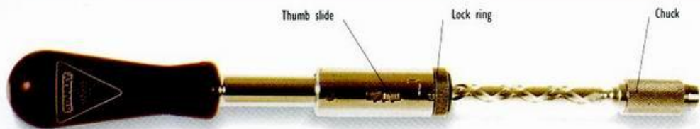
ABOVE: Yankee screwdriver – supplied with a selection of bits.
