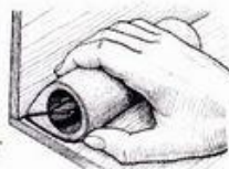
ABOVE: Using the tear-drop sander.
