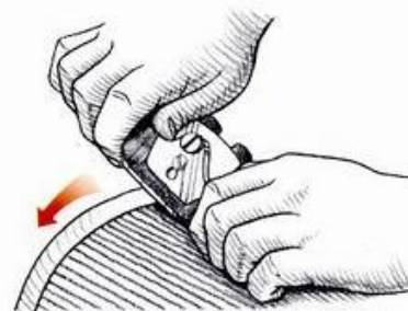
ABOVE: Following the grain downhill.
