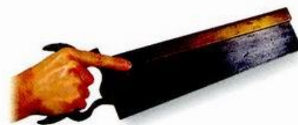
ABOVE: The handle of the dovetail saw is designed for maximum comfort. The notch at the top of the handle enables the woodworker to point and hook his index finger for optimum control.
