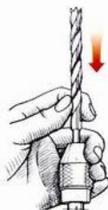
ABOVE: Putting the bit in the chuck.
