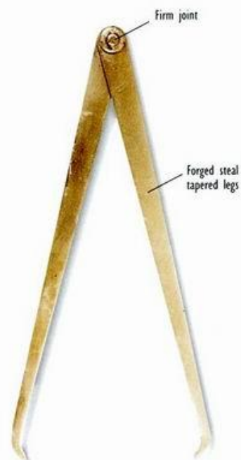
ABOVE: External firm joint calipers
