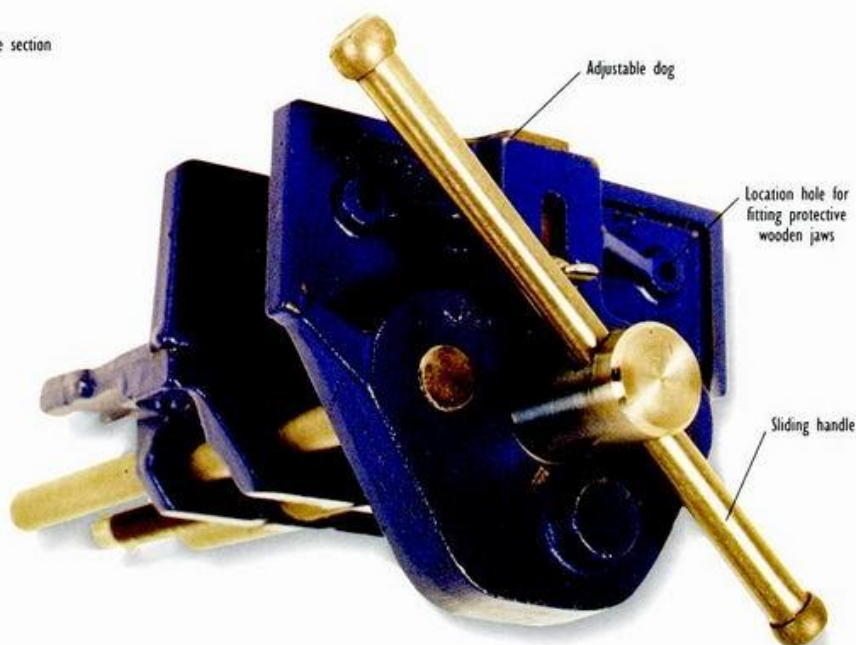
ABOVE: Plain screw vise with adjustable dog.
