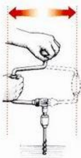
ABOVE: The sweep of the brace.
