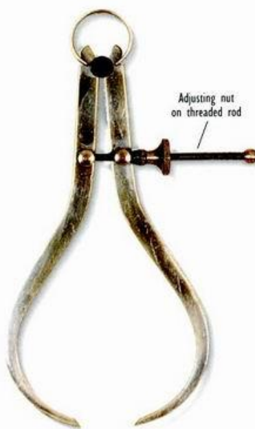
ABOVE: External bow spring calipers
