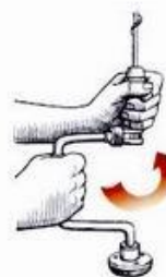
LEFT: To tighten up, hold the chuck and turn the brace.
