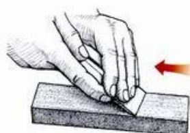
ABOVE: Honing the cutting edge.
