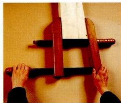
ABOVE: Clamping at an angle.
