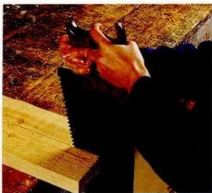
ABOVE: Overhand ripping on a bench
