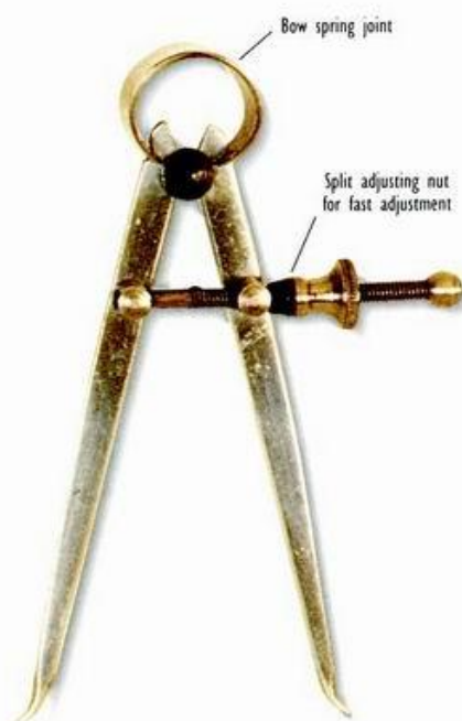
ABOVE: Internal spring bow calipers
