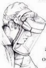
ABOVE: The powered anti-dust respirator.
