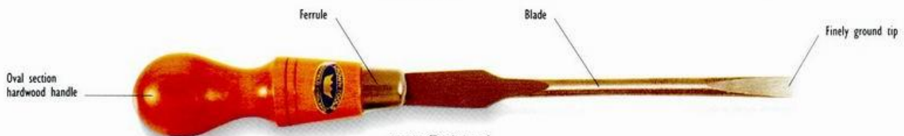
ABOVE: Traditional cabinet screwdriver
