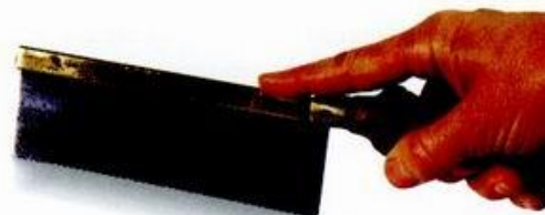
ABOVE: Extend the finger along the back of the saw to help guide the cut.
