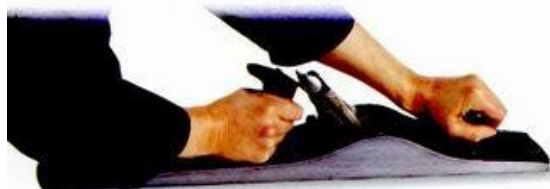
BELOW: Use both hands to achieve a well-balanced stroke.
