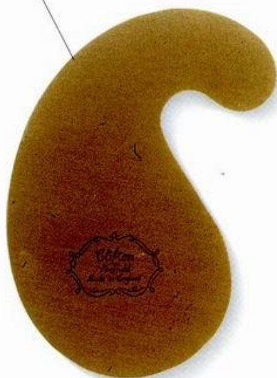
ABOVE: Scraper for shaped work.
