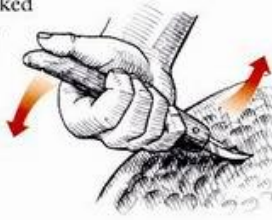
ABOVE: A crooked knife in action.
