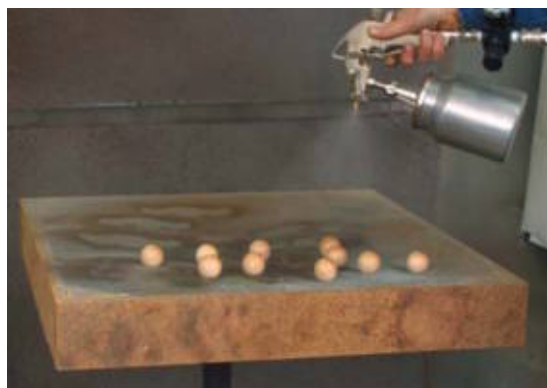
Spraying small wooden knobs on a screen box constructed with ½-in. wire mesh allows the air pressure to pass through so the parts don't blow around.
