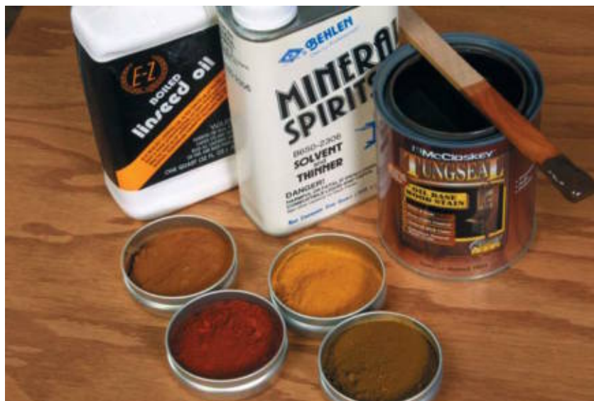
A typical oil-based wiping stain (right rear) consists of linseed oil (left rear) or alkyd binder, mineral spirits, and earth pigments (front).
