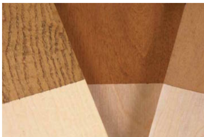
Pigment stains create contrast in ring-porous woods like ash (left). Diffuse-porous birch (center) colors more evenly, while dense maple (right) shows the least definition.
