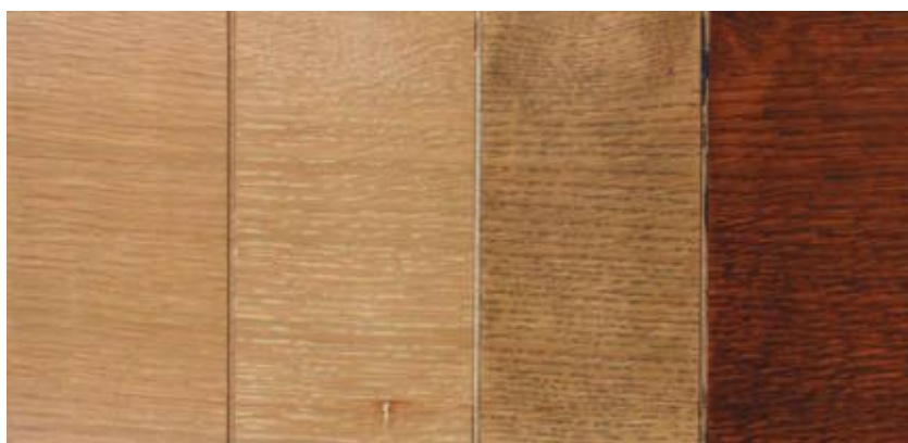
Water-based filler on white oak: from left, transparent filler; un-tinted neutral filler; dark brown filler; dark brown filler under alcohol dye stain.
