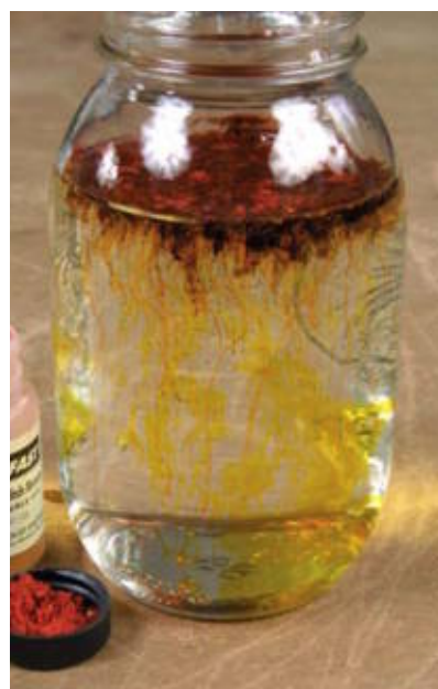
Dye powder placed in the proper solvent dissolves into a colored solution. This dissolving brown dye consists of red, yellow, blue, and black particles.
