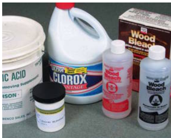
The three types of bleaches commonly used on wood are (from left) oxalic acid, chlorine (calcium hypochlorite, laundry chlorine bleach), and two-part wood bleach.
