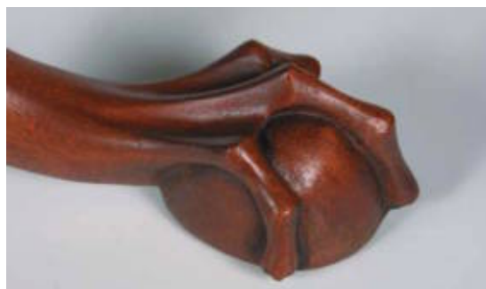
To retain the crispness of carvings, such as on this ball-and-claw mahogany foot, the author applied two light coats of shellac with an artist's brush, followed by a gentle rubbing with 0000 steel wool.
