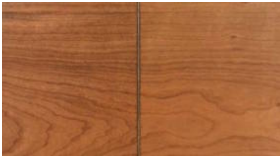
The intensity of a glaze is primarily controlled by how the wood surface is sealed. The left side of this cherry panel has one coat of sealer, and the right side has two.
