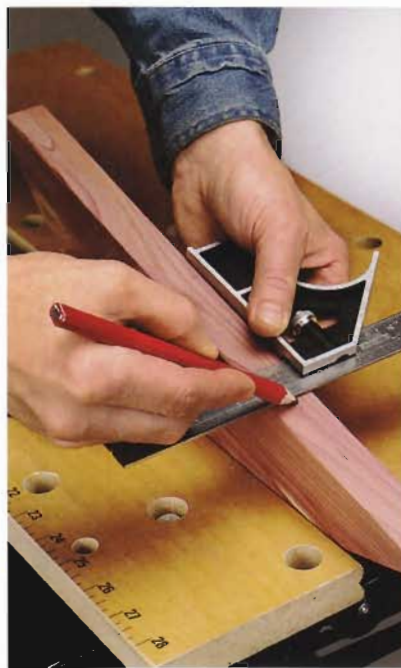
B. Use a combination square to make straight, accurate reference marks.
