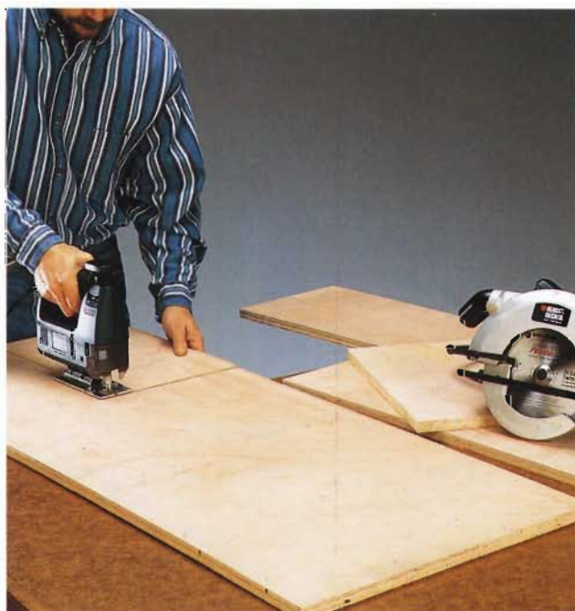
A. Cut along the straight cutting lines on the side panels with a circular saw, then use a jig saw or hand saw to finish the cuts at the corners.
