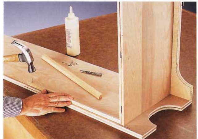
C. Attach the back braces to the sides, creating a \frac{1}{4} " recess for the back panel.
