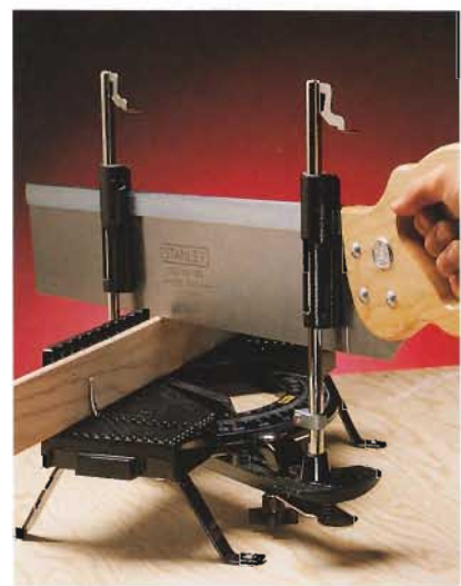
Make angled cuts in decorative trim moldings with a hand miter box to add a stylish flair to your project.
