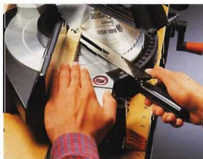
A. Duplicate the slope of the staircase with a T-bevel and a level and transfer the angle directly to a power miter saw or a miter box with a hand saw.
