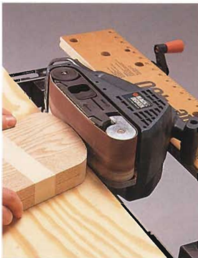
Clamp a belt sander and a scrap board to the workbench to create a stationary shaping tool.
