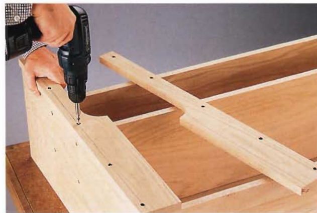
C. Fasten the legs to the front edges of the end panels. Make sure the outside edges of the legs overhang the end panels by \frac{1}{4} ".
