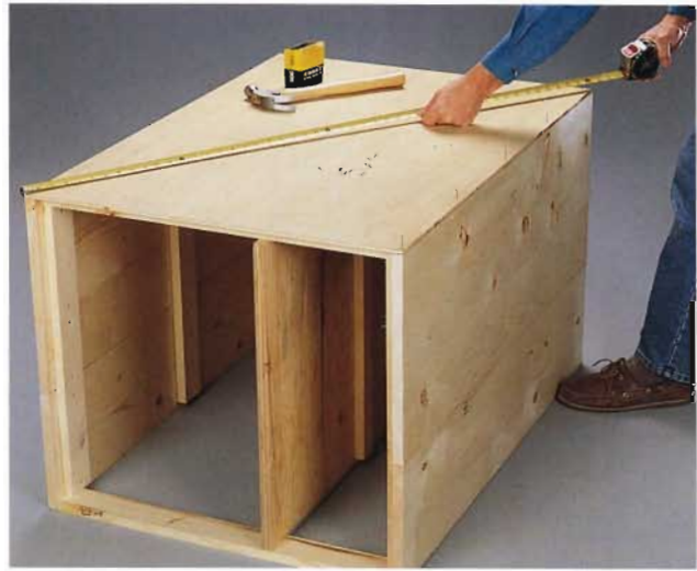
D. Check for square by measuring diagonally between the corners to make sure the distances are equal.
