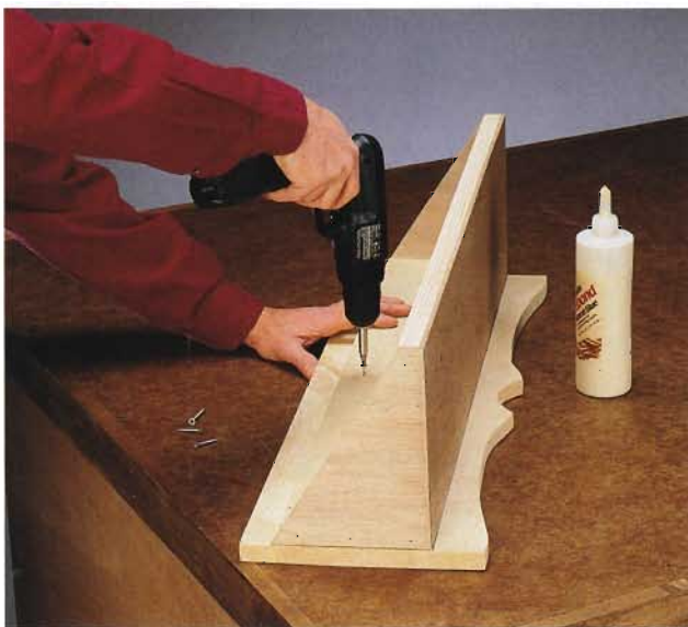
D. Drive wood screws through the inside of the bin and into the back of the false front.
