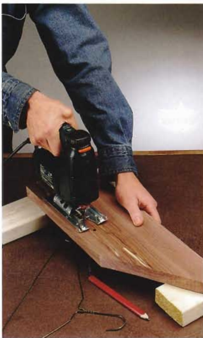
A. Cut the aromatic cedar with even pressure applied to the saw, or your cuts will be rough and more difficult to sand.
