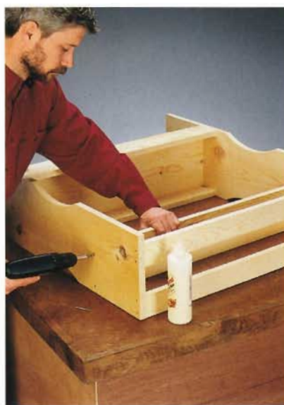
B. Fasten the bin stop board between the end panels to complete the assembly of the framework.
