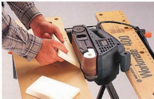
C. Clamp a belt sander to your worksurface, and use it as a grinder to shape bevels into the front edges of the tops.
