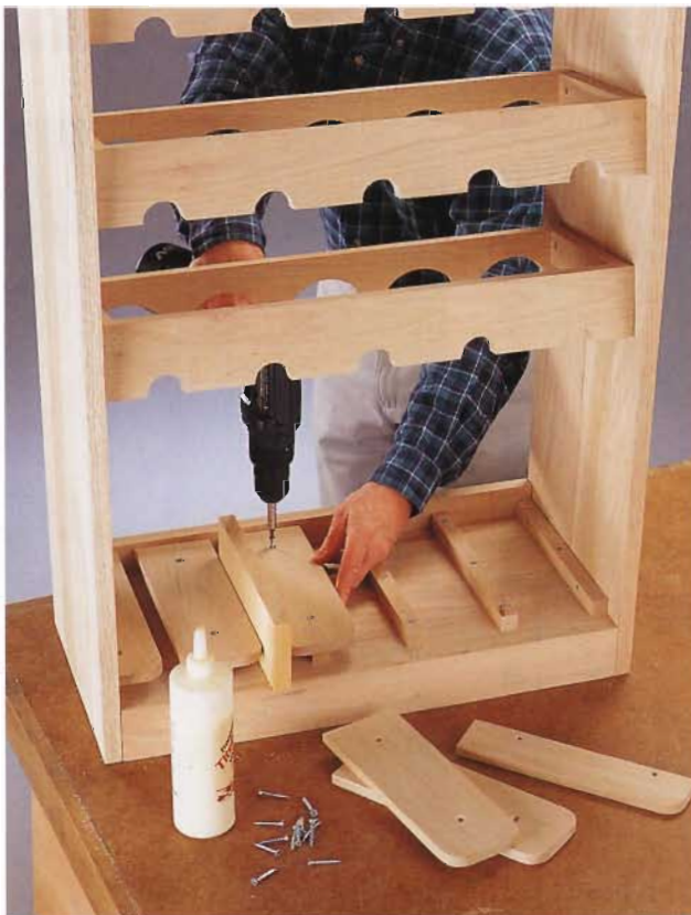
F. Use a \frac{1}{4} " spacer to guide the placement of the stemware plates.
