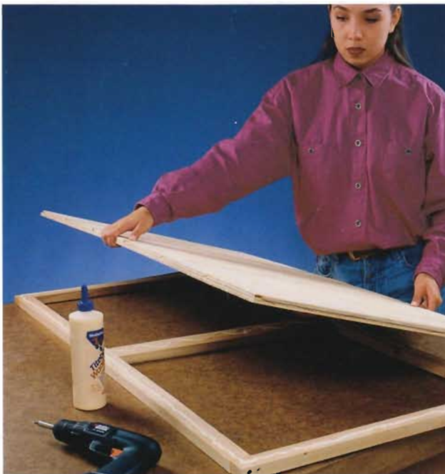
A. Cut and fasten the lid to the framework with the grooves in the panel running from back to front.
