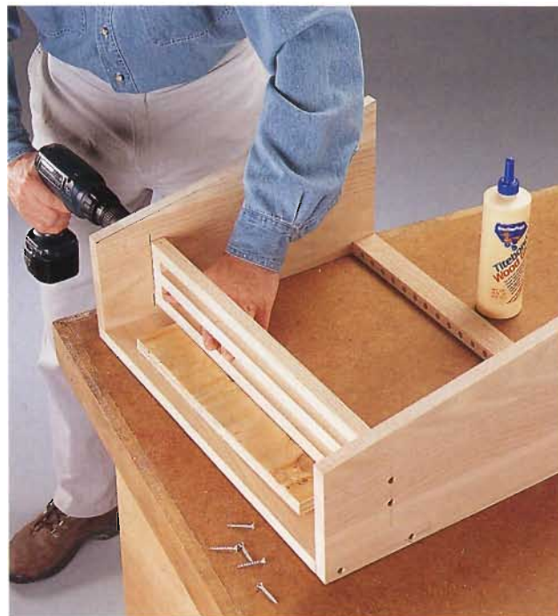
B. Use a \frac{3}{4} " spacer to position the shelf from the back while you drill counterbored pilot holes.
