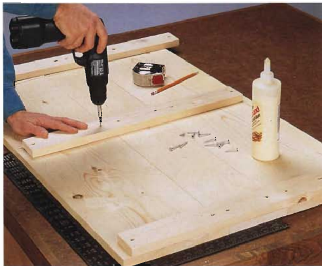
A. Fasten cleats to the side and middle boards, forming the cabinet sides.
