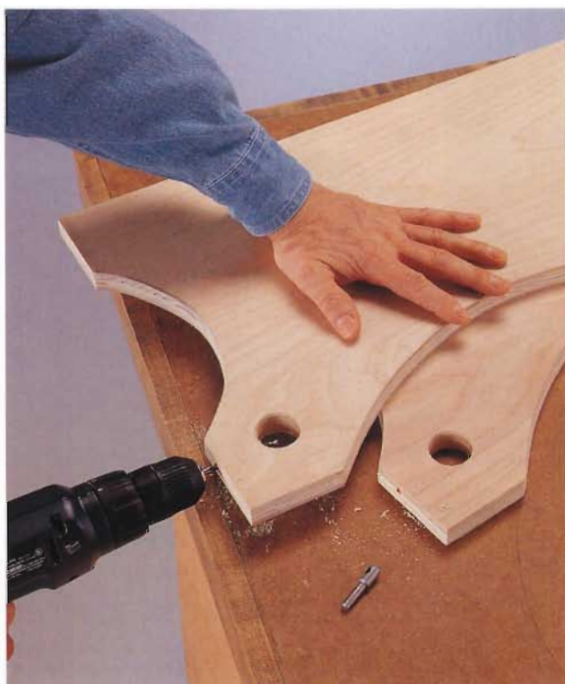
A. Drill pilot holes for the anchor screws through the bottom edges and into the dowel holes.
