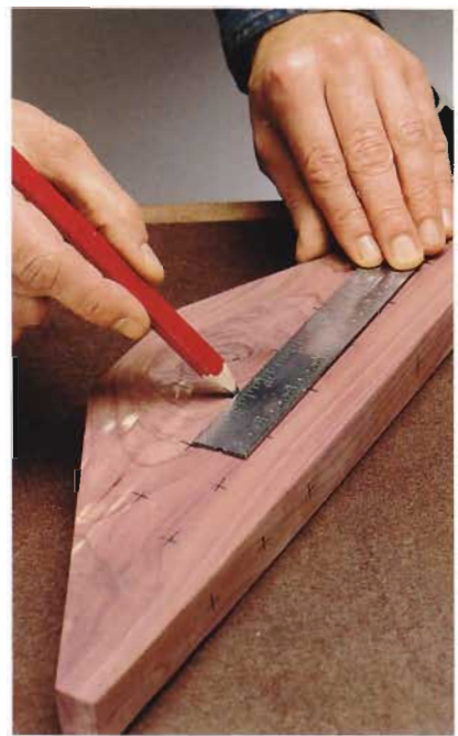
C. Offset the reference marks in the second tier of tie hooks by measuring out ¼" from the center mark.
