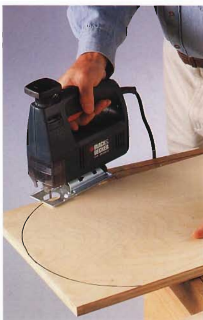
A. Use a jig saw to cut the 7\frac{1}{2} "-radius curves on the tops of the side panels.
