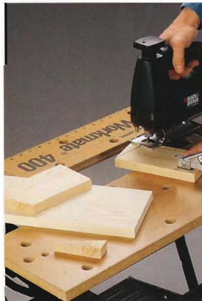
E. Draw angled cutting lines onto the box sides, then cut along the lines with a jig saw.
