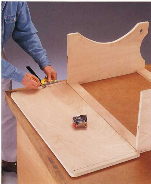
C. Draw reference lines on the top to use for positioning when attaching the top to the sides.
