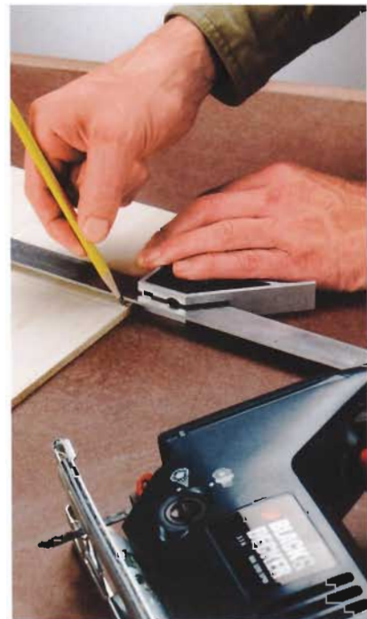
C. Mark and cut out the ¼" notches in the dividers.
