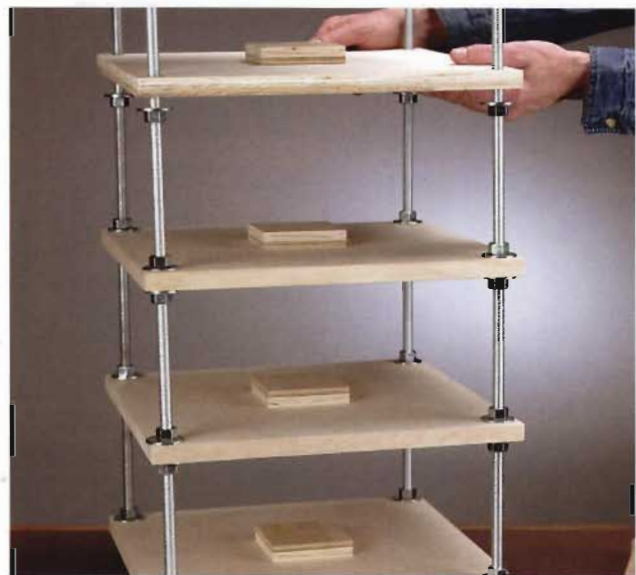
E. Slide the shelves down to rest on the washers below. Be careful not to chip the veneer surfaces.
