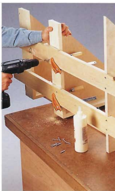
B. Drive screws through the standards and into the shelf rails.
