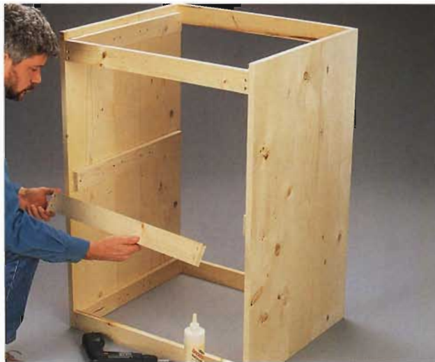
B. Attach front and back stretchers at the top and bottom, and a middle stretcher at the back.
