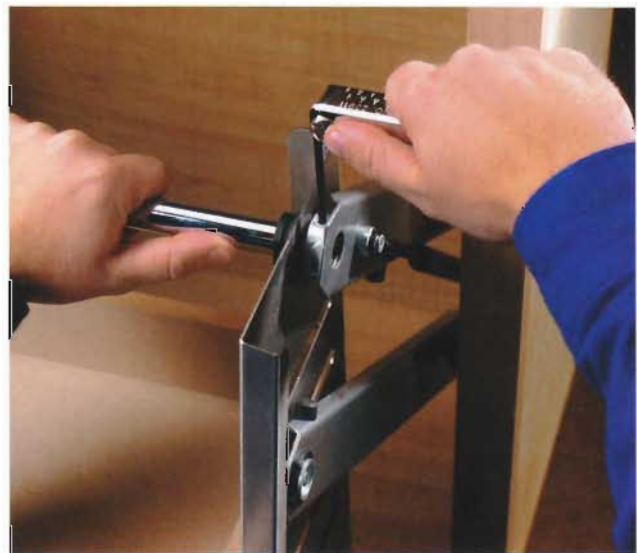
D. With the assistance of a helper, secure the shelf unit to the swing arms.
