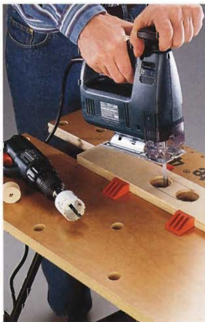
B. Make the ends of the handle cutout in the divider with a hole saw, then connect with a jig saw.
