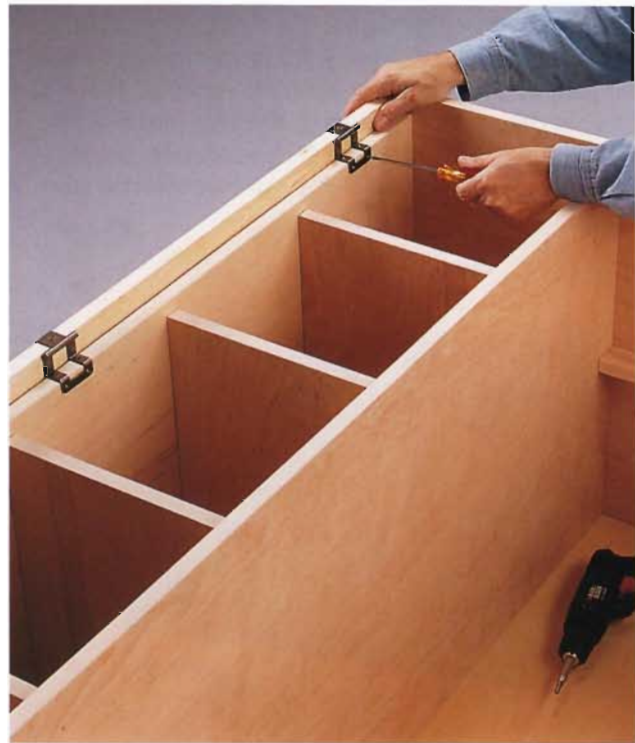
H. Position the doors and fasten the hinges to the side panels.
