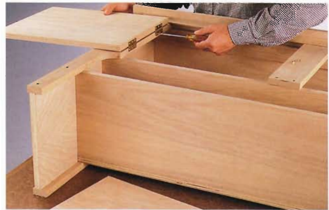
F. Attach each door to a leg, using 1\frac{1}{2} \times 3 " butt hinges.
