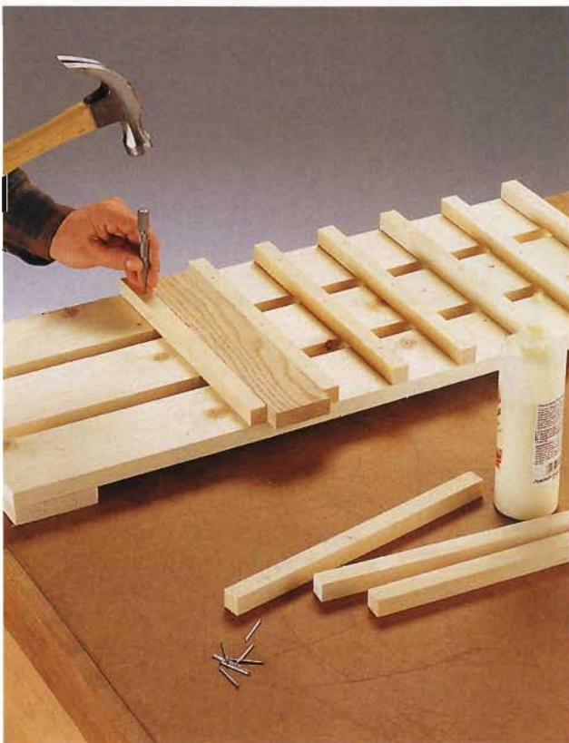
F. A 2\frac{1}{2} "-wide spacer helps ensure uniform placement of the wine shelf cleats.
