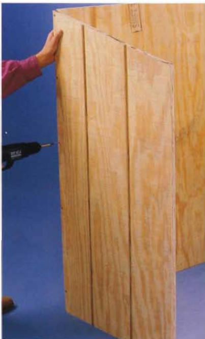
C. Attach the end panels to the back panel, keeping the back panel flush with the back edges of the end panels.
