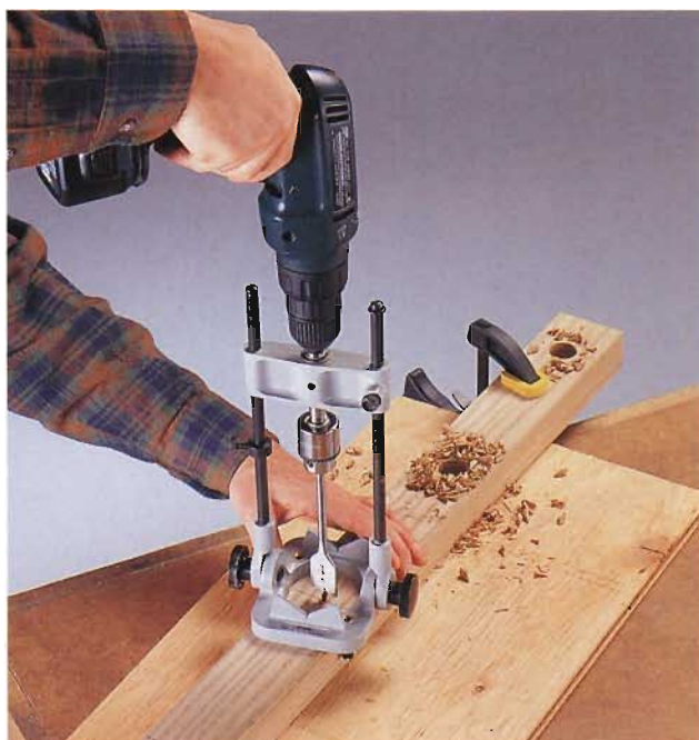
A. Place a scrap of plywood under the stretchers to prevent tearouts, and drill 1" holes in each stretcher.
