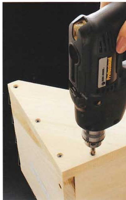
D. Position the backer board over the workpiece, aligning the edges, and drive screws through countersunk pilot holes, starting with the hole closest to the center.
