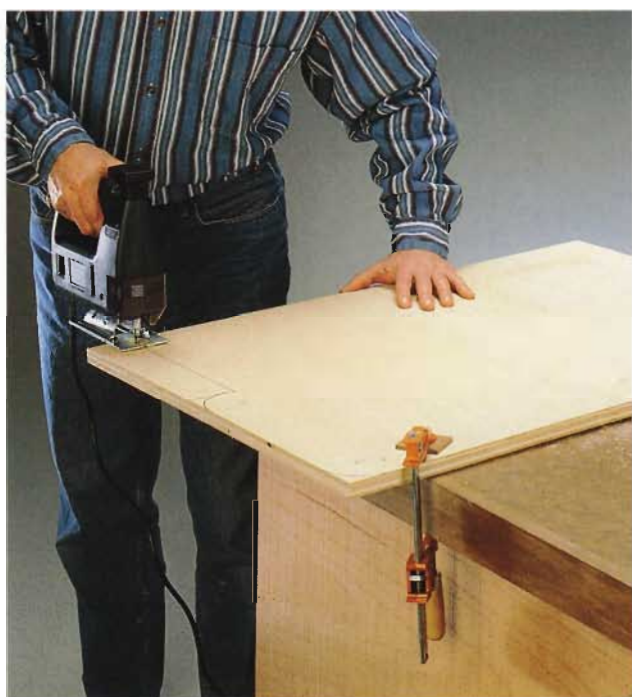
E. Use a jig saw to cut notches into the sides of the worksurface so it fits around the side panels.
