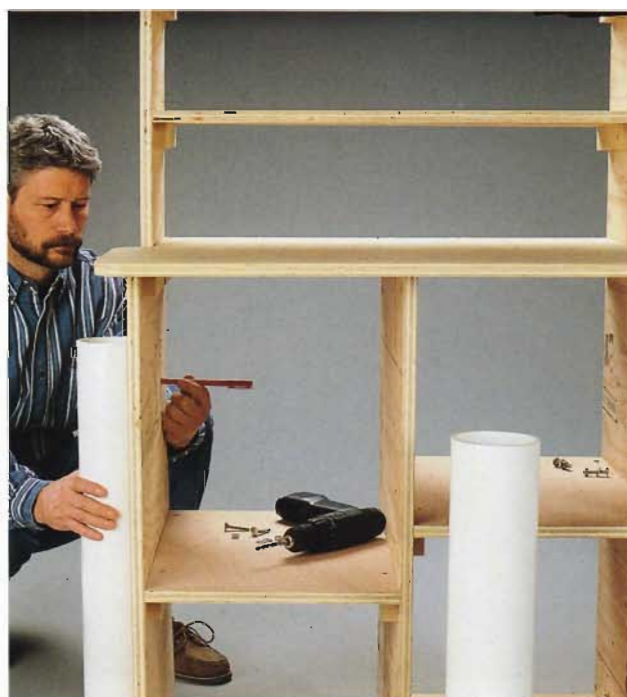
F. Insert a pen or pencil into the guide holes in each side panel and mark drilling points on the pipes.
