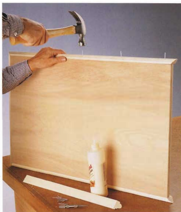
E. Attach the top cap around the perimeter of the lid. Drive nails in partially before positioning the strips.
