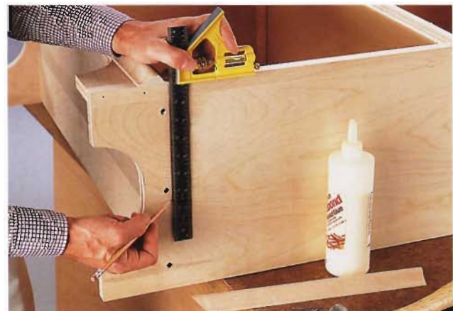
F. Using a combination square, draw lines on the sides, aligned with the top of the bottom facing.
