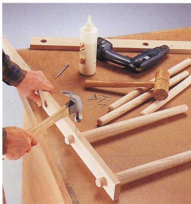
B. Insert the dowels into the holes, securing each with glue and a 4d finish nail driven through a pilot hole.
