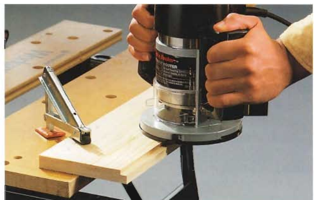
Rabbet grooves are routed into the edge of a panel and are used to join two panels into a 90° corner.
