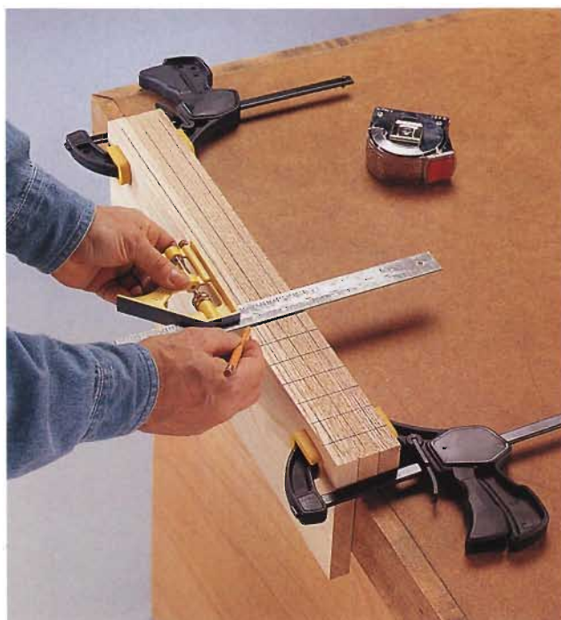
A. Clamp the back and the rails together, then measure and mark the dowel locations.
