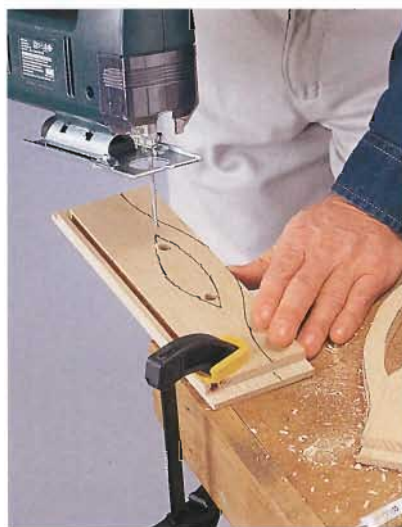
Make contoured internal cutouts by drilling starter holes and cutting along the lines with a jig saw.
