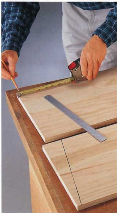
C. Measure \frac{1}{2} " along the front and 2\frac{1}{2} " along the back of each side, and connect the marks for the bottom rack alignment.
