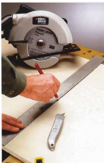
A. Lay out the block pieces. Score all crosscuts with a utility knife, then cut out the pieces.
