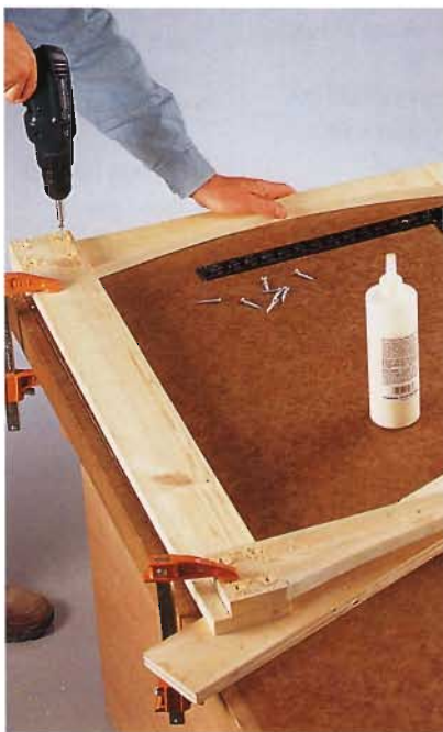
D. Assemble the arched front rails and the stiles into face frames.
