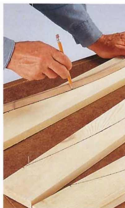
C. Use a flexible marking guide to draw the arches on the front rails.
