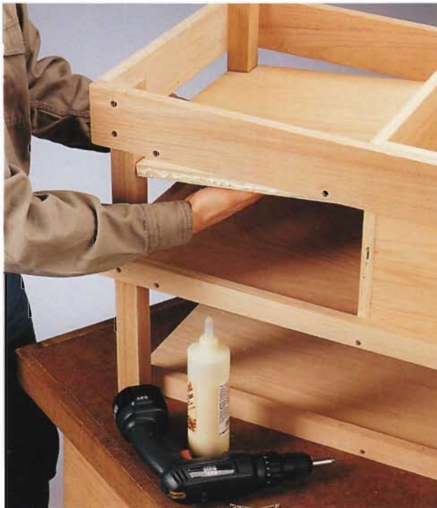
H. Glue the bin bottom between the credenza sides, flush with their bottom edges, and secure it with screws.
