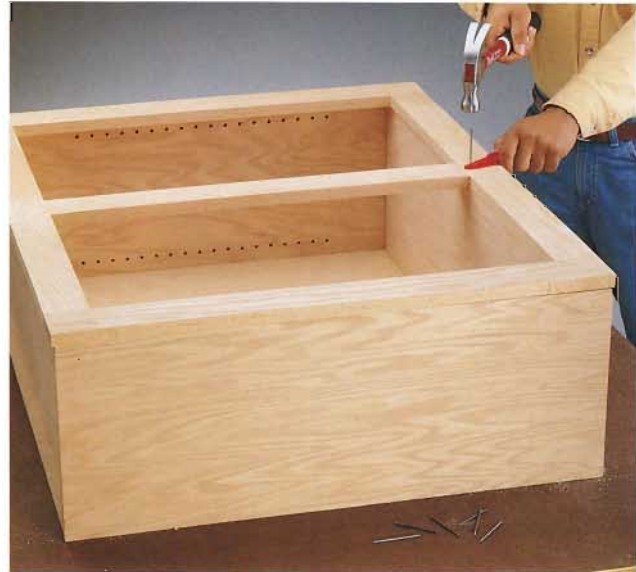
E. Center the face frame on the cabinet and attach it with glue and 2" finish nails.
