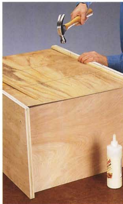
B. Attach cleats made from \frac{1}{2} " quarter-round molding at the outside edges of the back panel to give it extra strength.
