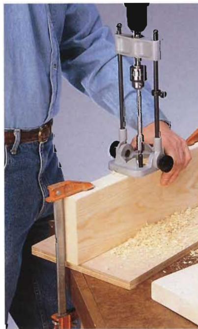
D. Drill a 1"-dia. hole through the handles, using a piece of scrap as a backing board.
