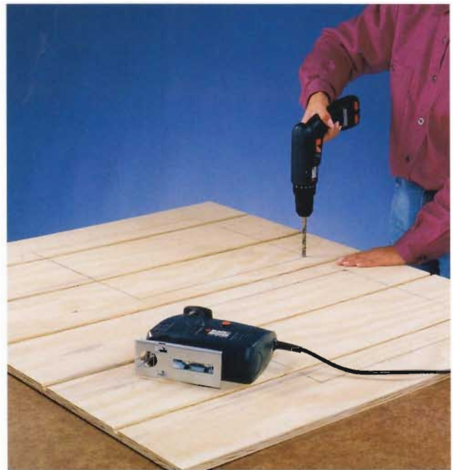
B. Drill a ⅝"-dia. starter hole at a corner of each door opening and cut out the opening.
