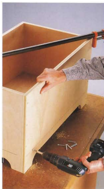
C. Hold opposite chest corners together with a bar or pipe clamp to keep the chest square.
