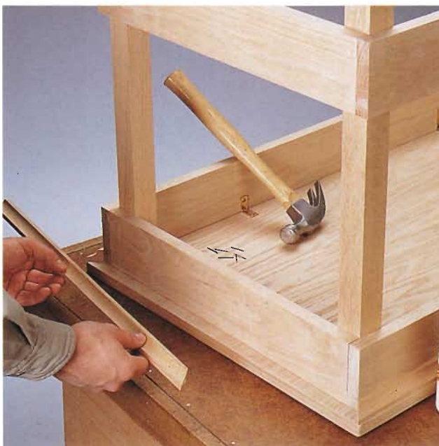
D. Install strips of oak cove molding along the underside of the desktop.
