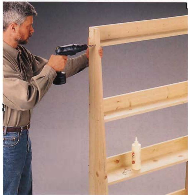
D. Attach the shelves, driving wood screws through the standards and into the ends of the shelves.
