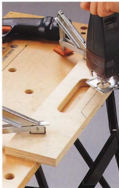
E. Cut access notches and finger-grip cutouts into the front and back of the tray.
