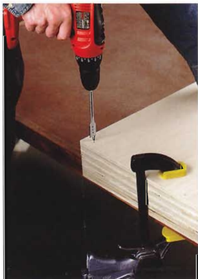
A. Clamp the shelves and a backer board together, with their edges flush. Drill a hole at each reference mark.
