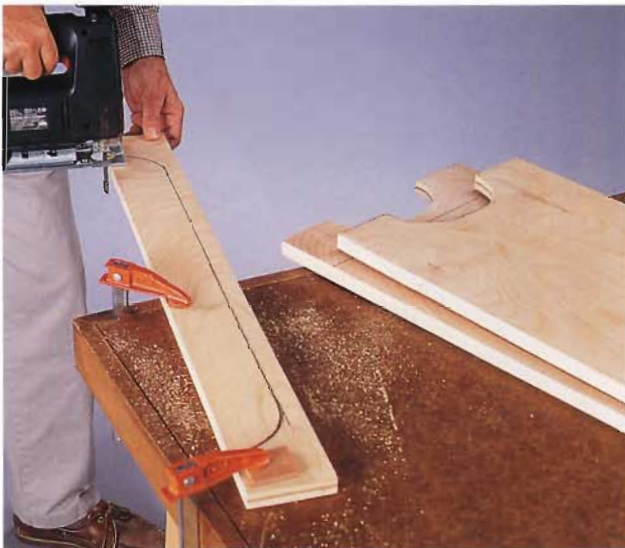
A. Cut arches along the bottoms of the side panels and front rail to create the bookcase "feet."
