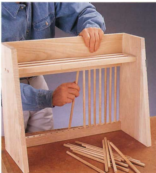
C. Insert dowels into the holes under the back first, then drop them down into the holes in the rail.
