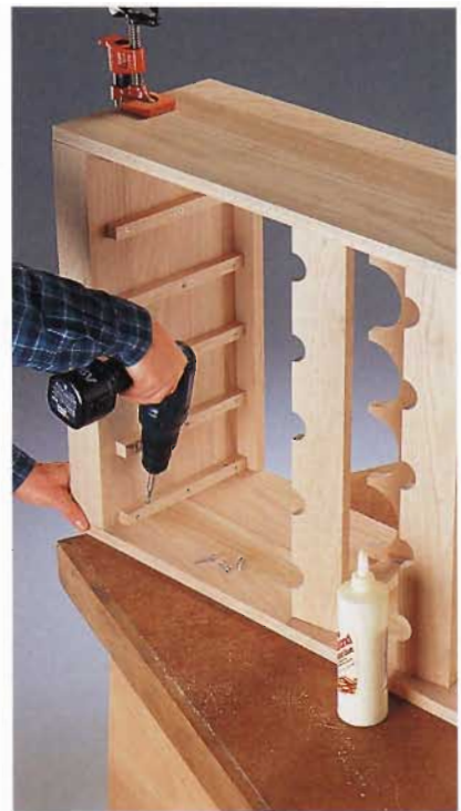
E. Drive screws through the slats to secure the top to the sides.
