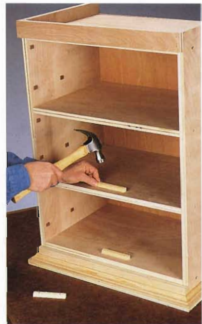
F. Turn the frame upside down, and use 1" brads to attach the stop blocks.
