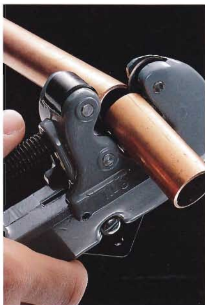
A. Position the tubing cutter, and score a line around the pipe. Rotate the cutter around the pipe until it separates.
