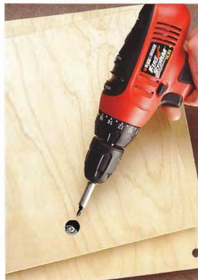
C. Fasten the lazy Susan to the base panel. Drill a hole in the bottom of the base to access the mounting holes inside the revolving ring.
