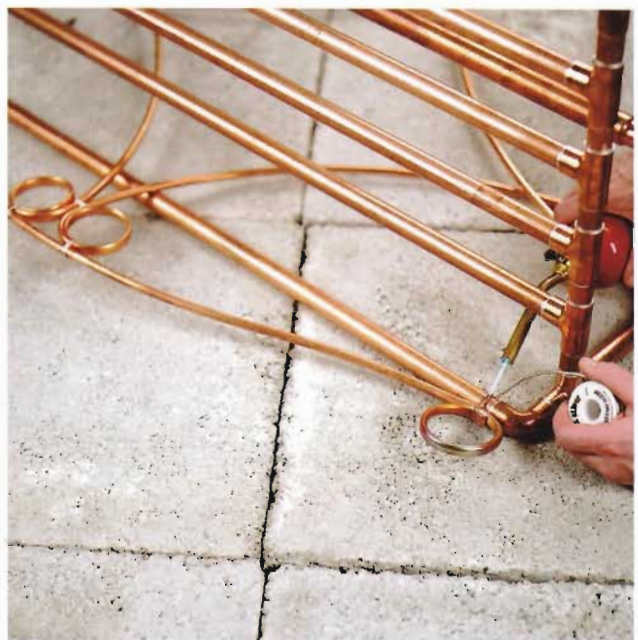
D. Solder the decorations to the rigid frame at the designated locations, centering them on the rack. Tap each soldering area with a hammer prior to soldering the joint to create a flatter area for adhering the solder.
