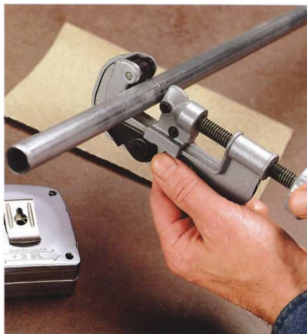
B. Tighten the cutting wheel to the conduit and turn the pipe cutter over the top of the pipe, tightening the cutter every few rotations.
