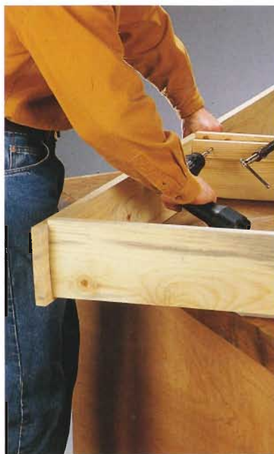
B. Clamp the lid supports in position flush with the top of the box in front and back, then fasten them with wood glue and screws.
