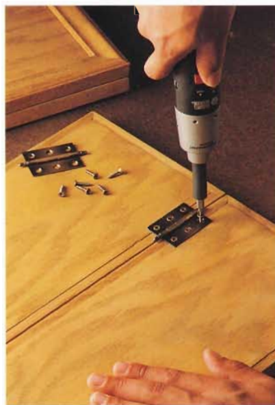
N. Build folding overlay doors for the center unit. Join each pair with butt hinges attached to backs of panels.
