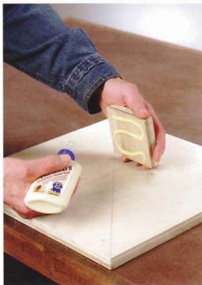
B. Install the divider squares, using wood glue and 1\frac{1}{4} " brads.
