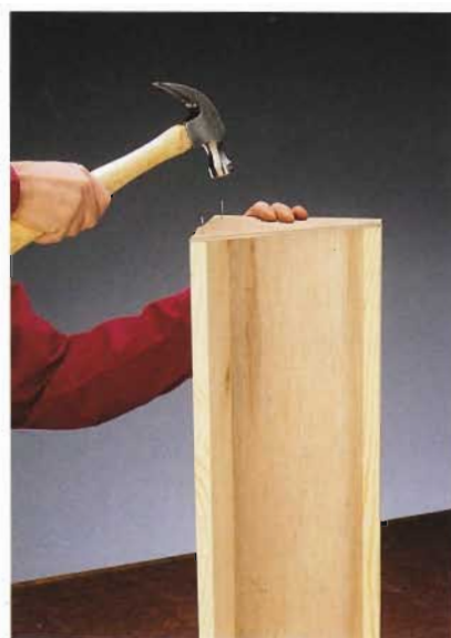
C. Fasten the bin sides with glue and wire nails.
