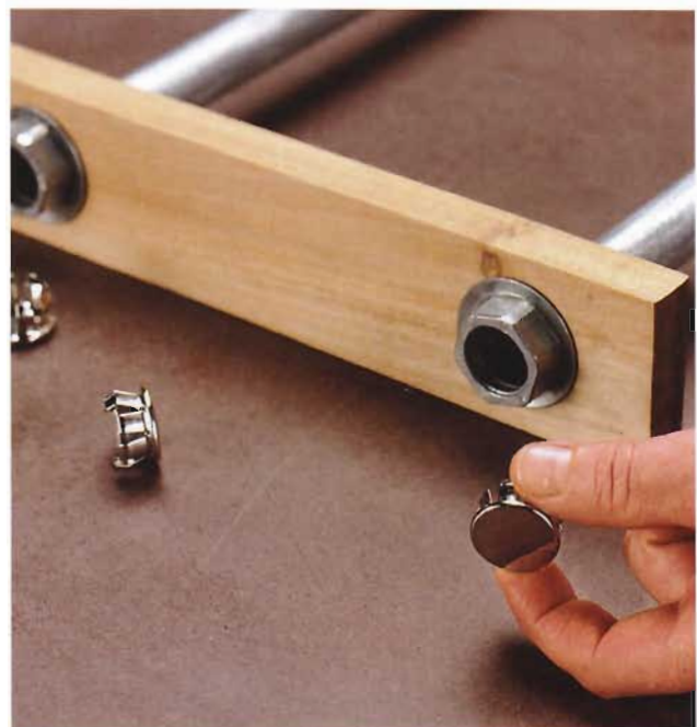
C. Finish the rack by plugging the holes in the compression fittings with 1" chrome-plated furniture caps.
