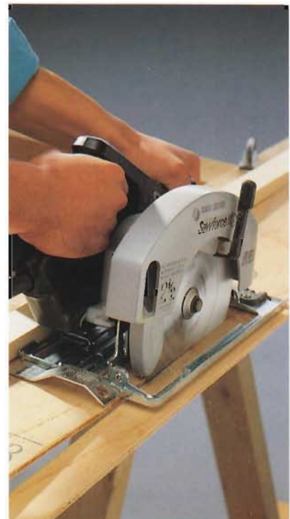
C. Cut off the excess using a circular saw, router, or jig saw.
