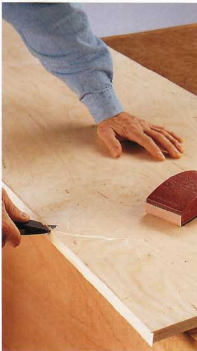
A. Apply veneer edge tape to the exposed plywood edges. Trim off excess tape with a sharp utility knife.
