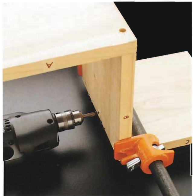
B. Clamp each new shelf to the workpiece so that the new shelf is flush against the work surface.
