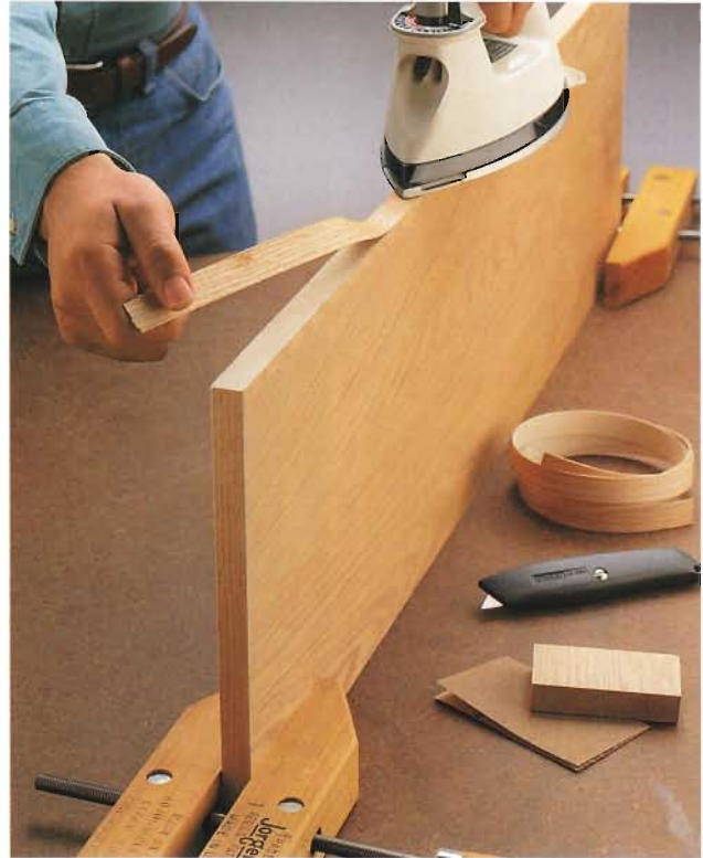
Use heat-activated veneer tape to cover unfinished edges of plywood or particleboard panels. Bond the tape with a household iron, then rub it with a block of hardwood, and trim the edges with a utility knife. Lightly sand the edges to smooth them.
