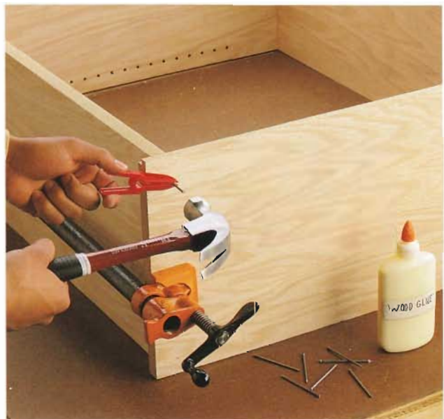
C. Reinforce each dado joint with 2" finish nails driven every 3".
