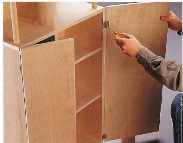
D. Hang the doors, using brass butt hinges.
