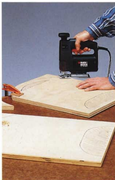
A. Make the handle cutouts and the curves at the top and bottom of the end panels with a jig saw.
