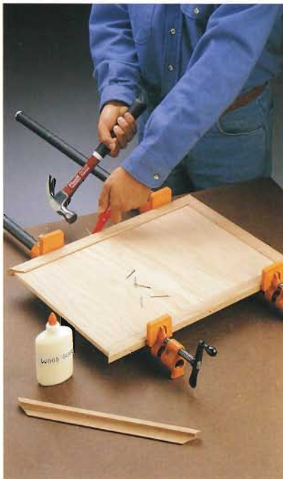
A. Attach the door-edge molding to the door panel by driving 1 1/2" finish nails through pilot holes.
