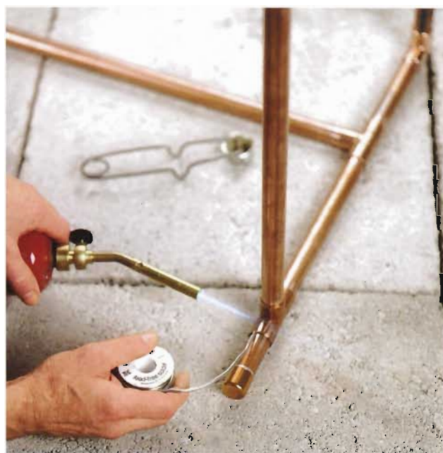
B. Solder the joints of the frame from the base up. Solder the upper shelf assembly separately to make the assembly process easier.
