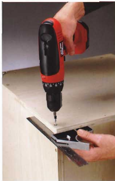
C. Drive in a corner screw, making sure the block is square before driving each additional corner screw.
