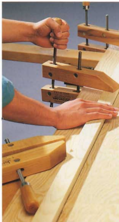
B. Fasten the cleat to the plywood with glue, and clamp the cleat every 12".
