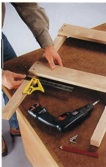
A. Check with a combination square to make sure the desk legs are square to the ends.
