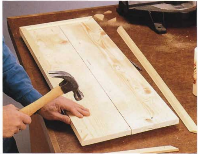
I. Attach pine stop molding to create a frame around the edges of the door boards.
