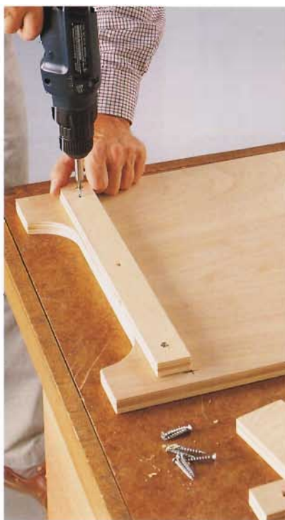
B. Center the end cleats over the kick spaces, leaving \frac{3}{4} " at each end where the side cleats will fit.
