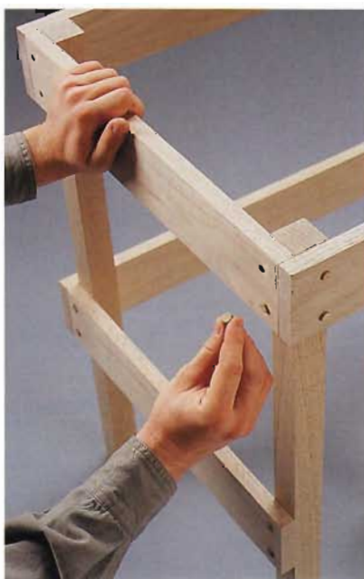
B. Glue oak plugs into the screw holes to cover the screws.
