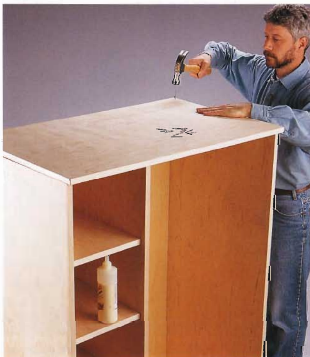
F. Fasten the top panel with glue and 6d finish nails.
