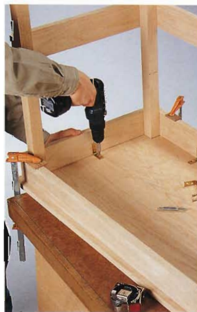
C. Fasten the desktop to the desk base with brass corner braces.
