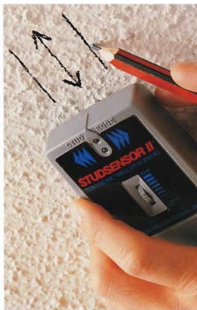
A. Locate the existing wall studs and ceiling joists. Mark the direction and edges of each joist with a pencil.
