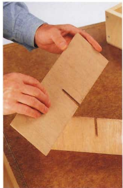
F. Cut out the tray dividers, then notch them to form half-lap joints. Test-fit them, then glue the dividers in place.
