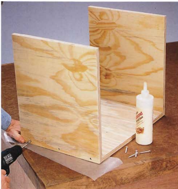
A. Attach the sides to the back, using glue and counterbored #6 \times 2" wood screws.
