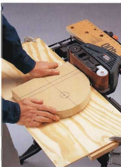
A. Use a belt sander clamped on its side to the work surface to gang-sand the end pieces.
