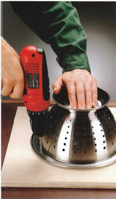
A. Drill the holes in \frac{1}{4} increments of the perimeter of the colanders.
