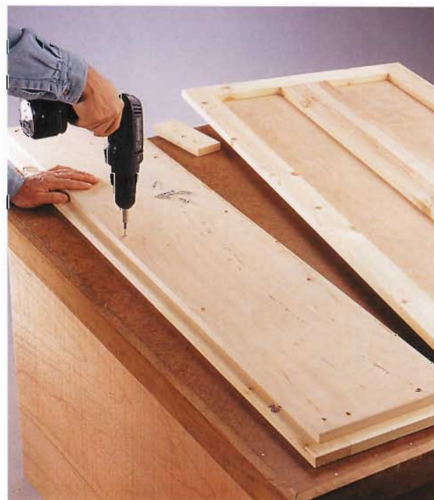
G. Attach the rails and stiles to the door panels with glue. Drive 3d finish nails through the frames into the panels.
