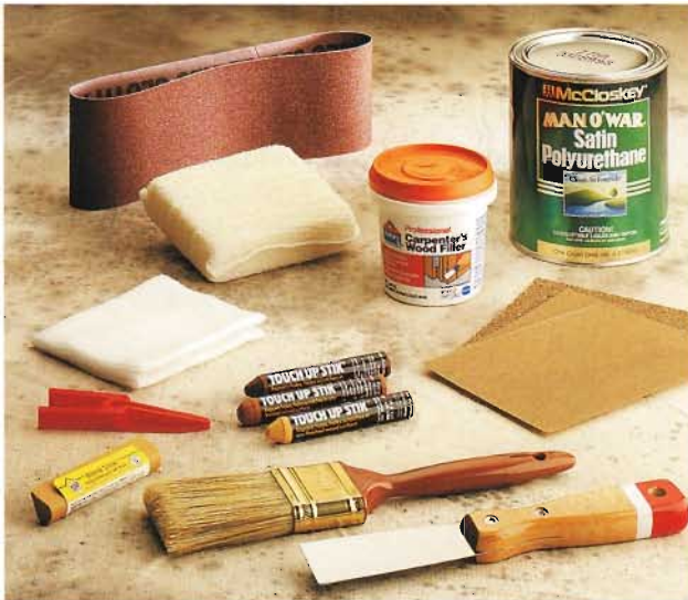
Specialty tools and materials for finishing work include: 120-grit sanding belt, staining pad, untinted wood filler, clear polyurethane, tack cloth, finish-nail holder, tinted filler sticks, paintbrush with blended bristles, putty knife, and sandpaper in 80-, 120-, and 220-grit sheets.
