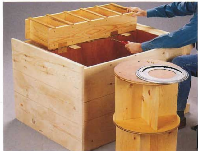
J. With spacers in place to help align the parts, attach the swing-out rack to the divider with 3 x 3" butt hinges.
