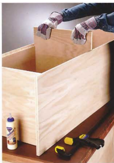
B. Assemble the cabinet frame with glue in each joint and clamp the joints tight. Make sure the front edges of the panels are flush.
