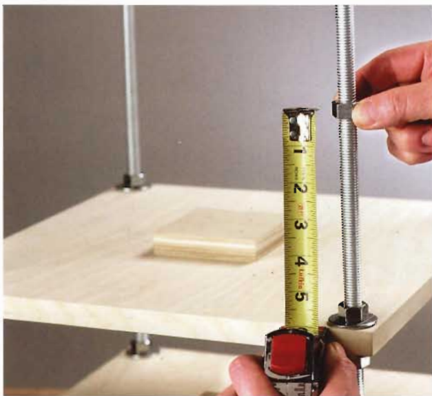
D. Position each set of hex nuts 6" above the previous shelf.
