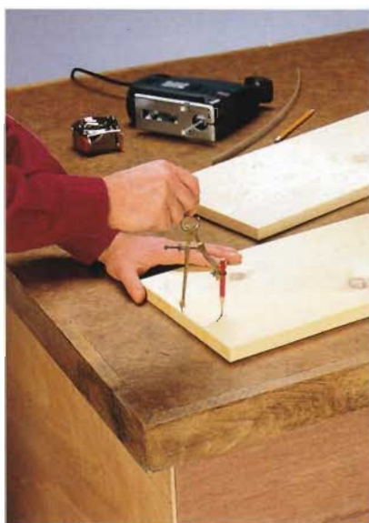
A. Use a compass to draw 2 \frac{1}{4} "-radius semicircles on the bottoms of the end pieces.
