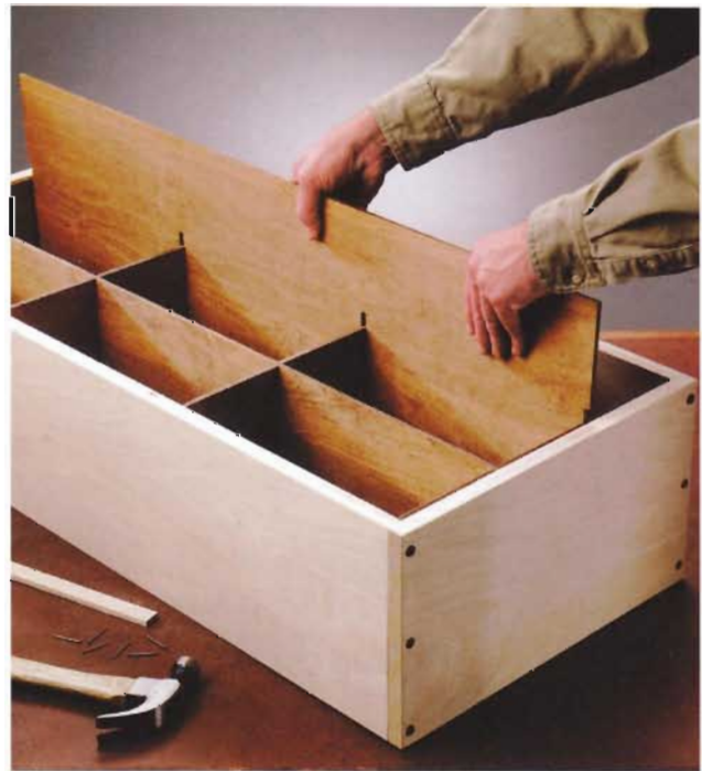
E. Slide the completed dividers into the box and install the stile and rail trim around the front edge.
