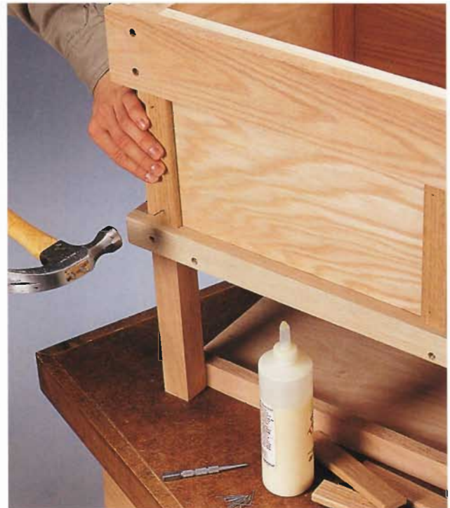
I. Attach strips of oak molding to cover the exposed plywood edges on the outside of the credenza.
