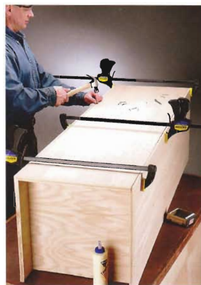
C. Attach the back panel with glue and 6d finish nails. Countersink the nail heads with a nail set.
