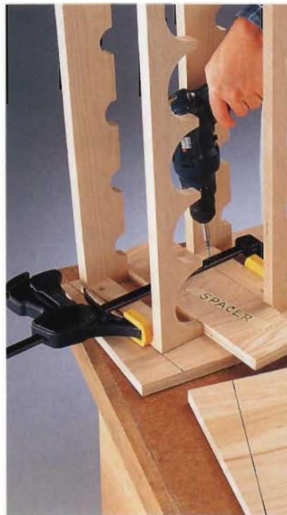
D. Clamp a 4 \times 10 " spacer between the top and middle racks for proper positioning.
