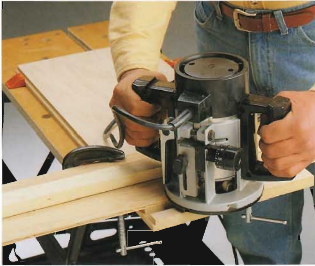
A. Measure and cut the \frac{3}{4} " plywood side panels to size. Then rout the rabbets and dados, using a router and a straightedge guide.
