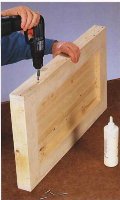
D. Attach the end and side frames to the cover panel assembly with glue and counterbored screws.
