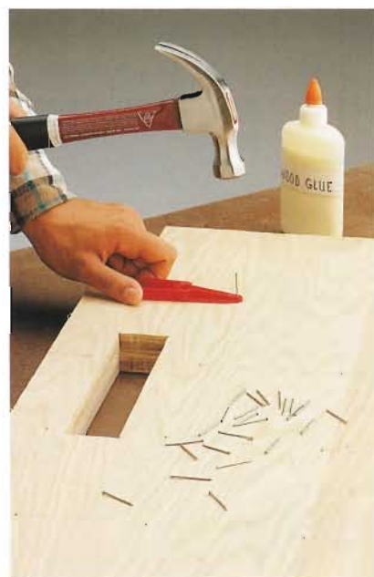
D. Join two of the notched permanent shelves together with glue and \frac{1}{4} " finish nails to form one double-layer shelf.
