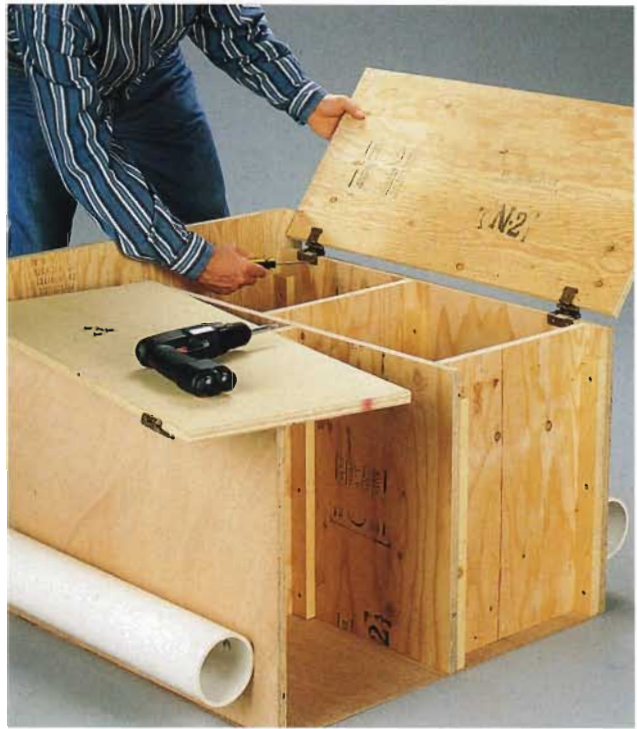
G. Hang the cabinet doors with self-closing cabinet hinges to keep the doors from swinging open.
