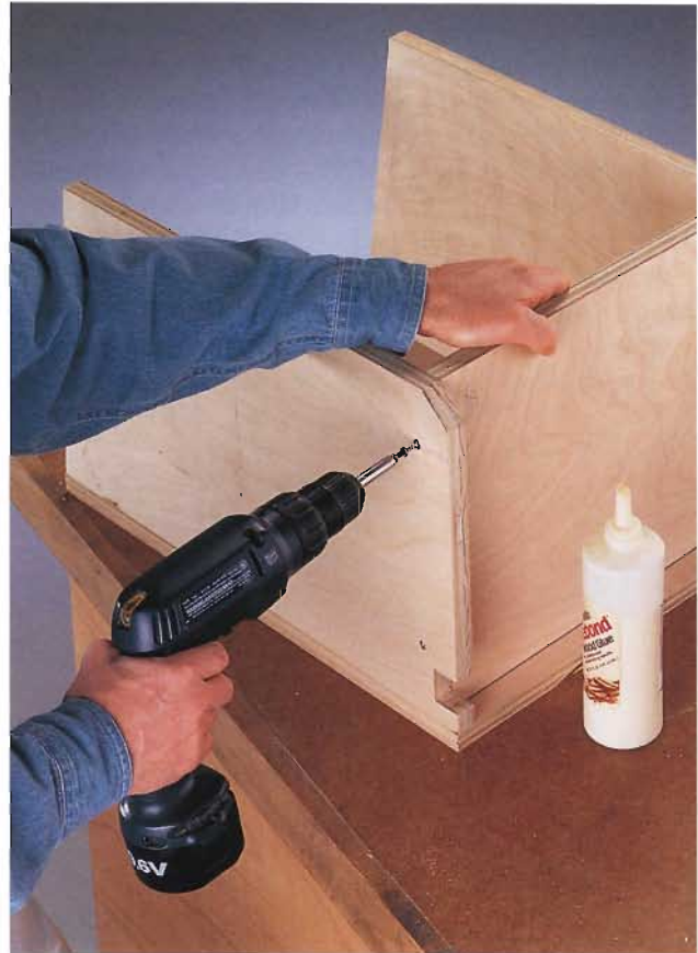
F. Position the bin bottom flush with the dowel notch, and attach it with glue and screws.
