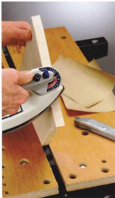
A. Apply veneer tape to the edges of the panels, using a household iron.
