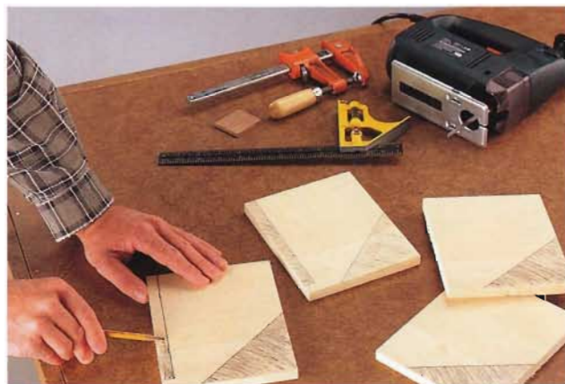
A. Shade-in the waste areas on the dividers to avoid making mistakes when cutting out the profiles.
