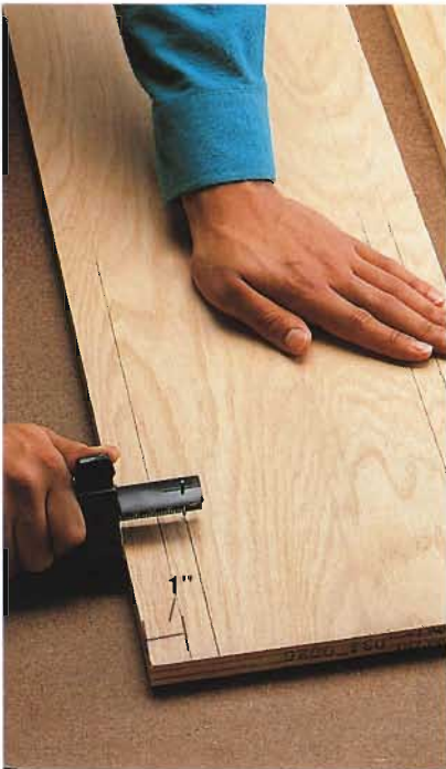
A. Mark the dado grooves at least 1" from the edges on the inside face of each riser, using a marking gauge.
