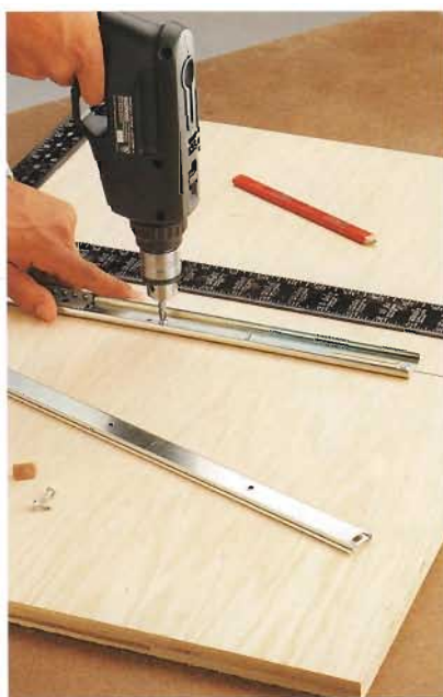
E. Attach the track for a center-mounted drawer slide at the center of one of the bottom panels.
