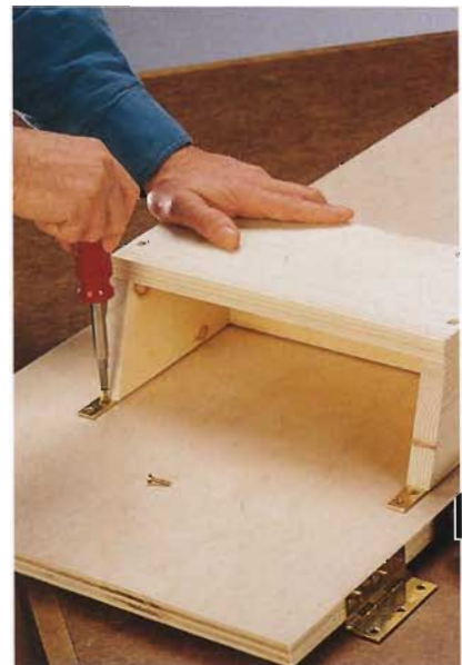
F. Use two brass mending plates to attach the box to the inside of the door.
