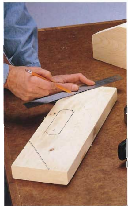
E. Lay out the handle shapes separately, using a straightedge, and cut them with a jig saw.
