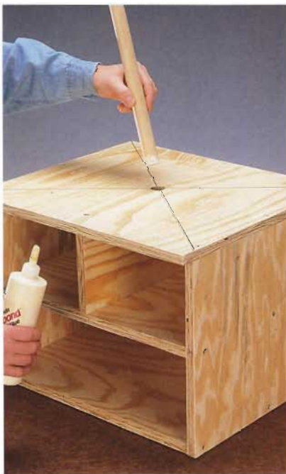
C. Apply glue to the dowel and insert it into the hole on the top of the cabinet.
