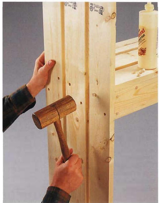
G. Use a wood mallet to pound glued \frac{3}{8} " birch plugs in place.
