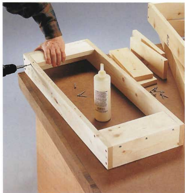
B. Apply glue and drive counterbored screws into the shelf faces and shelf ends to connect the stretchers.
