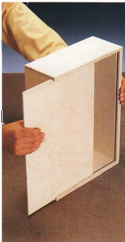
C. Slide the bottom panel into the dado grooves of the drawer assembly.
