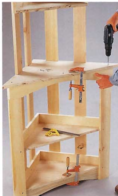
E. Drive screws through the center shelf and into the face frame.
