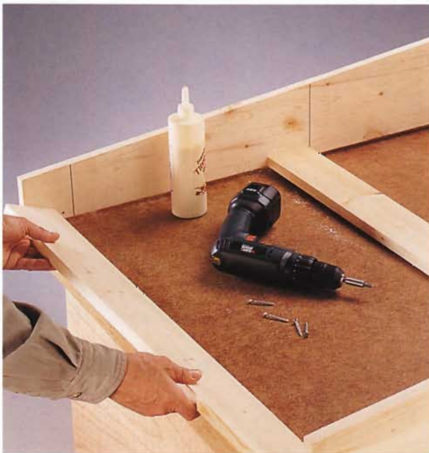
C. Fasten the spreaders between the bookcase standards. Make sure the bookcase remains square as you work.
