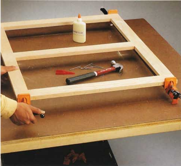
D. Cut the face frame pieces to size and clamp the rails between the stiles, reinforcing each joint with 4" finish nails.
