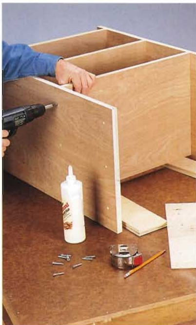
A. The duster panels support the drawers. Attach them with glue and screws driven through the sides.
