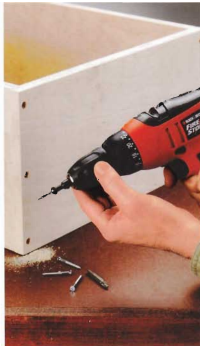
B. Assemble the panels of the box with 1½" wood screws driven through counterbored pilot holes.
