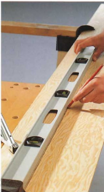
A. Use a carpenter's level to mark a straight line on the plywood strip.
