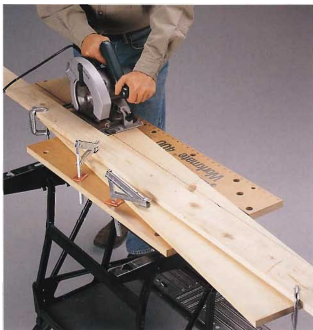
A. Clamp a straightedge to the standard, and make the taper cut with a circular saw.
