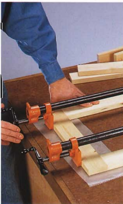
A. Apply glue to the end rails and position them between the end stiles, then clamp in place until dry.
