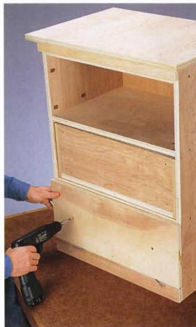
E. Drive screws through the knob holes in the drawer face to temporarily attach it to the drawer front.
