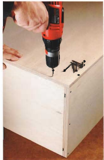
C. Assemble the cabinet sides, top, and bottom, then add the plywood back.
