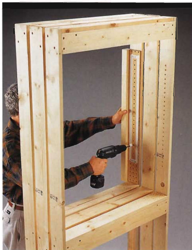
E. Use a pegboard template for uniform placement of peg holes.
