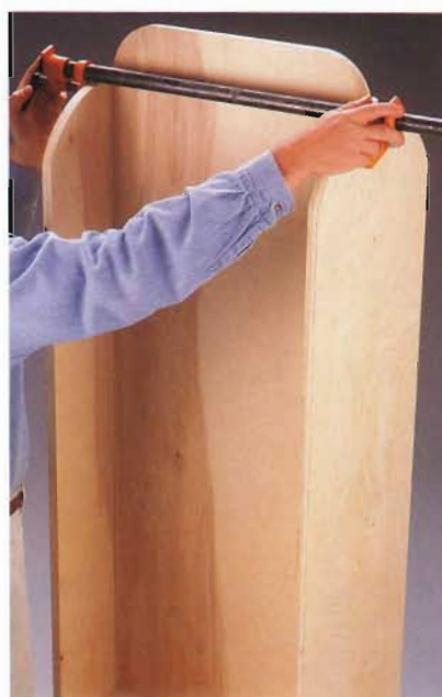
C. Install the shelves and lower rack, then clamp the side panels around the divider.
