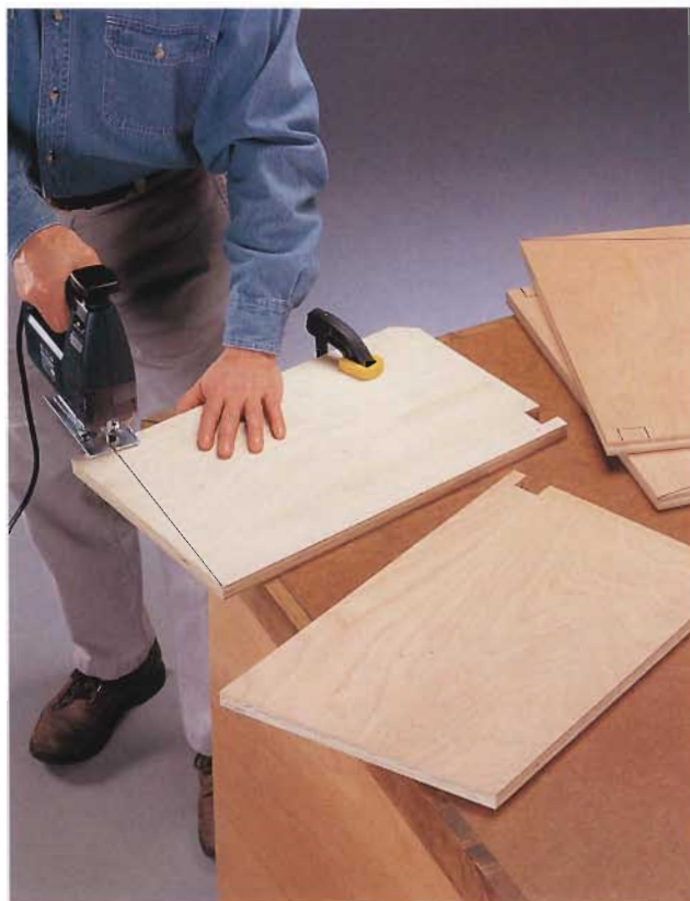
E. Clamp the bin sides to your work surface, and use a jig saw to cut the notches and bevels.
