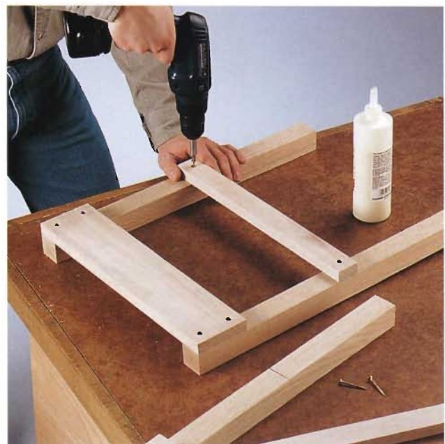
E. Attach the credenza ends and end rails to the legs with glue and wood screws.
