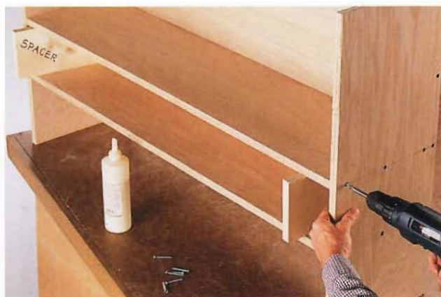
A. Use 5/4" spacer blocks set on the bottom shelf to position the top shelf for fastening.
