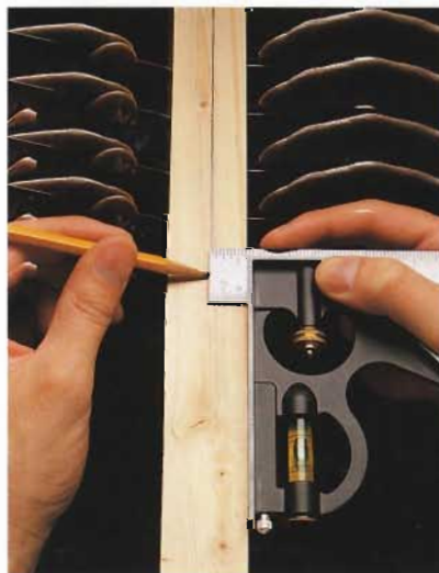
Use a combination square to mark a parallel line on the edge of the workpiece.
