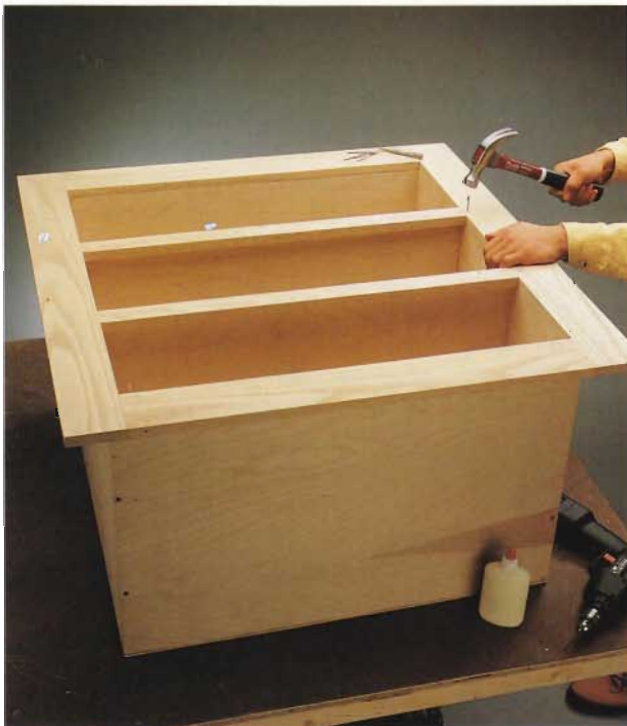
D. Glue the frame in place and attach it by drilling pilot holes and driving 1\frac{1}{2} " finish nails into the cabinet every 8". Use a nail set to countersink the nail heads.
