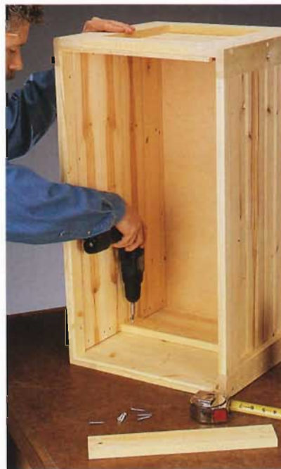
E. Fasten the handle cleats to the insides of the end panels with glue and screws.
