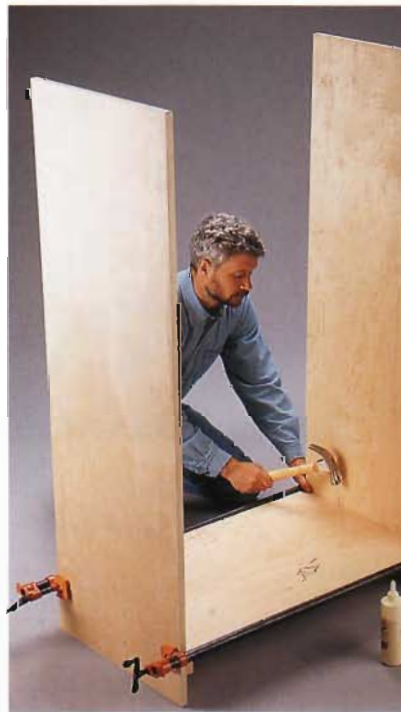
B. Clamp the bottom panel between the sides and fasten it to the cleats, using glue and finish nails.
