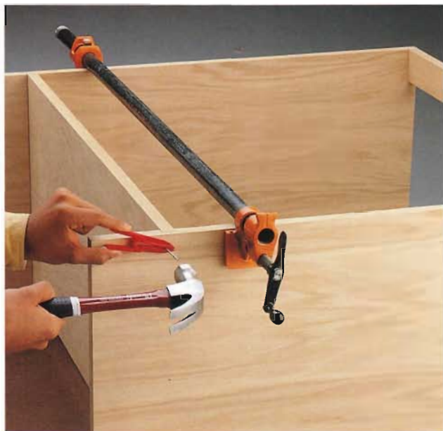
A. Assemble the side, bottom, and back panels with glue, and reinforce each joint with 2" finish nails.
