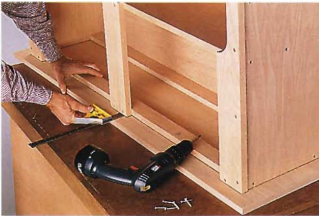
D. Measure the front and back overhang to make sure the carcass is centered on the top panel.
