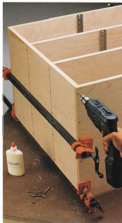
C. Clamp and glue the top and bottom panels to the side panels, then reinforce the joints with 2" screws.
