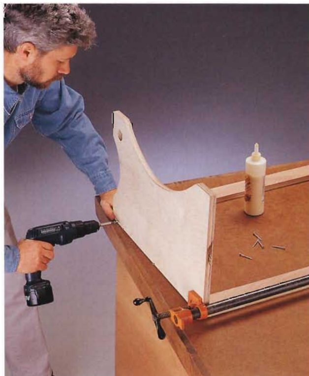
B. Apply glue and drive screws through the ends and into the stretchers. Use bar clamps to ensure square joints.
