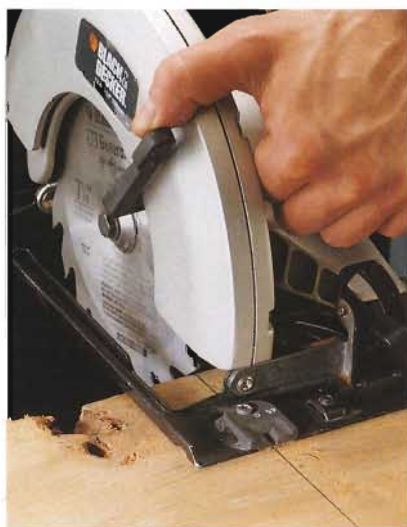
Line up the cutting guide of the circular saw with waste side of the cutting line and push the saw through the material with even pressure.
