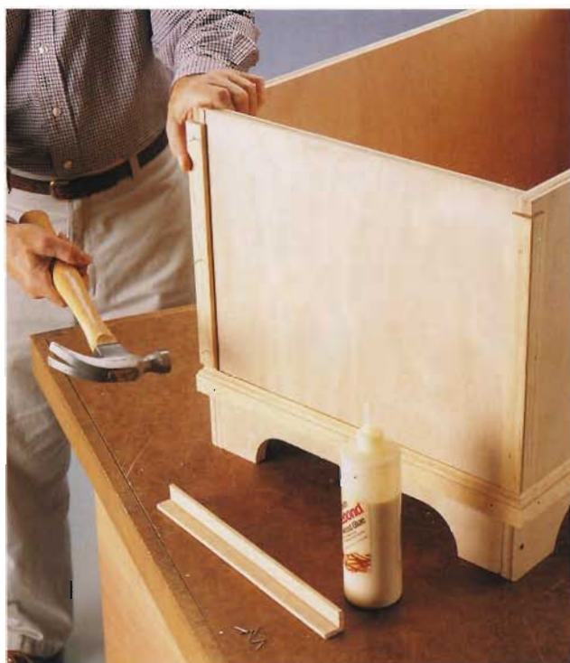
D. Fasten the corner molding over the corners to conceal the joints and screw heads.
