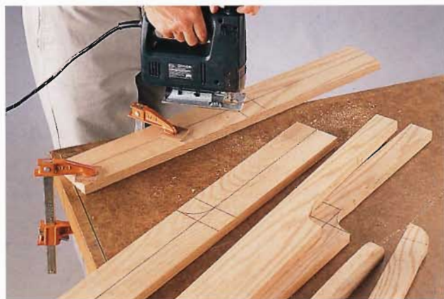
B. Cut the curved tapers in the legs with a jig saw.
