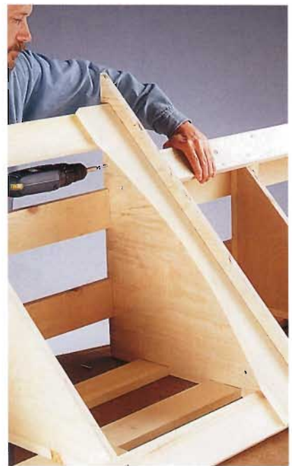
F. Drive wood screws up through the center shelf to secure the upper stiles.
