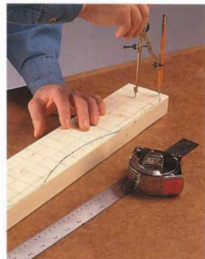
Use a compass and a square grid pattern to draw cutting lines for curves and shapes on your workpiece.
