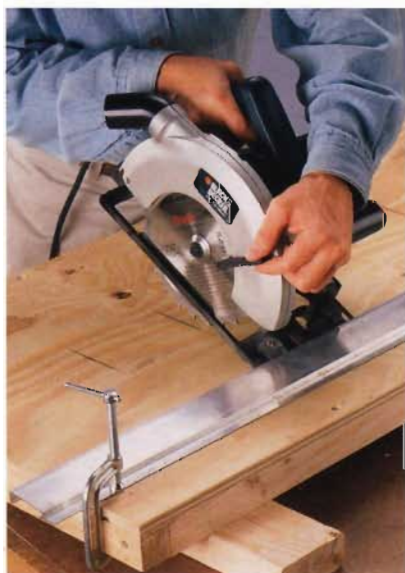
A. For ventilation, cut slots into the bottom panel, using a straightedge as a stop block for the foot of your circular saw.
