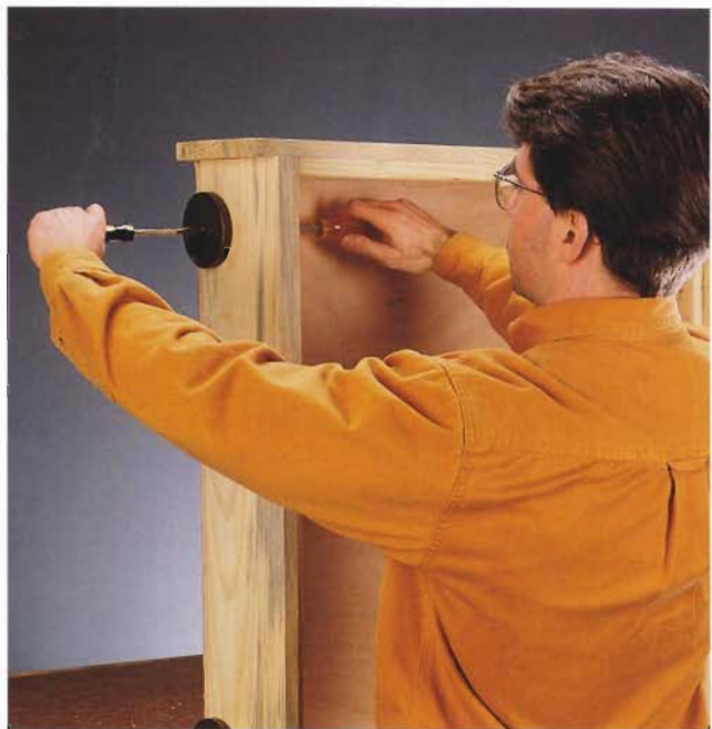
E. Mount bed-box rollers on the outside faces of the sides so the rollers extend \frac{1}{2} " below the box bottom.
