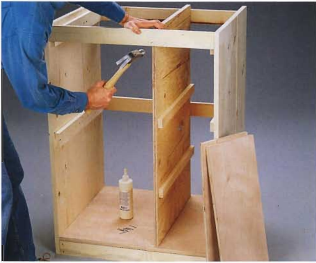
C. Install the divider 9" in from the right side of the cabinet.
