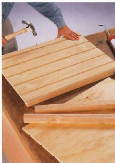
B. Position the corner braces beneath the small panels, and fasten them with construction adhesive and finish nails.
