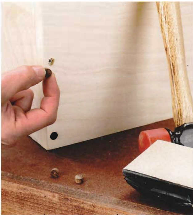
D. Insert glued walnut plugs into the counterbored pilot holes. Then sand until the the plugs are flush with the face of the box.
