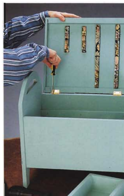
F. Attach the seat to the back of the chest with two evenly spaced 1\frac{1}{2} \times 1\frac{1}{4} " butt hinges.
