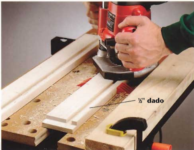
A. Cut the shelf pieces, then rout the rabbet and dado grooves for assembly.
