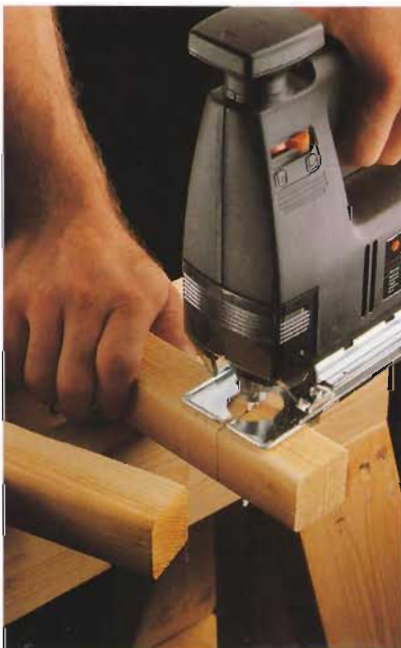
A. To build ladder brackets, cut the legs and cross braces from 2 \times 2 lumber.
