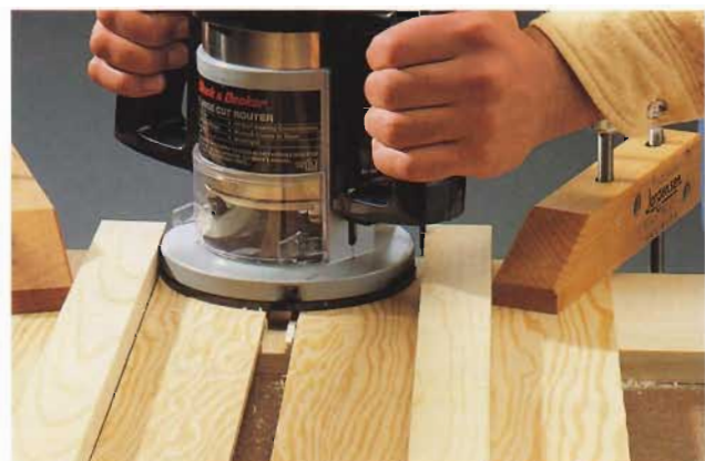
C. Rout the dado with two passes, holding the router base firmly against the straightedge cleats.
