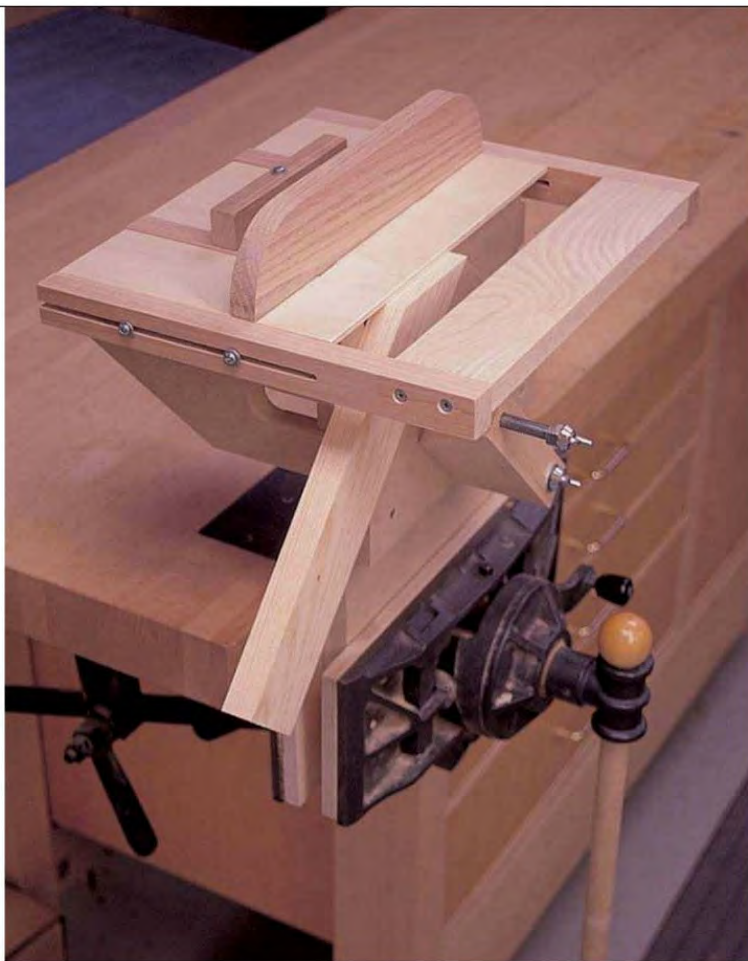
The slotting jig can be clamped in a vise or secured to the edge of a workbench. The jig's clamp swivels so it can be used to secure left- or right-hand miters.
