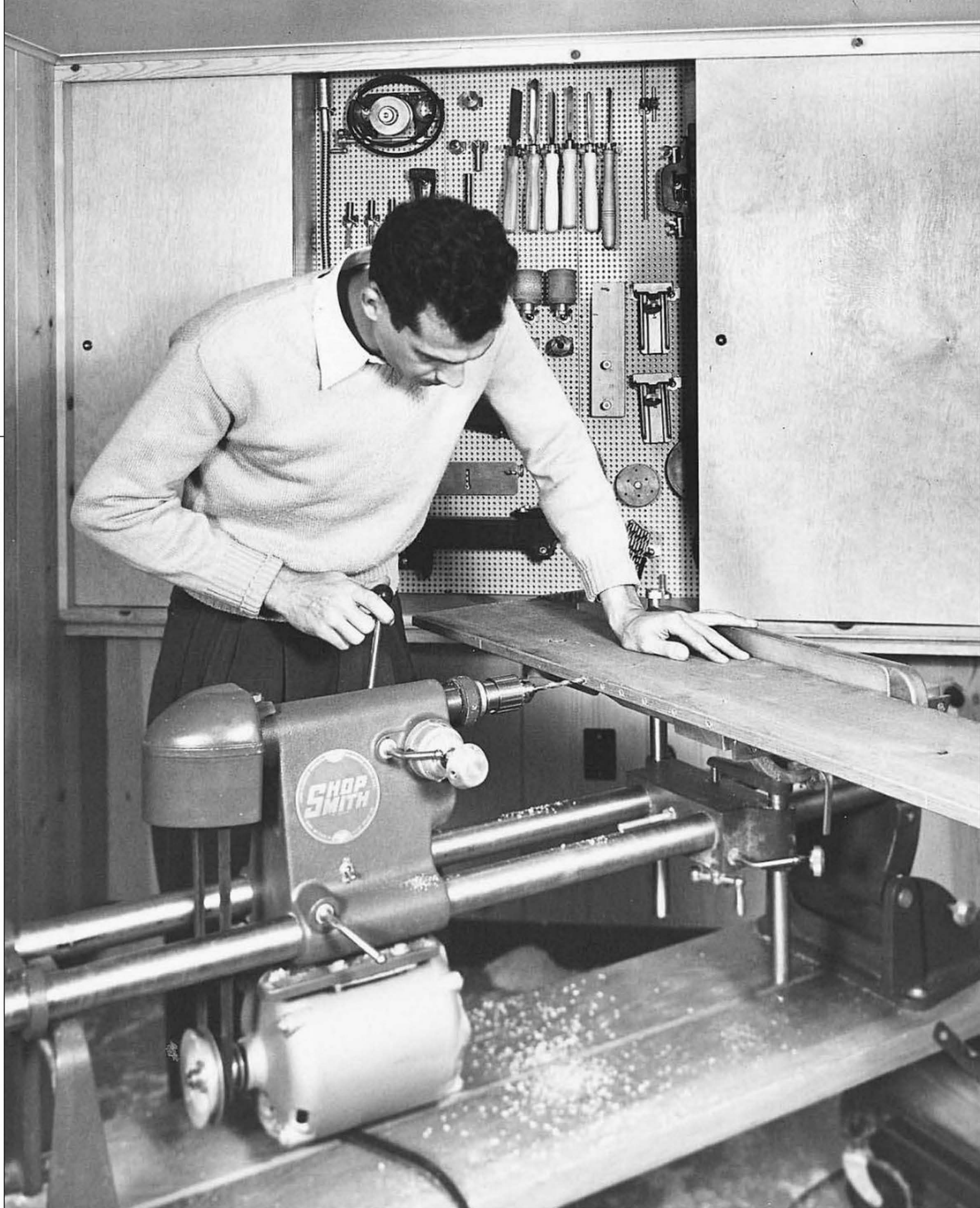
Who is the young man demonstrating horizontal boring on the Shopsmith 10ER? Why it's R.J. DeCristoforo himself, using the first power tool he ever owned.
