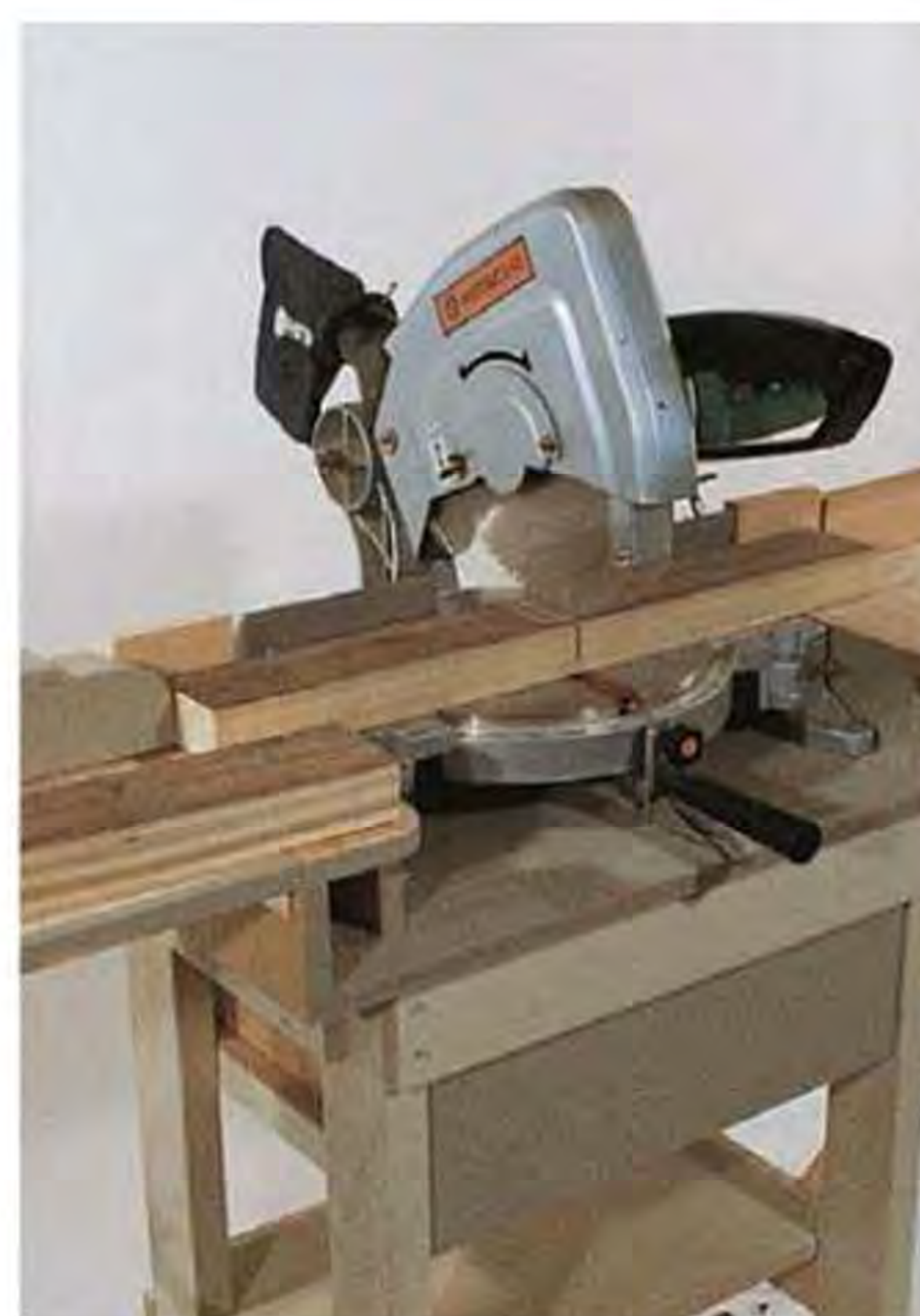
The stop functions on either side of the saw can be inverted if necessary.
