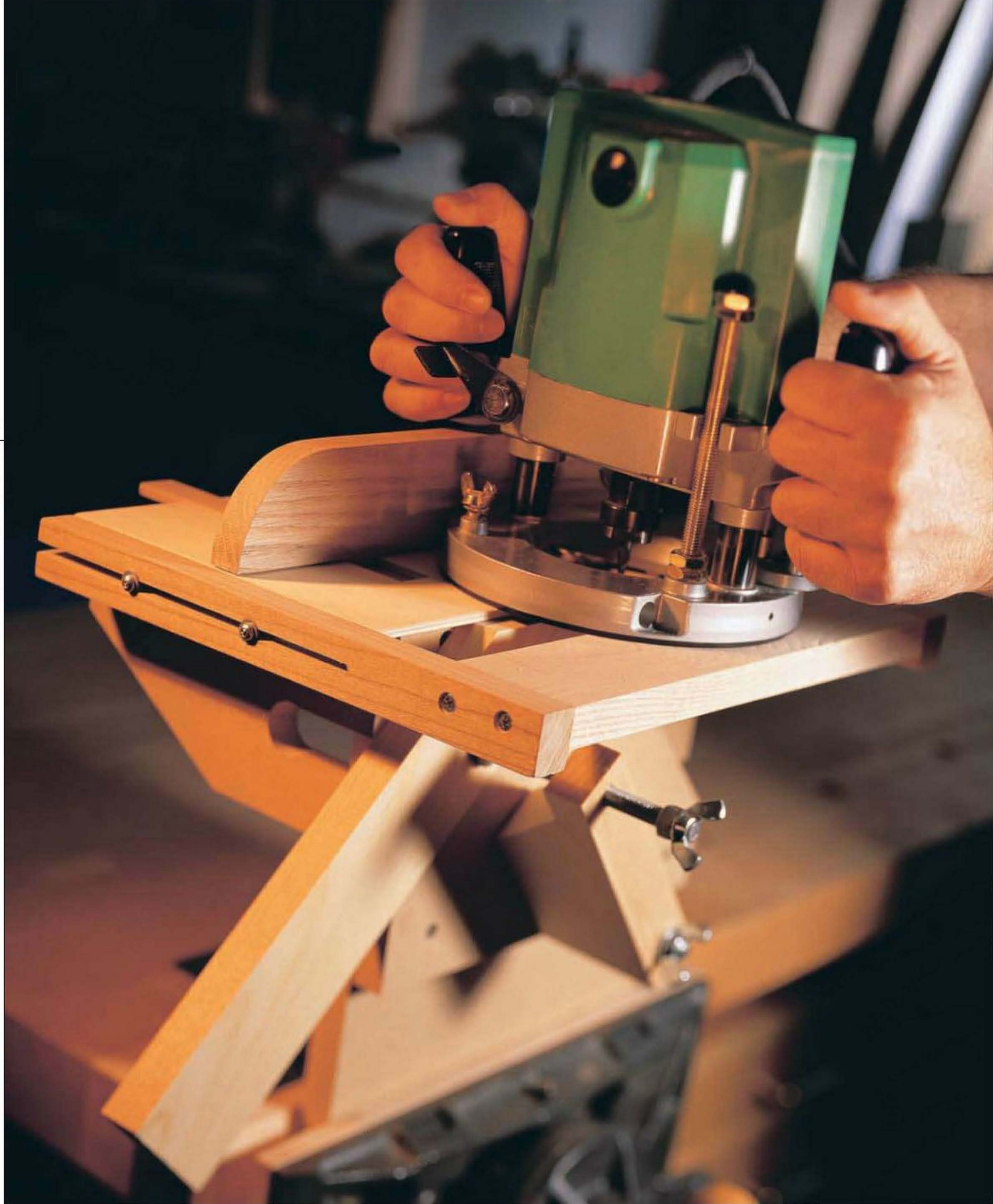
The outboard support (table extension) allows the use of even heavy-duty routers. An access slot in the jig's braces accepts a C-clamp when one is needed for additional work security.
