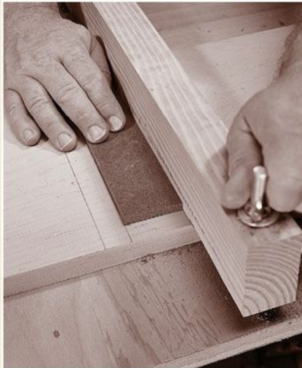
I use the positioning gauge to align the stock underneath the clamping bar. The edge of the gauge indicates the inside
