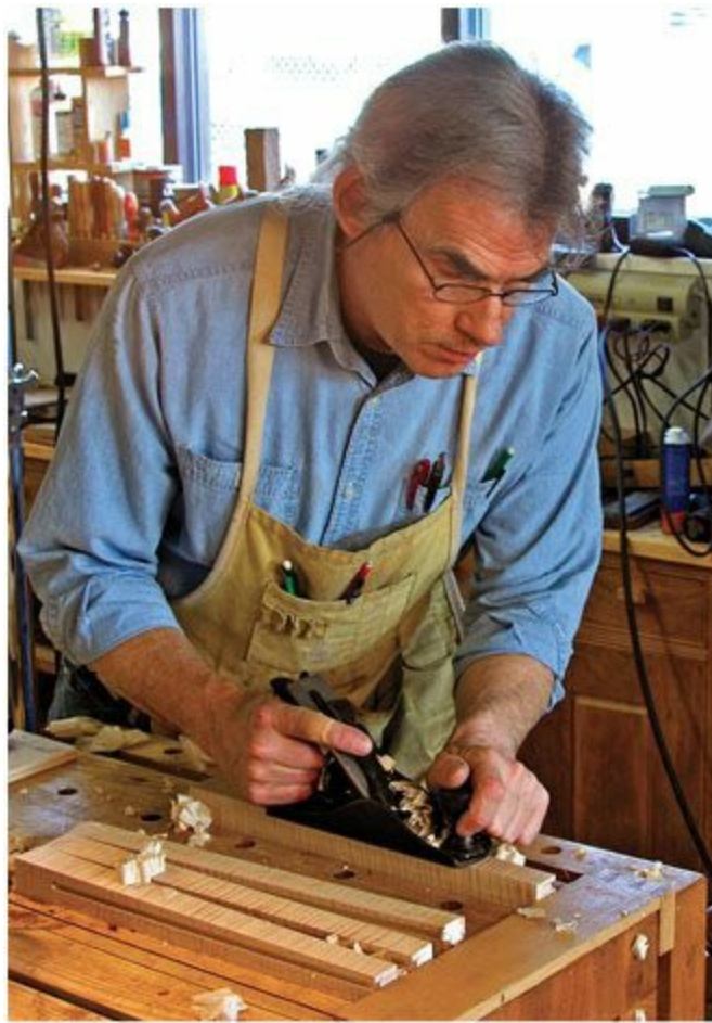
Smooth sailing. A handplane quickly removes the machine marks from the columns and it leaves a flat, smooth surface.
