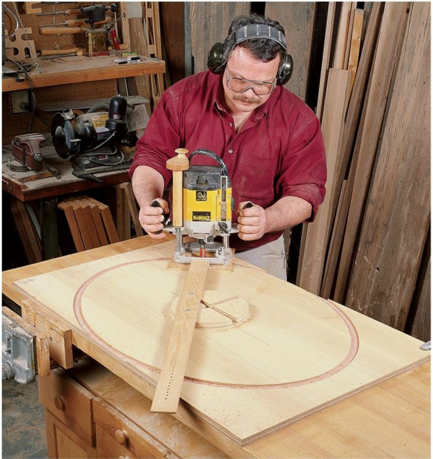
Routing an oval with a double trammel setup. The resulting curve is perfectly fair.
