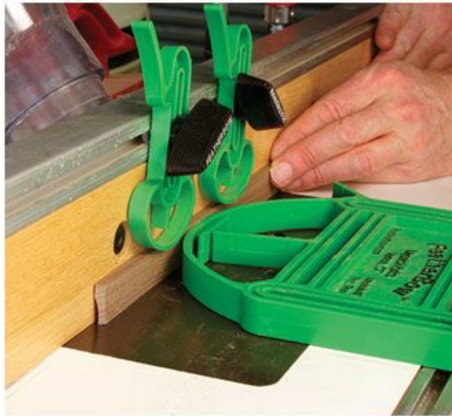
First on edge. The first cut of the cornice moulding is made with the wood on edge.
