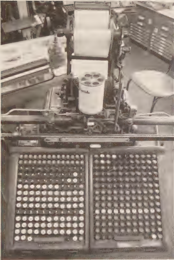
Figure 7.6 A Monotype keyboard, with punched paper tape, line-width gauge, and drumlike justification scale visible at top. Also shown here are the various QWERTY keyboards used for roman, italic, bold, or small capital letters as required. The red numeric keys (at the top left of the keyboard) are used to punch the computed justification parameters at the end of the line. 49
