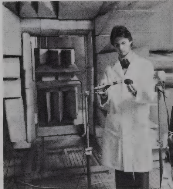
An anechoic chamber (above). The ceiling, walls, and floor have been covered with a material designed to absorb sound and cut out reverberation.
