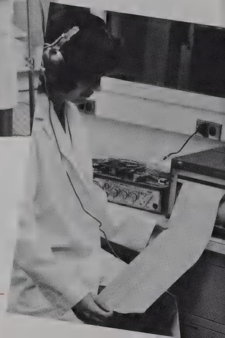
A Visicorder (below). In this technique, a light beam responds to the electrical characteristics of the speech signal and makes traces on light-sensitive paper.
