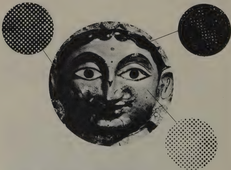
Fig. 19.7. The halftone principle
