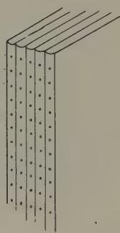
Fig. 19.18. Adhesive binding. Three types of adhesive binding are currently in use. In perfect binding , the spine is roughened and glued to receive the paper cover. In notch binding the spine is scored by a series of notches, and in burst binding it is roughened by perforation. Glue is then forced into the notched or perforated spines.
