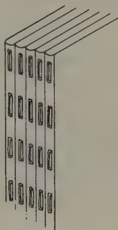
Fig. 19.18. Adhesive binding. Three types of adhesive binding are currently in use. In perfect binding , the spine is roughened and glued to receive the paper cover. In notch binding the spine is scored by a series of notches, and in burst binding it is roughened by perforation. Glue is then forced into the notched or perforated spines.
