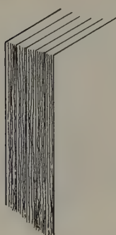
Fig. 19.18. Adhesive binding. Three types of adhesive binding are currently in use. In perfect binding , the spine is roughened and glued to receive the paper cover. In notch binding the spine is scored by a series of notches, and in burst binding it is roughened by perforation. Glue is then forced into the notched or perforated spines.
