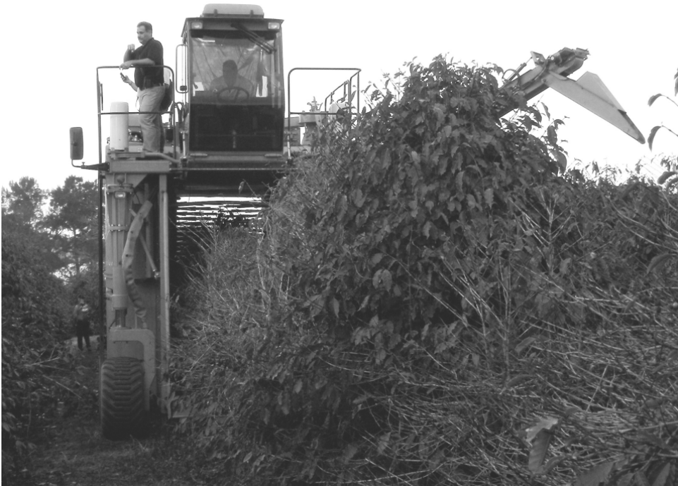
Figure 61.1. A mechanical harvester at work; the cherries are shot into the bed of a truck to the right. Brazil, 2010. Photo by Robert Thurston.
