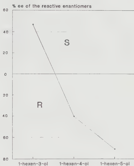
Figure 9. PPE catalyzed esterification of isomeric hexenols. (Reproduced with permission from reference 17. Copyright 1990 Pergamon.)
