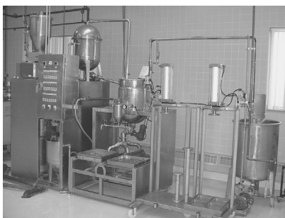
FIGURE 8.5 A pilot-plant small production scale tofu machine (Model PT-60 Ta-Ti-Hsing Co.) housed in Dr. Chang's laboratory at the North Dakota State University for traditional pressed tofu making.
