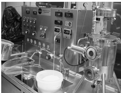
FIGURE 8.6 A small pilot-scale UHT processor (Microthermics Co.) housed in Dr. Chang's laboratory at North Dakota State University for soymilk quality research.
