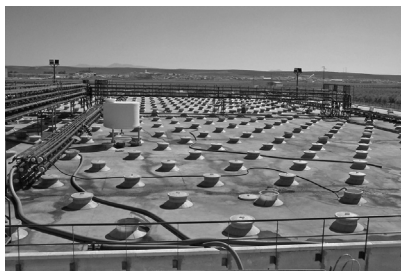
FIGURE 16.5 Bulk fermentation system used in large industries. Each fermenter has a capacity of approximately 10 tons.
