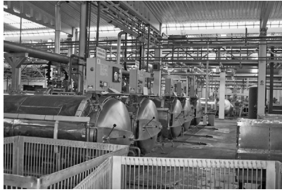
FIGURE 16.6 Retorts used for the sterilization of olives at industrial scale.
