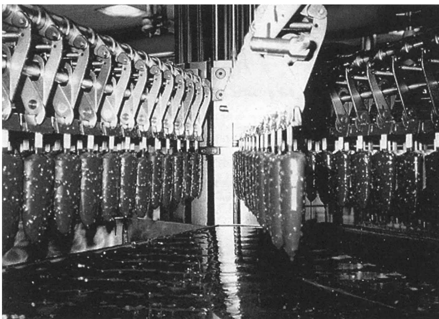
Figure 5.10 A stick product that has just been coated by dipping in chocolate
