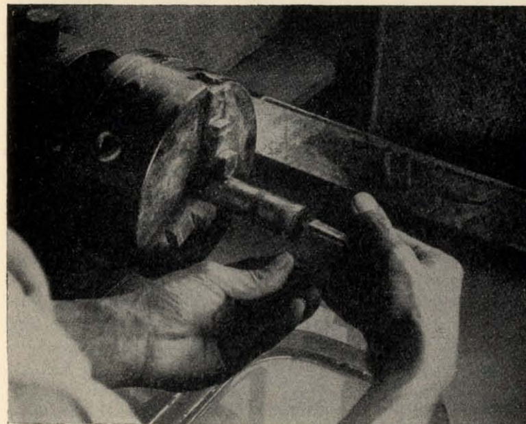
FIG. 10-5.—METHOD OF GRINDING THE KEY, USING SHEET-METAL "BUTTERFLY"
