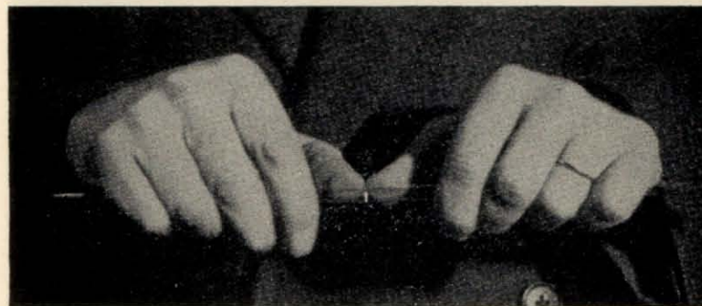
FIG. 4-2.—BREAKING A SMALL TUBE Note the position of thumbnails.
