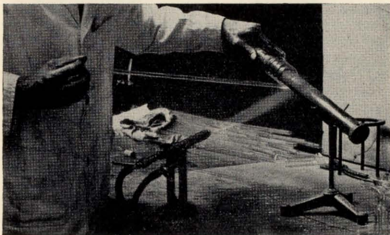
FIG. 7-10.—THE FORMER SHOWN IN THIS ILLUSTRATION IS AN ELABORATE TYPE AS USED IN A PRODUCTION GLASSBLOWING SHOP
