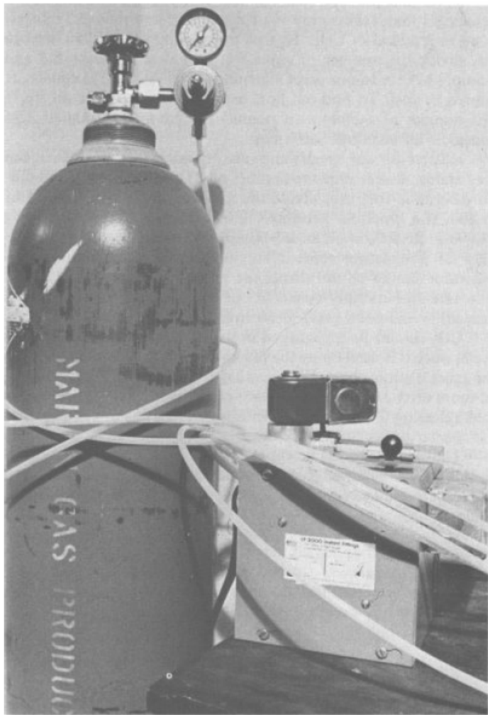
CO 2 tank with automatic regulation and flow control can more than double the growth in an enclosed grow room or greenhouse.
