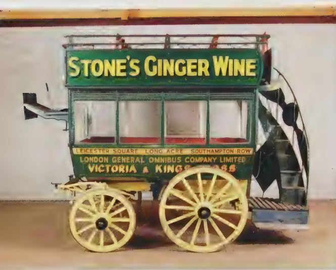
15. Garden Seat Omnibus, c.1890, in the later, improved style, with an extra-wide wheelbase, an external staircase rather than a ladder, and with proper seats on the top deck. Horse-drawn omnibuses of this type predominated in the 1870s and 1880s, before trams began to supersede them.
