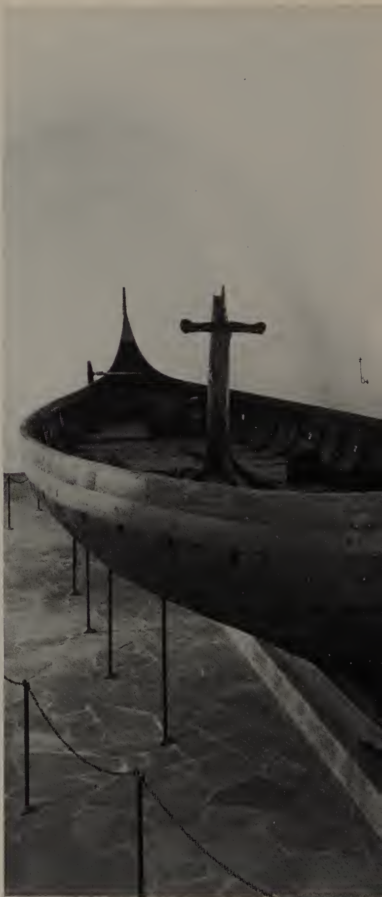
The Gokstad ship. The Viking warship made of oak and measuring 76 feet 5 inches (23.3 metres) in length which was used for a royal
