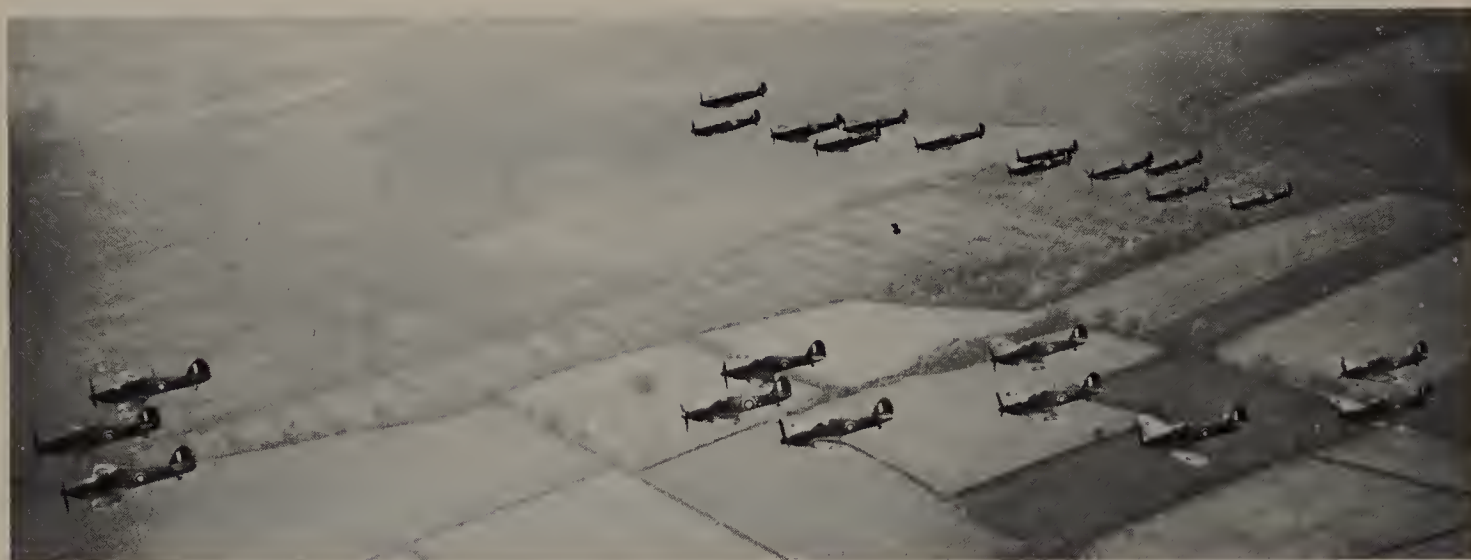
Hurricanes (foreground) and Spitfires in close formation. Both aircraft were powered by liquid-cooled Rolls-Royce Merlin engines of 1030 hp, but whereas the Hurricane had a maximum speed of 328 mph (525 kph) at 20,000 feet (6096 metres) the Spitfire could reach 362 mph (579 kph) at 19,000 feet (5791 metres).
