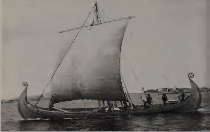
26 The Edda, a full scale replica of the Oseberg ship, during one of her earliest trials under sail in 1988. The Oseberg ship had been used as a burial ship for a Norwegian princess, and was excavated in 1904. It was 21.75m long by 5.1m wide, with 15 pairs of oars. It may have been built, c.800, as some form of high performance 'royal yacht'. Courtesy M.O.H.Carver and D.Lee
