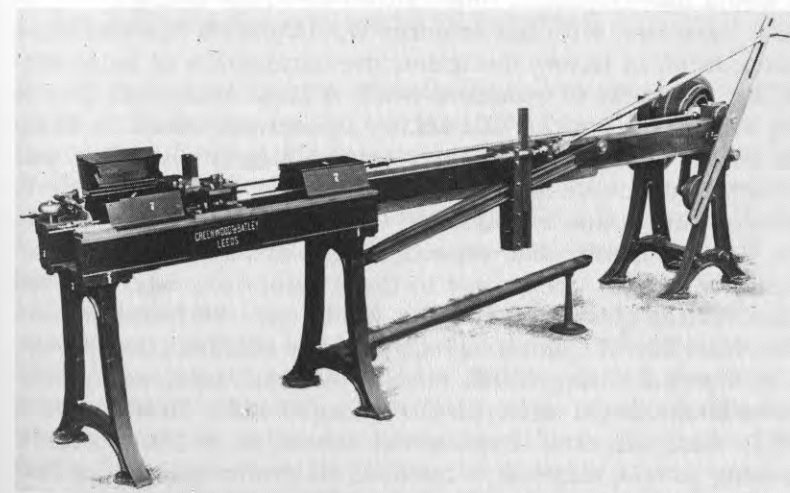
American pattern self-acting rifling machine, used to rifle barrels for the Berdan 2 infantry rifle at the Tula Armory. Purchased from Greenwood and Batley in 1871, the machine was put into operation at Tula in 1873. Rifling was the final mechanized operation on the gun barrel; fine work was crucial for the sake of the ballistic qualities of the rifle and also so as not to waste the previous work on the barrel. An index mechanism on the left side of the rifling machine automatically set the cutter that made the grooves of the barrel. Not needing to set the cutter manually, one worker could tend four machines, and each machine could rifle ten barrels in ten hours with virtually no defects. The barrel shop at Tula also used Enfield and Belgian pattern rifling machines, which could rifle an equal number of barrels but required one worker for every machine. Photograph courtesy of the West Yorkshire Archive Service, Leeds.
