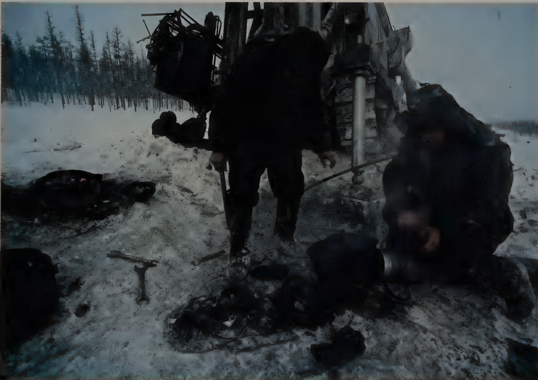
Gloveless mechanics use gasoline that has been heated to thaw and wash chilled parts of a drill.
