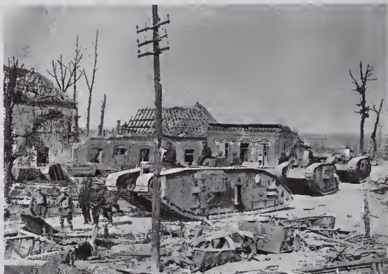
LEFT Tanks were expected to crush wire and, often using ropes and grapnels, to clear avenues for attacking infantry.
