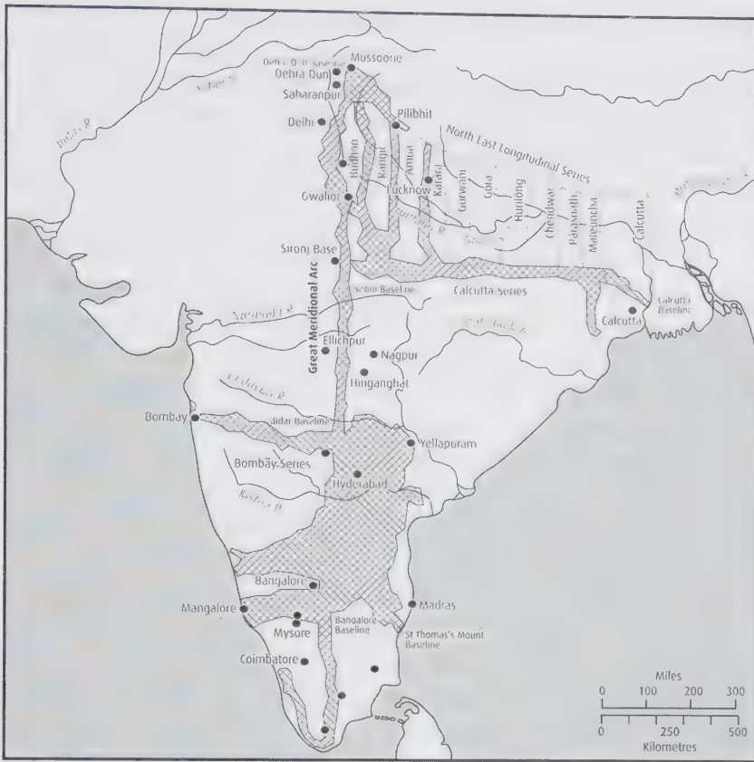
Fig. 7.2 Surveys of India: William Lambton's initial triangulation of southern India (1799–1817) and the arcs of the Great Trigonometric Survey of India, completed by 1843. Source: Edney (1997: 20). By permission of and © University of Chicago Press.
