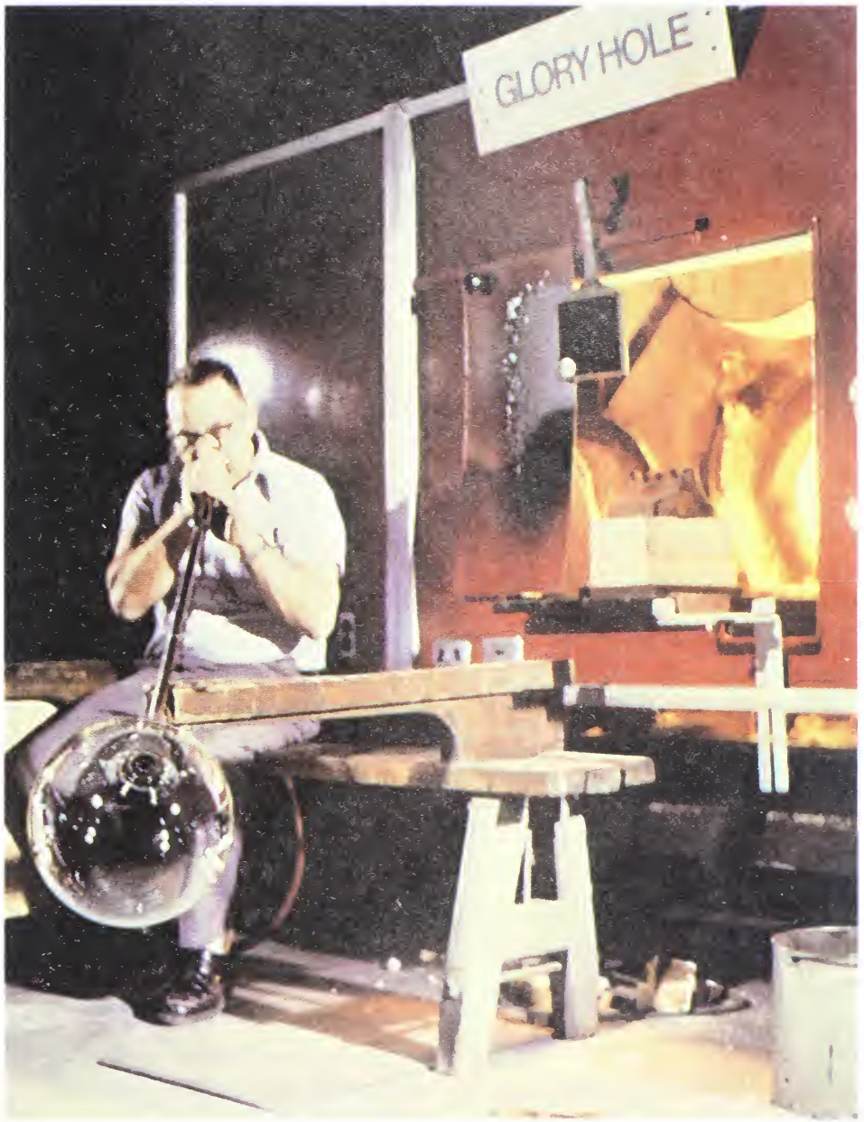
A modern glass blower at work in the Corning Glass Center, Corning, New York. The procedure he is following is described on p. 114.
