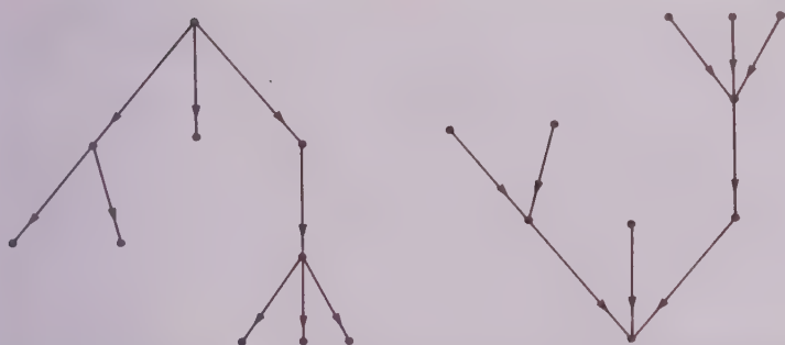
Fig. 16.2. An out-tree and the converse in-tree.
