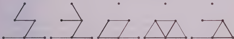
Fig. 4.8. A cocycle basis for G of Fig. 4.7.
