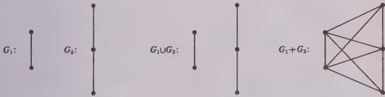
Fig. 2.16. The union and join of two graphs.
