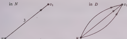
Fig. 5.8. The transformation from network to multigraph.
