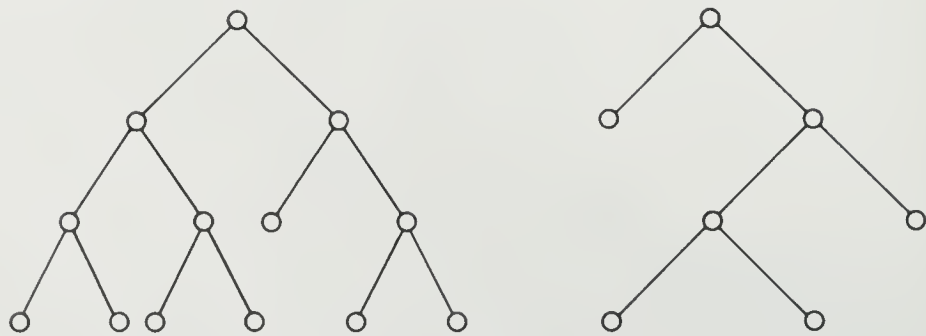
Figure 3.6 Balanced and unbalanced complete 2-ary trees
