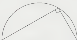
Figure 2.14. A right-angled triangle meets the semicircle on its hypotenuse.
