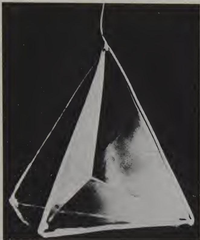
Fig. 1-7. Soap films, made by dipping a tetrahedral wire frame into a soapy solution. Notice that the tetrahedral bubble has curved faces. From Peter S.
