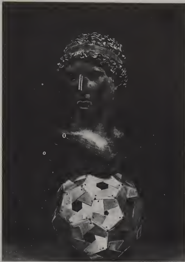
Fig. 9-23. A mechanical model illustrating rigidity in a T = 3 icosahedral lattice, built of 90 identical pieces of \frac{1}{32} -inch-thick sheet aluminum bent to represent dimers connected by pentamer/hexamer bonds. The diameter along the threefold axis is 11.5
