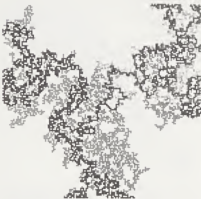
FIGURE 7.13: The backbone (filled circles) and the percolation cluster from a simulation on a 147 \times 147 quadratic lattice at p_c = 0.593 (Oxaal et al., 1987).
