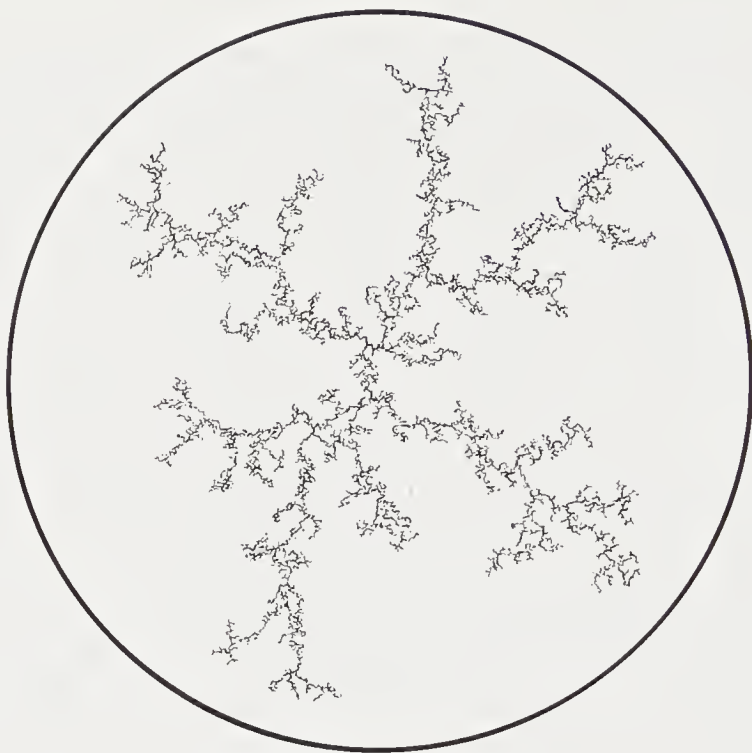
FIGURE 6.14: Fractal viscous fingering with a fractal dimension D = 1.64 \pm 0.04 in a two-dimensional porous medium consisting of a layer of 1-mm glass spheres placed at random and sandwiched between two plastic sheets. Air (black) displaced glycerol at a capillary number Ca of 0.15. The structure was observed at a time t = 0.8t_0 , where the breakthrough time is t_0 = 28.6 s (Måløy et al., 1987b).
