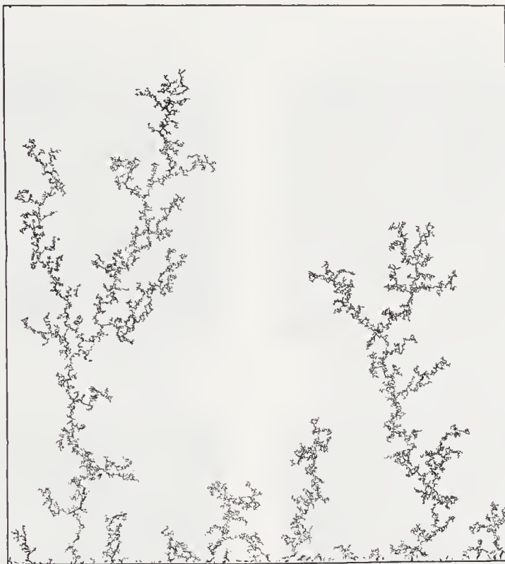
FIGURE 4.13: Viscous fingering in the displacement of glycerol by air (black) in a two-dimensional porous model. The model consists of glass beads 1 mm in diameter arranged as a close-packed random single layer between transparent plates. The model is placed horizontally. Air is injected along a line shown at the bottom in the figure, and the displaced glycerol leaves the model at the line indicated at the top of the figure (Måløy et al., 1987c).
