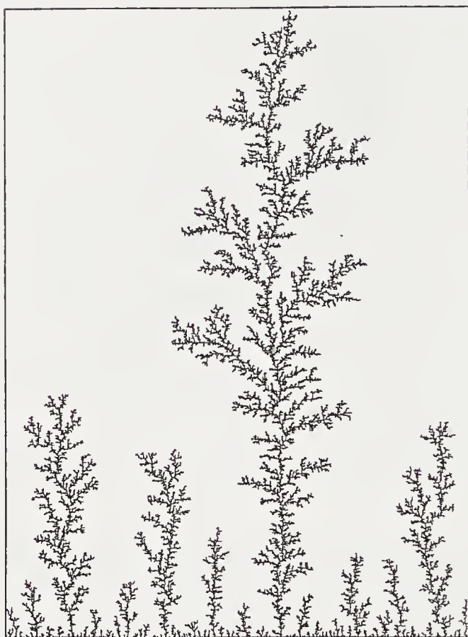
FIGURE 4.12: DLA growth from a line. The particles start on random walk trajectories from the top line and they are reflected from the side walls. The particles attach on contact to the bottom line and to trees connected to the bottom line. The baseline is 801 cells long, and the height of the longest finger is 1099. The number of particles is 47,348 (Hinrichsen et al., 1987).
