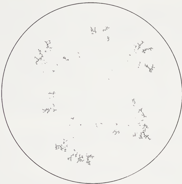
FIGURE 6.15: Active growth zone of the viscous fingering structure shown in figure 6.14. The time between the two pictures used to construct the growth zone was 2.8 s, which corresponds to a relative time increment of \Delta t/t_0 = 0.10 (Måløy et al., 1987b).
