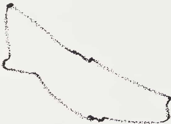
FIGURE 6.10: The experimental attractor for thermal convection. The time series of temperatures, x_t , is used to plot the temperature at time t + 1 , i.e. x_{t+1} , versus x_t . The figure corresponds to a projection of the attractor of the motion in phase space (Jensen et al., 1985).
