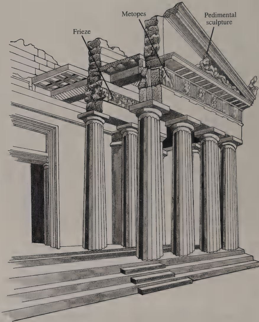
Figure 6.2. Sectional Drawing of the East End of the Parthenon Showing Relationship of Frieze, Metopes, and Pediment (After N. Yalouris)
