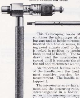
This Telescoping Inside Micrometer combines the advantages of a telescoping gage and an inside micrometer. When inserted in a hole or recess, the measuring point adjusts itself to the work and is locked in position by turning knurled knob at end of handle. The tool is withdrawn and the micrometer thimble is turned until it contacts the shoulder on the rod and micrometer reading is taken.
