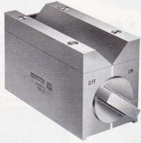
Permanent Magnet V Block No. 750D follows the principle of Brown & Sharpe Permanent Magnet Chucks. It is designed for holding iron or steel work of round or rectangular cross section and, also, irregularly shaped pieces which can be placed between and in contact with the V faces. It is suited particularly for toolmaking, inspecting and manufacturing
