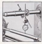
For use in holding dial indicator swivel and arm to arbor, spindle or similar machine member while checking runout of parts or alignment of fixtures. Brass shoe on end of bolt swivels to prevent injury to a finished surface.
