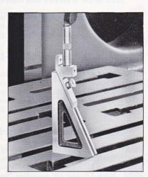
No. 625 is set accurately to micrometer and permits a range of settings from  $\frac{1}{4}$ " to  $\frac{81}{2}$ ".
