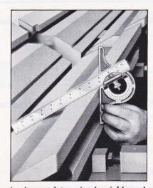
Angles are determined quickly and accurately with a Protractor.
