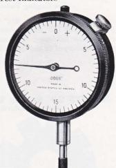
Can be attached to any of our indicators, with exception of No. 740, which requires a smaller gage. Also used on special attachments for testing purposes on machine or bench work.
