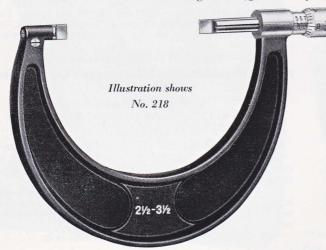
For measuring depths of narrow grooves and diameters of forming tools. Blade on spindle end does not rotate. Blades are .030" thick and permit measurements in slots having a depth up to  $7_{52}$ ".
