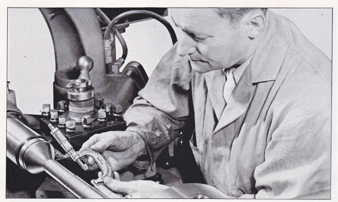
In addition to the general usefulness of ordinary micrometers the two-inch Micrometer Calipers Nos. 47, 47RS, 48 and 48RS have a narrow anvil end which gives them advantages in measuring in narrow slots, keyways and other places inaccessible to micrometers with frames of the conventional type.
