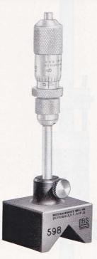
In conjunction with an inside micrometer, this attachment makes a useful, accurate and economical combination. The end of the micrometer measuring rod is first lined up with the base of the attachment, the clamp screw is tightened, and the tool is ready for use. The V groove adapts it for use on cylindrical work. It is convenient not only as a height gage but for many other measurements as well.
