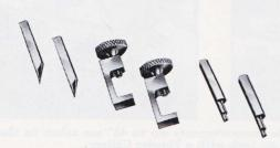
Center Points quickly convert a 6" or 150 mm. vernier caliper into a direct reading precision divider. With them the distance between two points or between a point and some locating part is determined precisely.
