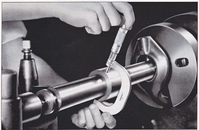
When using a large micrometer, frame should be held securely in one hand at point where weight of tool is supported most conveniently without cramping the measuring surfaces. The finger and thumb of other hand should turn the thimble.
