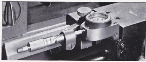
Micrometer Heads serving as integral parts of machines accurately determine table or carriage movements as well as tool settings.
