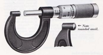
Anvil is rounded. Back of frame at anvil is cut away so that anvil enters tubing as small as  ${}^{1}/_{22}$ " inside diameter. Has black enameled, I section frame. Thimble and barrel have rust resistant, dull chrome finish with easily read black graduations. Thimble is large diameter with wide divisions. The micrometer screw is hardened with accurately ground threads. Smooth, tapered surfaces provide extremely accurate sliding adjustment for wear on threads. Thimble is locked to spindle.
