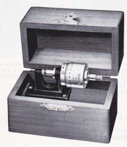
It is found of service to wire drawers, watchmakers and others who desire fine measurements, and where the work is of such a class that a micrometer can be used when placed on a bench.
