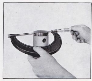
Micrometer Calipers Nos. 55 and 55RS with 2 to 6-Inch Range are Extremely Useful. In Motor Service Work they
