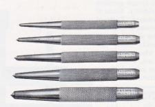
Brown & Sharpe Center Punches are made of tool steel selected for this type of work. They are hardened and both ends are tempered. Center Punches are about 4" long and have a nicely knurled finger grip. Points are ground carefully at an angle which will give maximum strength and penetration and at the same time provide a punch mark in which drills will start easily.
