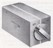
Permanent Magnet Block No. 760 follows the principle of Brown & Sharpe Permanent Magnet Chucks. Iron or steel work wide enough to span the insert in center of top of block can be held firmly. It is suited particularly for toolmaking, inspecting and manufacturing and for both wet and dry grinding.
