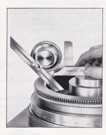
Bevel Protractor measuring angular clearance on ring gear.
