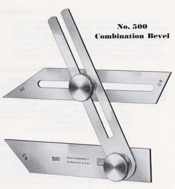
With this tool it is possible to transfer any angle from one surface to another. It can be used, also, for laying out angles as the back of the tool is smooth and can be laid flat on the work.
