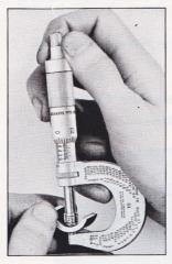
With attachment on spindle, micrometer measures wall thickness of the curved section at any point, no matter how long the piece.
