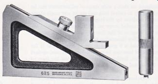
With this gage, time spent by the planer hand in adjusting the cutting tool is reduced to a minimum. By setting gage to a micrometer, surface gage or caliper and bringing the planer tool in contact with it, the first cut may be relied upon to give the desired dimension. This gage may be used on its side as diameter of adjusting nut is less than thickness of base.
