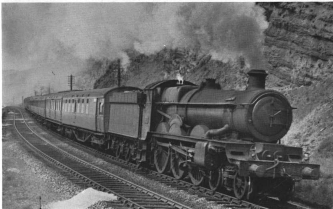
lower: With standard boiler, top feed external steam-pipes — "Star" class, No. 4043, Prince Henry near Dawlish. [E. D. Bruton.]
