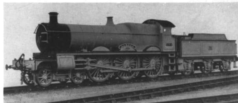
The first full exploitation by Churchward of his design features—No. 171, Albion in 1903.
