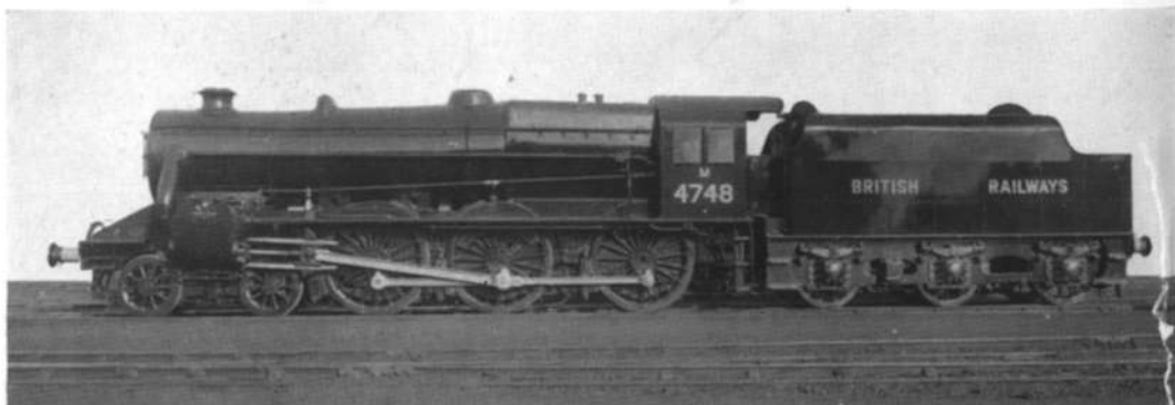
"Black Stanier" with Caprotti valve gear, No. 4748.
