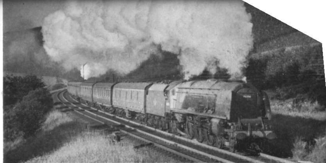
British Railways No. 46256, Sir William A. Stanier F.R.S. fitted with Ivatt's Delta trailing truck.
