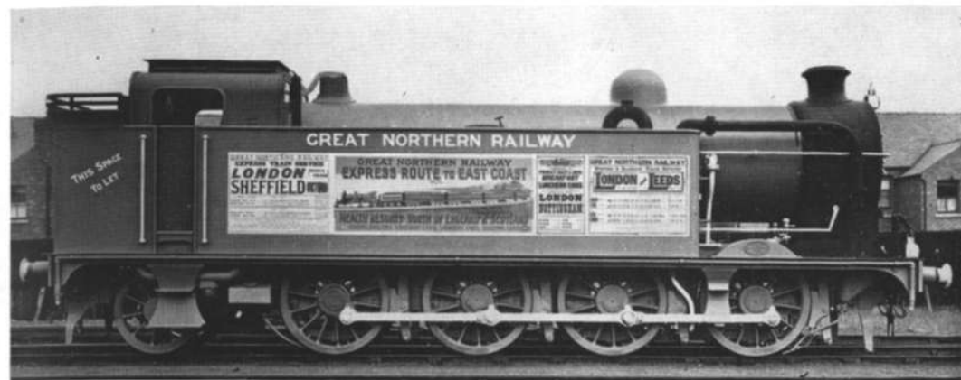
Ivatt's 0-8-2 condensing suburban tank, No. 116, as first built in 1903 with long tanks, which probably prompted this short-lived advertising scheme. The pictorial poster shows No. 990 with a train of 6-wheel-bogie carriages.
