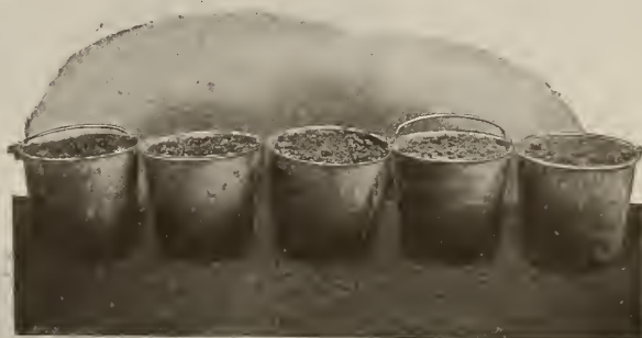
FIVE PAILS OF DIRT WASHED FROM AIR DURING ONE WEEK'S OPERATION OF AIR WASHER
