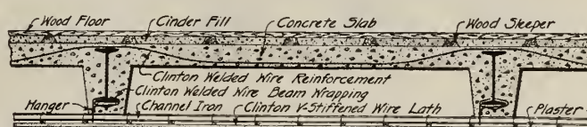
Fireproof System Showing Finished Floor and Ceiling
