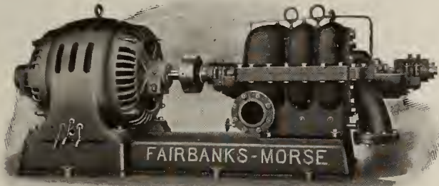
FIG. 1000. 5-INCH, 3-STAGE, HORIZONTALLY SPLIT CASING CENTRIFUGAL PUMP, DIRECT CONNECTED TO 75 H.P. FAIRBANKS-MORSE INDUCTION MOTOR
