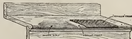
APPROVED METHOD OF REPAIRING WORN STEPS
