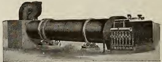
DRYER USING INDIRECT STEAM HEAT
