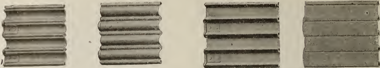
Interlocking Steel Slat No. 2 Fitted with alternate endlocks. It is 1\frac{13}{16} ins. wide on centers, depth of crown, \frac{9}{16} in. Made in gages Nos. 24, 22, 20, 18 and 16. Especially adaptable to shutters equipped with mechanical operating device Interlocking Steel Slat No. 5 Fitted with alternate endlocks; 1\frac{1}{2} ins. wide on centers, depth of crown, \frac{1}{2} in. Made in gages Nos. 22, 20 and 18. Especially designed for doors and shutters manually operated by handle in bottom bar. When in perpendicular arrangement, shoulders are brought into rigid alignment
