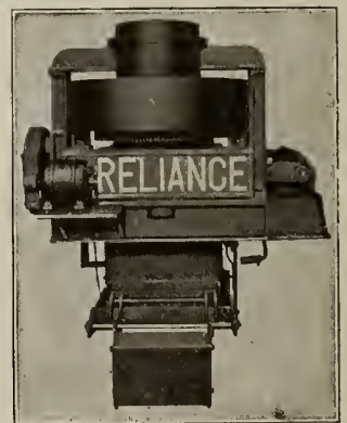
RELiance AUTOMATIC COAL SCALE Front view showing driving gears and operating shaft in dustproof case, and hopper bottom
