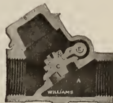
FIG. 254. SECTIONAL VIEW OF MEDIUM REGRINDING SWING CHECK VALVE
