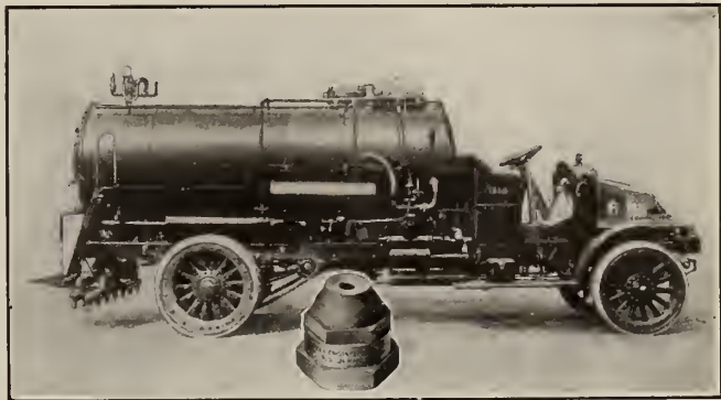
SPRAYING BITUMINOUS BINDER WITH “SPRACO” NOZZLES
