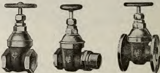
FIG. 1 FIG. 2 FIG. 3 BRONZE GATE VALVES 1/4 in. to 2 1/2 ins., 175 lbs. working pressure, 350 lbs. test 3 to 4 ins., 125 lbs. working pressure, 300 lbs. test
