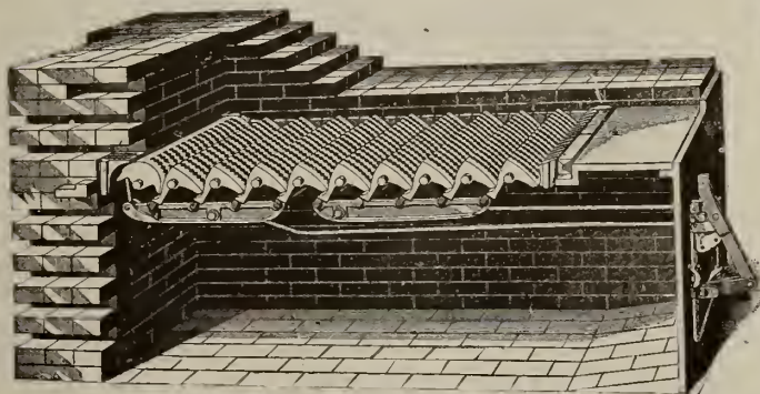
GRATE SHOWING SHAKING POSITION
