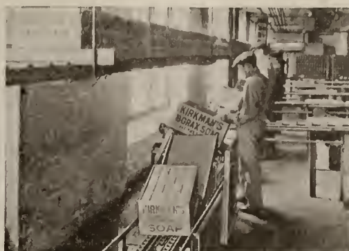
Packing of all kinds of products systematized by Lamson conveyors. Conveyors bringing empty boxes and bars of soap to packers and carrying packed boxes away to nailing machines
