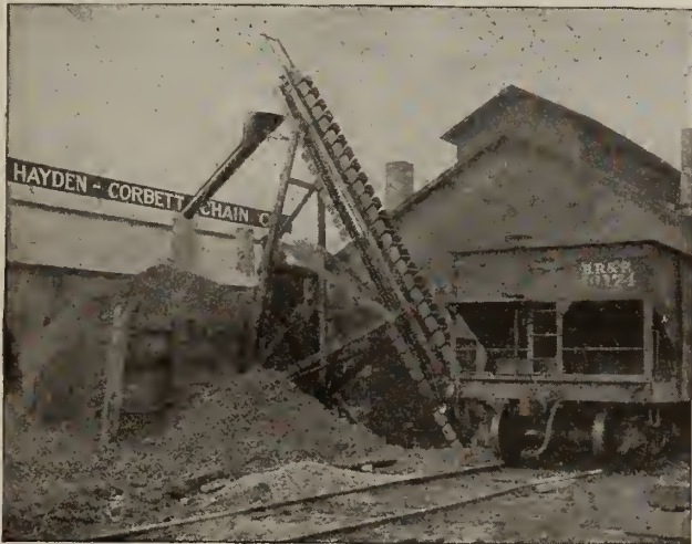
COKE BEING FED DIRECTLY INTO BUCKETS OF CONTINUOUS BUCKET ELEVATOR BY THE "COLUMBUS" RECIPROCATING FEEDER
