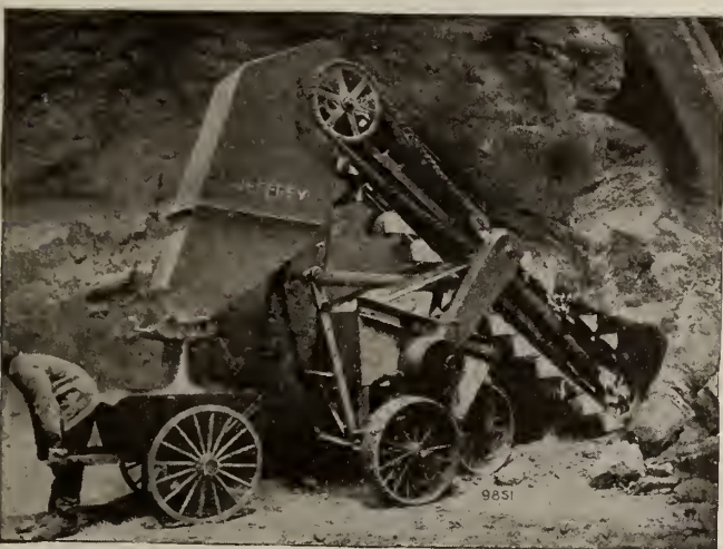
DIGGING AND LOADING HARD ACID PHOSPHATE IN FERTILIZER PLANT WITH JEFFREY TYPE "G" LOADER
