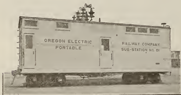
500 KW. PORTABLE SUBSTATION. 60000 VOLTS A.C.; 1200 VOLTS D.C.
