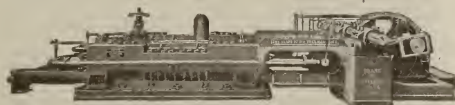
DEANE FORGED END HORIZONTAL POWER PUMP FOR OIL LINE HEAVY PRESSURE WORK
