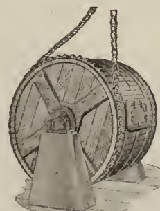
TANNERS' DRUM DRIVEN WITH CHAIN AND SPROCKET
