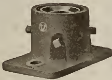
VERTICAL SHAFT STEP BEARING Adjustable in all directions. Tempered steel button and babbitted bushing, surrounded by oil reservoir of ample capacity. Operates with minimum friction loss
