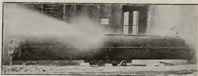
FIG. 2. HYDRAULIC TEST ON 42-INCH PIPE Showing riveted pads blown out at gage and inlet; lock-bar joint remaining tight
