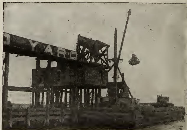
No. A-904. HAYWARD CLASS "E" CLAM SHELL BUCKET On a mast and gaff rig, unloading coal from barge and dumping into hopper
