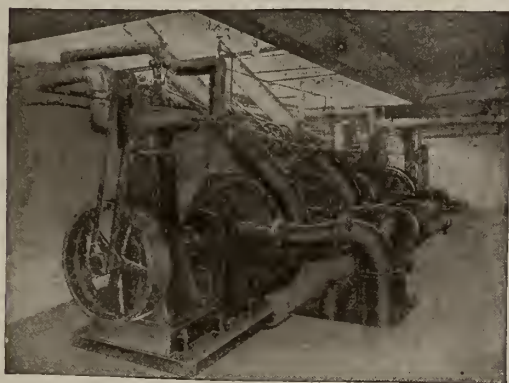
"ABC" TYPE A ENGINES DRIVING CENTRIFUGAL PUMPS Used for barometric condenser service
