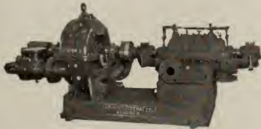
FIG. 516. LEA-COURTENAY 4-STAGE BOILER FEED PUMP, DIRECT CONNECTED TO STEAM TURBINE Designed to deliver 400 gals. per minute against an 800-ft. head
