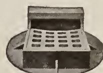
FIG. 162AK. CATCH-BASIN INLET Top 23 in. by 32 in. Bottom flange, 42 in. diam. Grating concave at rear
