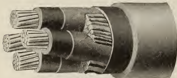
AMERICORE LEAD INCASED CABLE 4-conductor, stranded, rubber, tape, jute and lead
