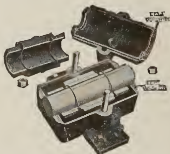
CLARAGE FAN BEARING OPEN FOR INSPECTION
