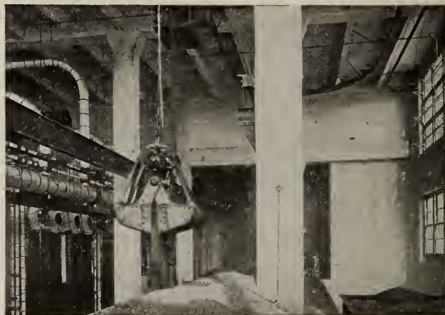
No. A-2456. HAYWARD ELECTRIC MOTOR BUCKET Rehandling fuel in a boiler room from car to bunkers
