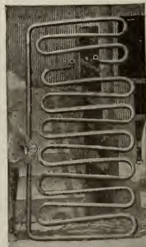
2-in. Special Cooling Coils, for Hearth Jacket Plates
