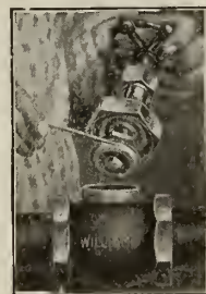
FIG. 107-E Applying oil and emery, which is always at hand, when new discs are not. Contrast this with costly method of inserting new discs which are not always available when needed
