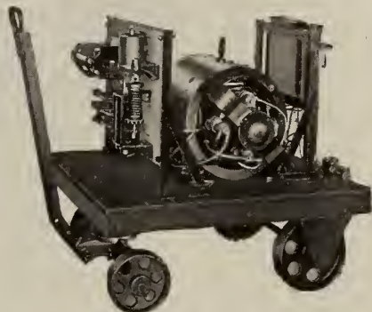
ONE-ARC, DYNAMOTOR TYPE, PORTABLE OUTFIT
