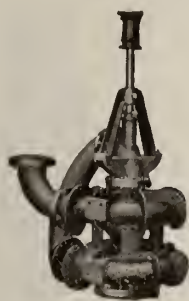
TYPE H High pressure, 2-stage, vertical shaft, for total heads to 150 ft.
