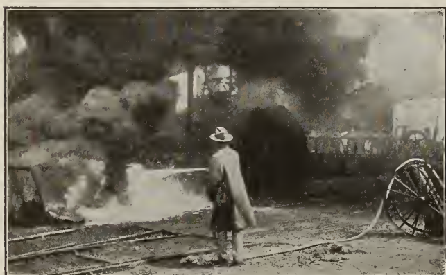
FIERCE FIRE IN PIT (11 by 13 ft.) AT COKE PLANT Tar, benzol and gasoline burning. Foamite Firefoam engine just starting
