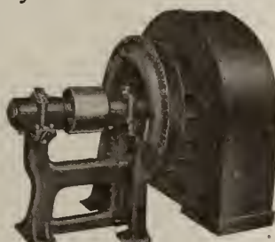
CLARAGE STYLE "C" EXHAUST FAN Multiblade wheel partly removed from housing
