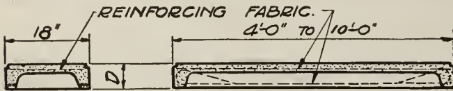
DETAIL LONG SPAN "CHANNEL" TYPE GYPSUM ROOF TILE
