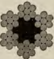
Fig. 5 HAULAGE AND GUY ROPE Round strand (6 x 7)
