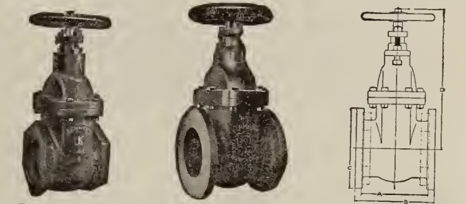
Fig. 57. Screwed "STANDARD" IRON BODY, BRONZE MOUNTED GATE VALVE Fig. 58. Flanged "STANDARD" IRON BODY, BRONZE MOUNTED GATE VALVE Fig. 59. Dimension Diagram MOUNTED GATE VALVE With double disks, parallel seats, inside stationary stem of bronze of 50,000 lbs. tensile strength
