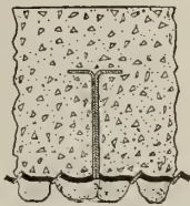
T-RIB COVERED COMPLETELY BY CONCRETE
