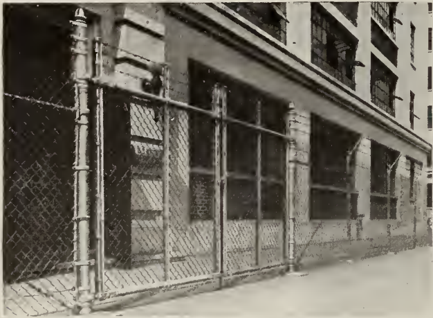
PLATE NO. E3693. ANCHOR POST CHAIN LINK FENCE WITH ELECTRICALLY WELDED GATES, ERECTED AT THE U. S. FLEET SUPPLY BASE, SOUTH BROOKLYN, N. Y. Height.....7 ft. Length.....5100 ft. Fabric.....Chain link woven steel—wire No. 9 gage, 2 in. mesh
