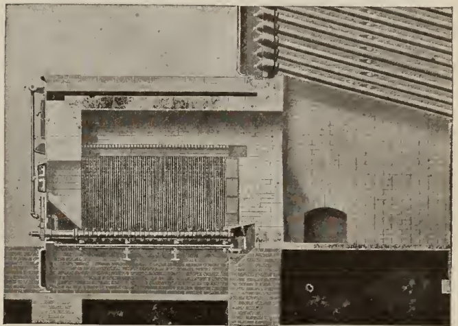
MURPHY AUTOMATIC STOKER Dutch oven setting
