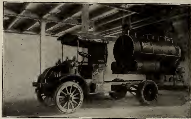
FIG. 67. TANK AND SPRAYING EQUIPMENT REMOVED FROM CHASSIS
