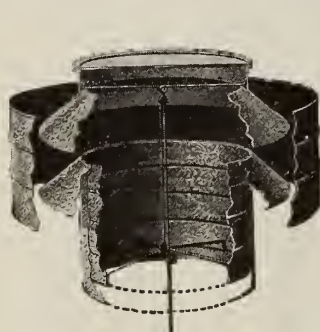
FIG. 1A. "BURT" GLASS-TOP VENTILATOR Sectional view
