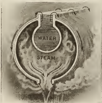
SECTION THROUGH NATIONAL DIRECT CONTACT FEED WATER HEATER
