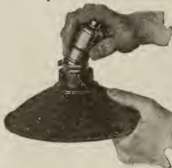
D REFLECTOR ON SOCKET To hang a D reflector on a socket, loosen screw, snap socket in ring, and tighten screw
