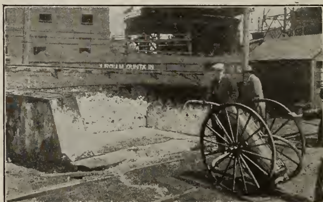
FIRE SHOWN OPPOSITE COMPLETELY EXTINGUISHED Firefoam coats the burning walls and floats on the burning inflammables in the bottom of the pit, completely extinguishing the fire and making refashing impossible
