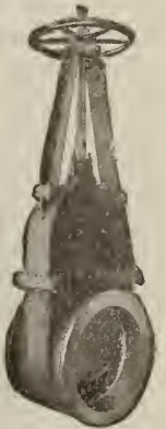
Fig. 48 "LOW PRESSURE" GATE VALVE Outside rising stem and yoke. 30 lbs. test pressure. Iron, bronze mounted, all-iron
