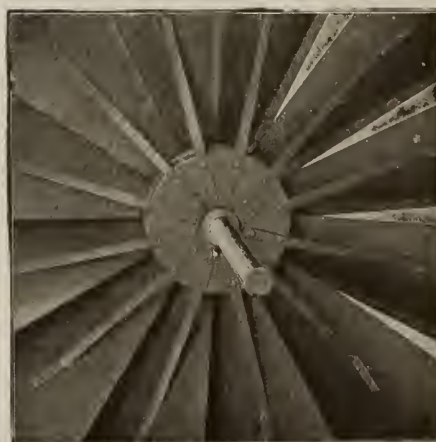
BUCKEYE DISC FAN BLADES Showing rigid bracing
