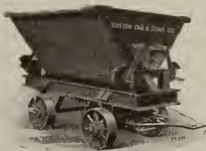
FIG. 3530. ROCKER DUMP TRAILER With extra wide tired wheels for uneven, soft ground; used in connection with tractors
