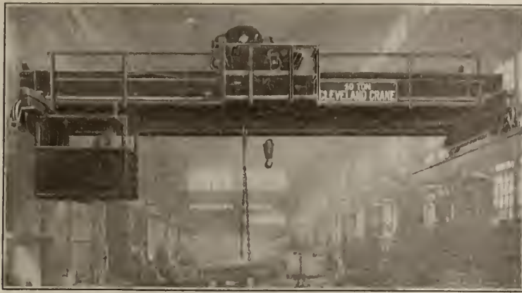
10-TON FOUNDRY CRANE 34-foot span
