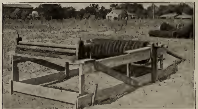
MACHINE FOR FLATTENING CONCRETE REINFORCEMENT IN ROLLS, HAND OPERATED
