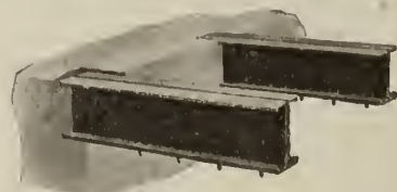
STEEL JOIST SUPPORTED BY MASONRY WALL
