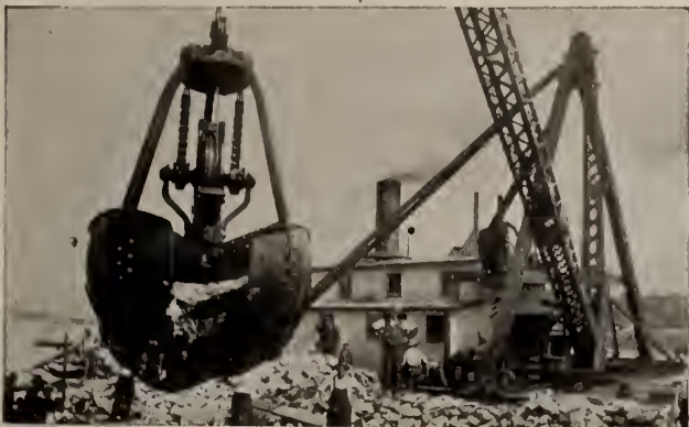
No. A-2358. HAYWARD 3-SIDED ORANGE PEEL BUCKET WITH CUT-OFF BLADES Handling a boulder larger than itself
