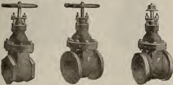
Iron Body, Screwed Wedge Gate, Flanged Brass Mounted, Hub End STANDARD STRAIGHTWAY WEDGE GATE VALVES For 125 lbs. working pressure. Tested to 150 lbs. hydraulic pressure per sq. in. with valve closed Also furnished in cast steel or bronze at special prices
