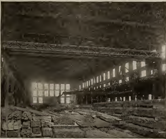
LANE ELECTRIC CRANE FOR LONG SPANS, BRIDGE OF STEEL GIRDER, LATTICE BOX TYPE
