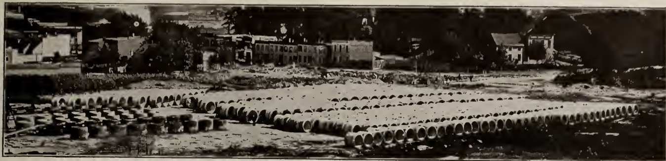
54-INCH AND 66-INCH PIPE MANUFACTURED FOR INTERCEPTING SEWER, ALBANY, N. Y.
