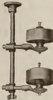
ADJUSTABLE MULE STAND Adjustable in every direction. Complete as illustrated with ceiling plate, guy rods, turnbuckles and compression grease cups. Crowned iron pulleys furnished unless otherwise specified. Stationary mule stands also furnished
