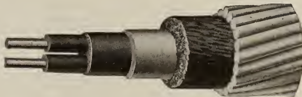
2-CONDUCTOR TWIN SUBMARINE CABLE, LEAD INCASED, JUTE SEWED AND ARMORED
