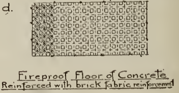
DETAIL OF FIREPROOF FLOOR CONSTRUCTION
