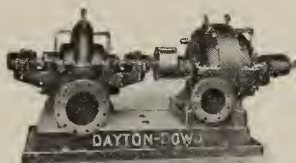
DAYTON-DOWD 10-IN. TYPE "CS" SINGLE-STAGE TURBINE DRIVEN PUMP
