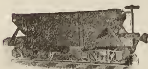
FIG. 226. HOPPER BOTTOM CAR Large double truck, with brake and automatic coupler for locomotive traction
