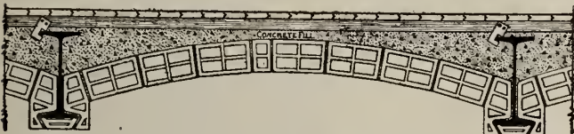
FIG. 5. TYPICAL SPAN OF NATCO SEGMENTAL ARCH
