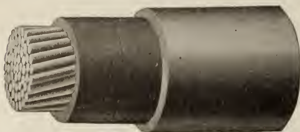
AMERICORE LEAD INCASED CABLE Stranded tinned copper conductor, rubber insulated, taped and lead incased
