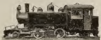
31-TON CLASS I-S 2-4-2 DOUBLE ENDER SIDE TANK LOCOMOTIVE
