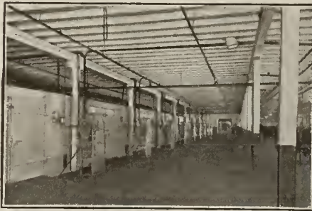
BATTERY OF 15 ELECTRICALLY HEATED OVENS
