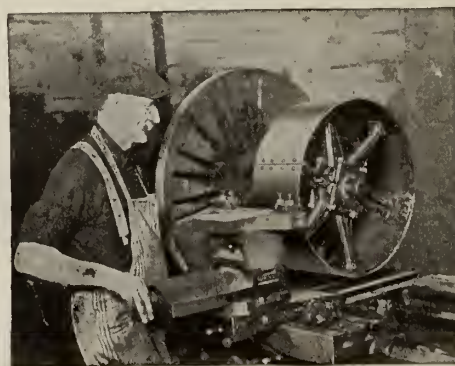
FACING THE EDGES OF A KEYSTONE PULLEY RIM
