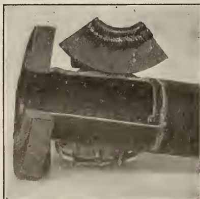
WELDED BOILER TUBE SHOWING PERFECT FUSION OF METAL
