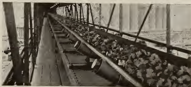
ROBINS BELT CONVEYOR HANDLING COKE
