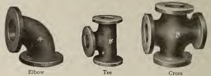
CAST IRON STANDARD FLANGED FITTINGS For 125 lbs. working pressure. Made in all styles and sizes, straight and reducing Also furnished in cast steel or bronze at special prices
