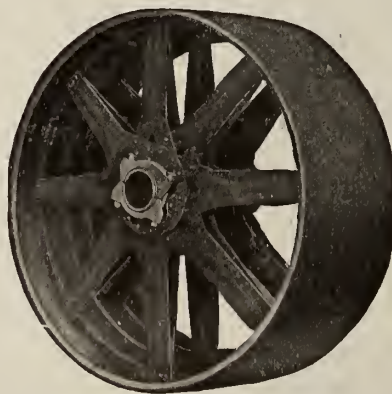
DOUBLE AND TRIPLE-ARM PULLEY 12- to 120-in. diameter, inclusive, when width of face is too great for safety with single arms
