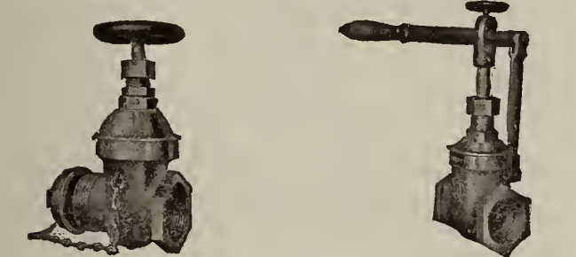
Fig. 31. "STANDARD" BRONZE HOSE GATE VALVES For working water pressures up to 150 lbs. Solid wedge disk and stationary stem. Unless otherwise specified, without cap and chain Fig. 36. "STANDARD" QUICK OPERATING LEVER VALVE Disk can be securely locked in any position by wheel screw. For working pressure of 150 lbs. water and 125 lbs. steam. Sizes, ½, ¾, 1, 1¼, 1½, 2, 2½ and 3 ins.
