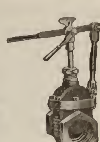
FIG. 11. Showing Sliding Stem and Lever
