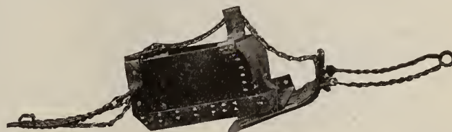
OPERATION —Operated by double drum friction hoist. Front drum operates load cable; rear drum operates “pull back” cable. The load cable generally leads from front drum through a guide block to bridle chains on front of scraper. The “pull back” cable leads from rear drum through guide block to elevated guide block at the far end of the excavation directly back of scraper, and thence to bridle chains on runner frame of scraper.
