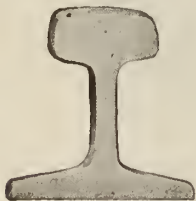
LIGHT STEEL RAILS A.S.C.E. sections, 8, 12, 16, 20, 25, 30, 35, 40, 45, 50 and 60 lbs.
