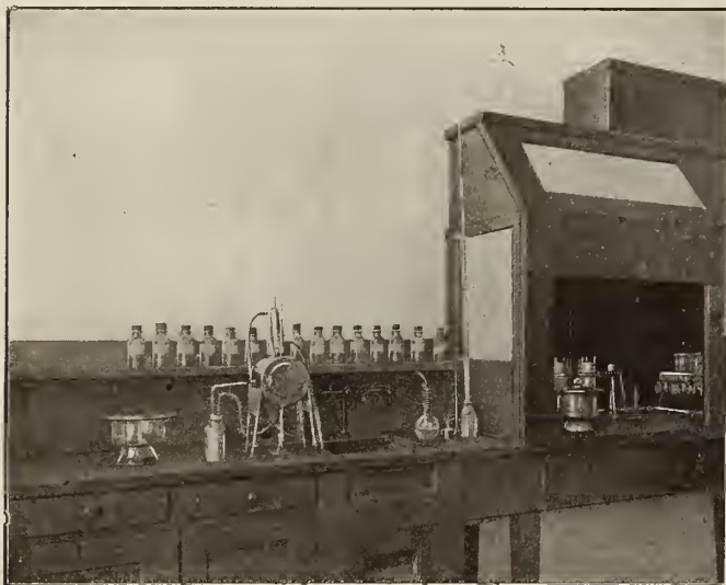
FUME HOOD, TABLE TOP, BACK, REAGENT SHELF, AND SINK OF ALBERENE STONE
