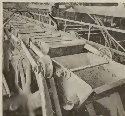
PECK OVERLAPPING PIVOTED BUCKET CARRIER For handling coal and ashes, stone, gravel, etc.
