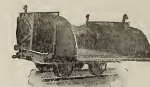
FIG. 414. DOUBLE SIDE DOOR COAL CHARGING CAR
