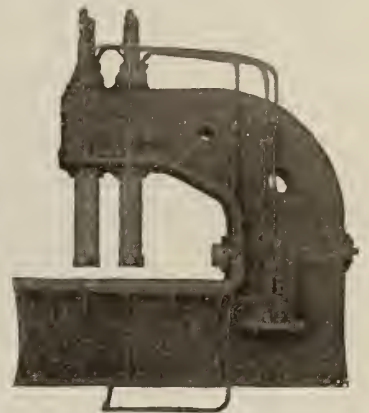
200-TON SECTIONAL FLANGING PRESS
