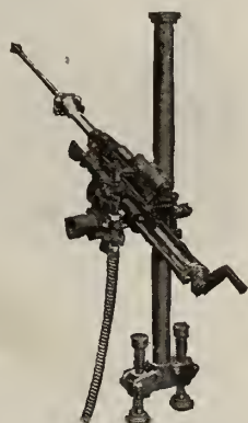
C-22 IMPROVED TYPE "GATLING" DRILL With patented cushion device, mounted on column Most powerful "one-man" drill on the market
