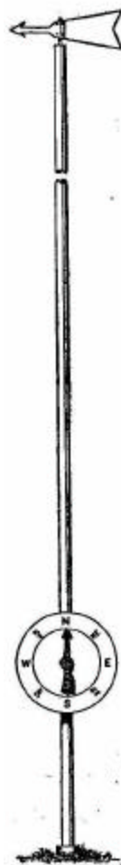
FIG. 165.—Wind vane with dial.
