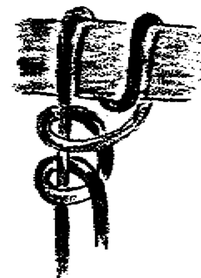
k Round Turn—Two Half Hitches. Mooring knot.
