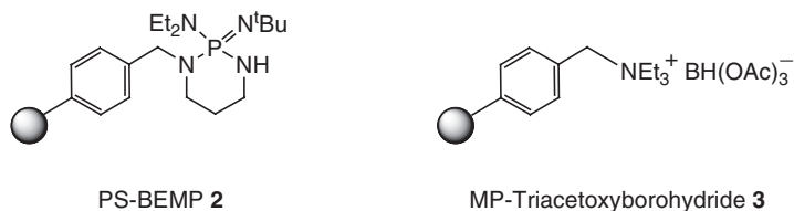
Figure 2 Some examples of commercial polymer-supported reagents
