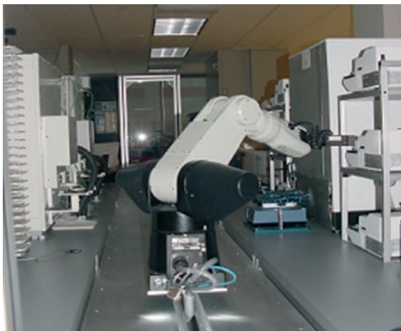
Figure 5 The lead evaluation robot above is loading a 384-well microtitre plate into a liquid-handling device. The robot move up and down a track, move plates between reagent addition stations, incubators and readers
