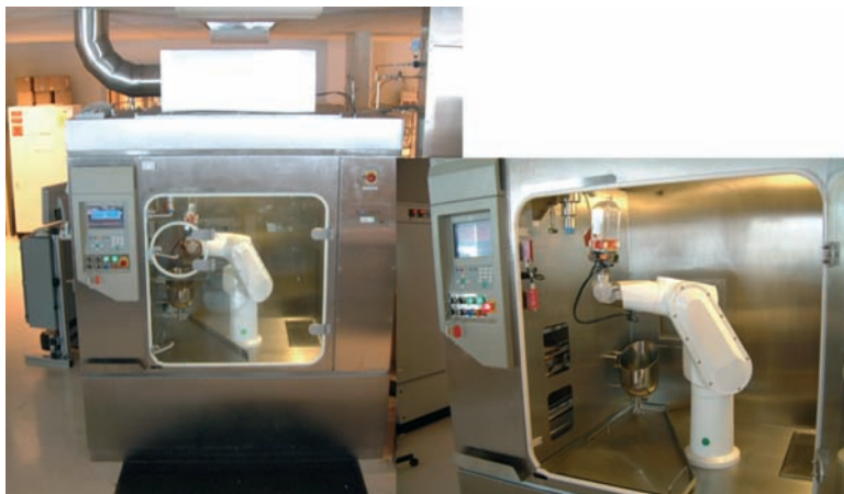
Figure 3 Photograph of the Cellmate™ robot built by The Technology Partnership, Cambridge, UK. This robot performs cell seeding in either large T flasks or roller bottles, exchanges media, rinses cell sheets, purges gases, harvests cells by trypsinization or scraping, and supports transfections
