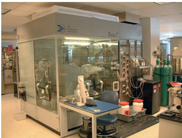
Figure 4 A photograph of the SelecT™ robot built by The Technology Partnership, Cambridge, UK. This robot maintains between 1 and 50 cell lines, performs passaging, cell counting and viability measurements, and direct plating into microtitre plates for bioassay
