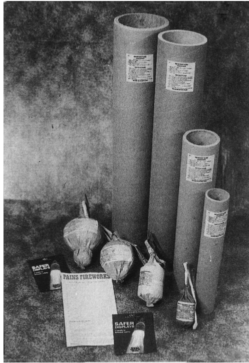
Figure 4.1 50, 75, 100 and 125 mm shells plus mortars, ca. 1990 (but no longer available to the general public). (Courtesy of Pains Fireworks Ltd.)
