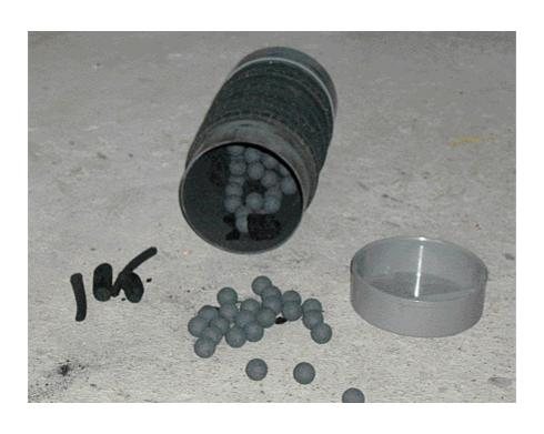
This shows the basic construction. The black horizontal bar is the rubbercovered roller, driven by the motor on the right. The two small white structures are small plastic wheels, such as are used under furniture. The container consists of a section of PVC tubing with fitting end caps. The picture shows some of the lead media (1.78 cm diameter lead balls), and a few chunks of charcoal. These will be broken up in the mill in a matter of minutes. Strips of rubber are glued around the container as
